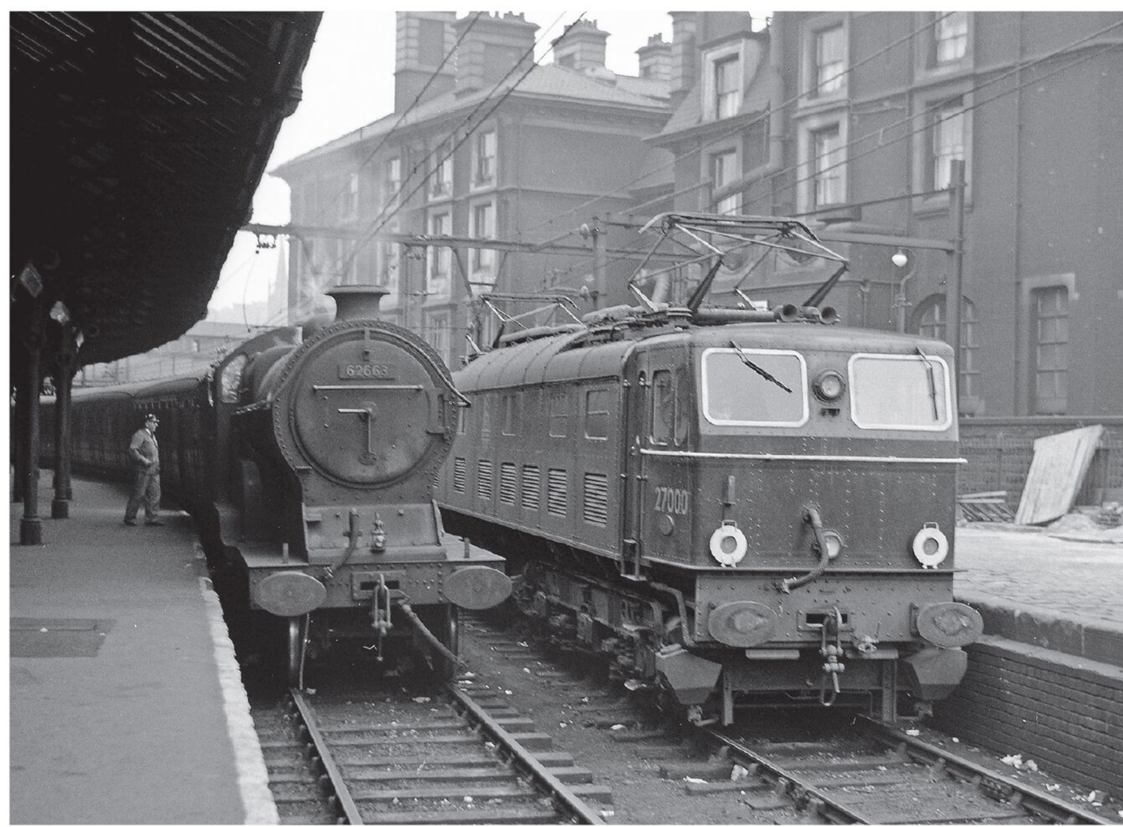
◀ Class D11 4-4-0 No. 62663 Prince Albert is pictured at Sheffield Victoria in this 1958 view, whilst alongside is now-preserved EM2 Woodhead electric locomotive No. 27000. Photo: Rail Photoprints
