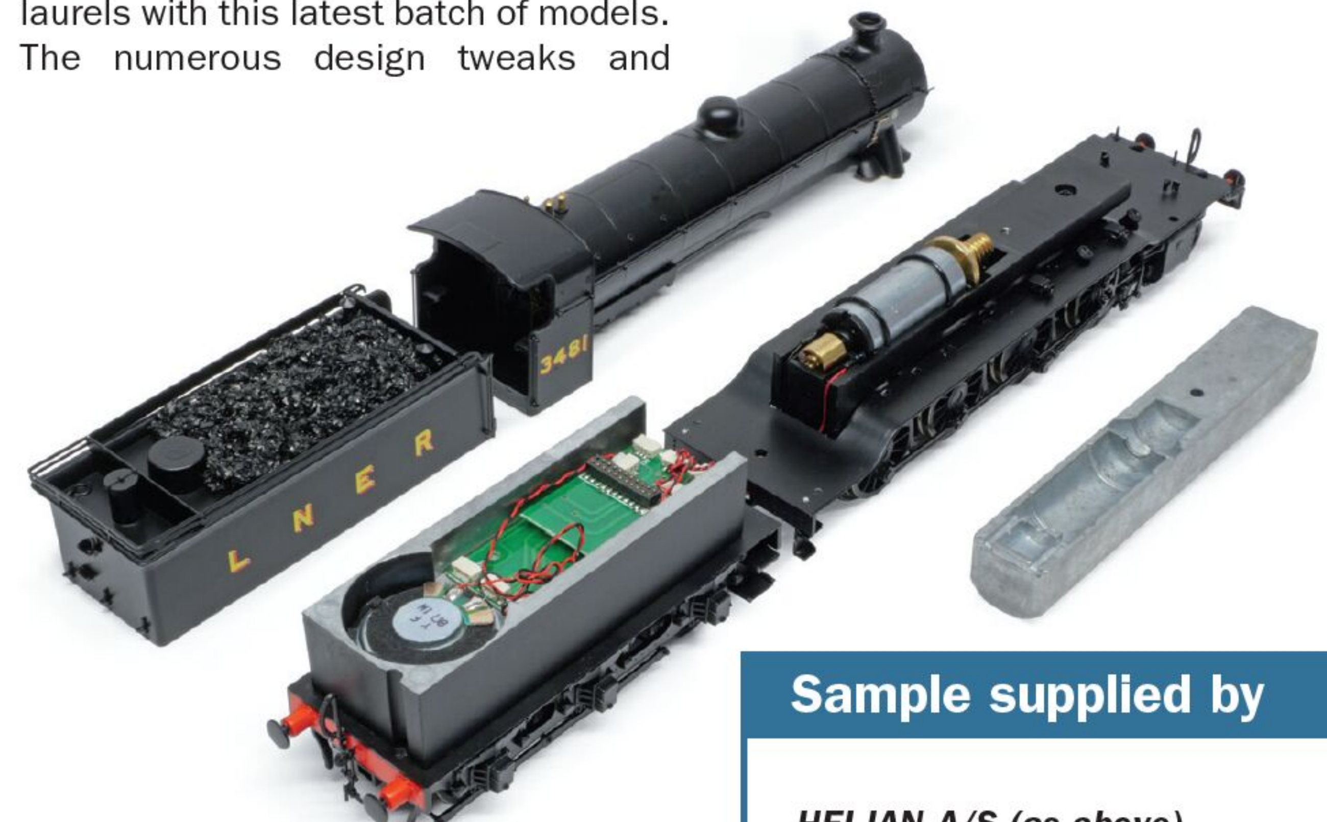
▲ The tender now features a pre-fitted sound speaker.
