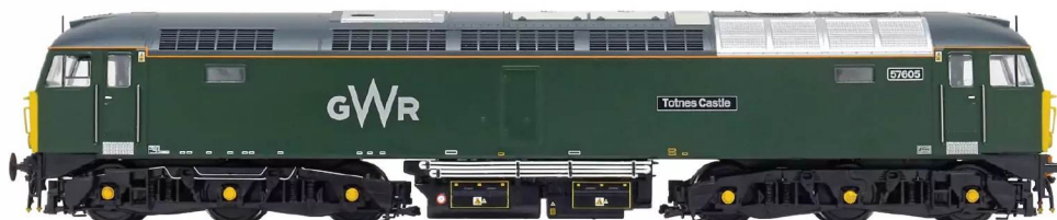
▲ The Class 57 chassis has a 21-pin decoder interface, but no sound provision.
