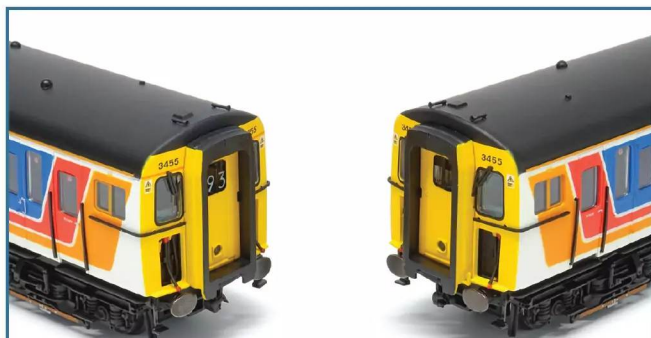
▲ The drawbar for coupling two units together is designed to resemble the prototype's buckeye couplings...
