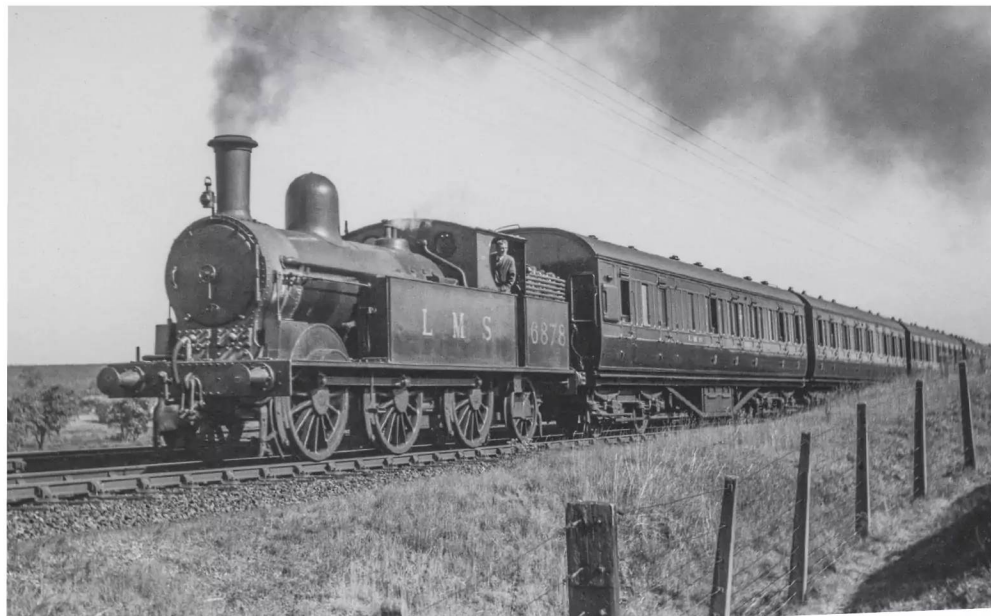
▲ The LNWR '1560' Class/18" Tank numbered 80 in total with construction taking place at Crewe between 1898 and 1902. Essentially a tank engine version of the company's 'Cauliflower' 0-6-0s, these mixed traffic machines were often used on suburban services between Euston and Watford, hence their unofficial nickname of 'Watford Tanks'. 77 passed into LMS stock, with 15 still in service upon Nationalisation, although only two survived long enough to receive a BR number. LMS No.6878 is on a passenger service in this picture, believed to have been taken in the 1930s near Cannock. Photo: Rail-Online
