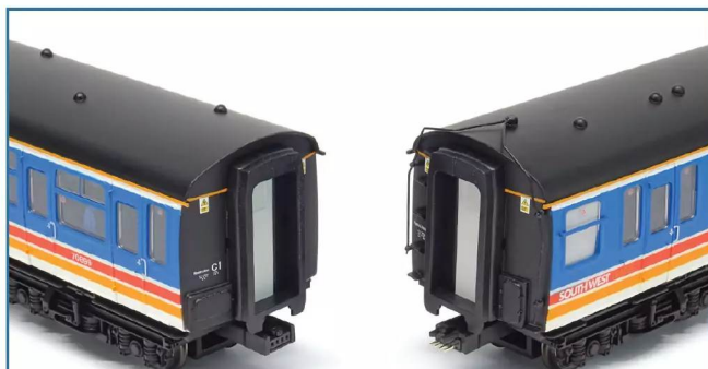
▲ ...while a new four-pin close coupling arrangement joins the four cars of the unit.
