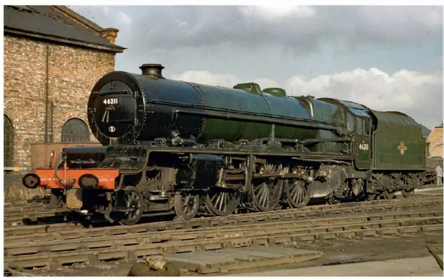
▲ No.46211 outside Crewe Works on 15 March 1959, in the condition and livery modelled, with speedometer and Automatic Warning System equipment. Photo: Colour-Rail
