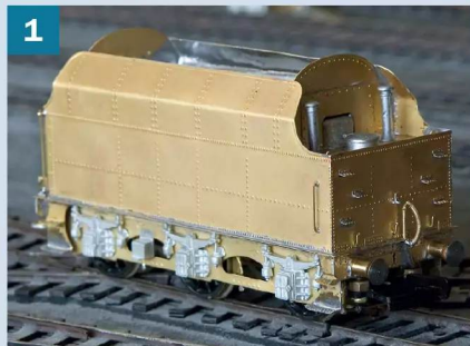
1 ▲ The assembled Comet Models tender kit for a Stanier 10-ton 4,000-gallon design (ref.TK8) prior to separation of the chassis from the body for painting. The kit comprises etched brass frets with cast brass, nickel silver and whitmetal detailing parts.
