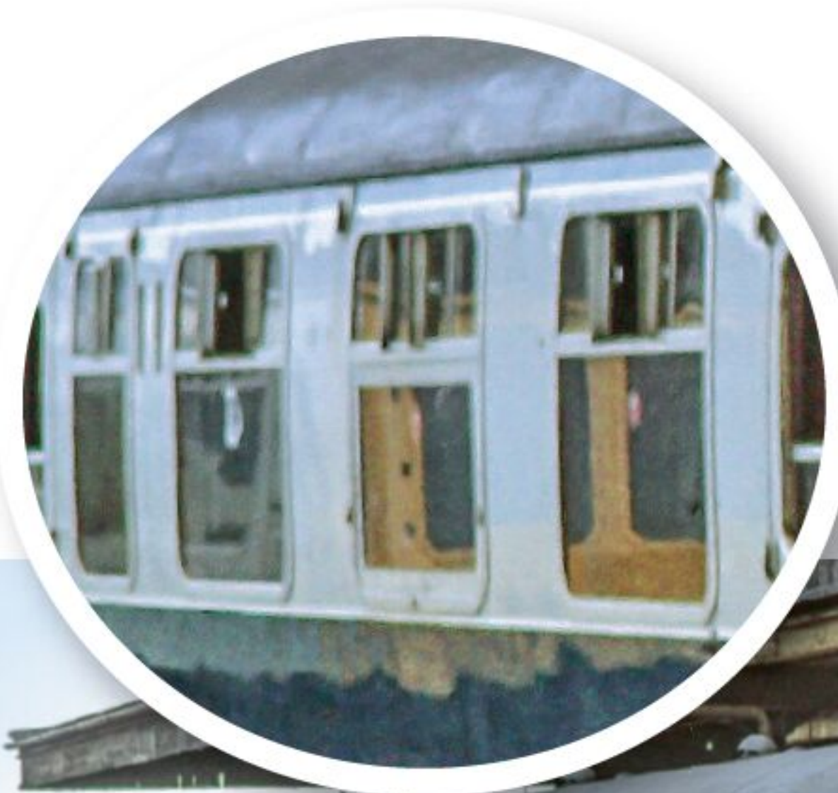
▲ The frame of the direct access window is clearly visible in this view of BR Mk.I CK E15957, recorded at York on 27 August 1978. Photo: Transport Treasury
