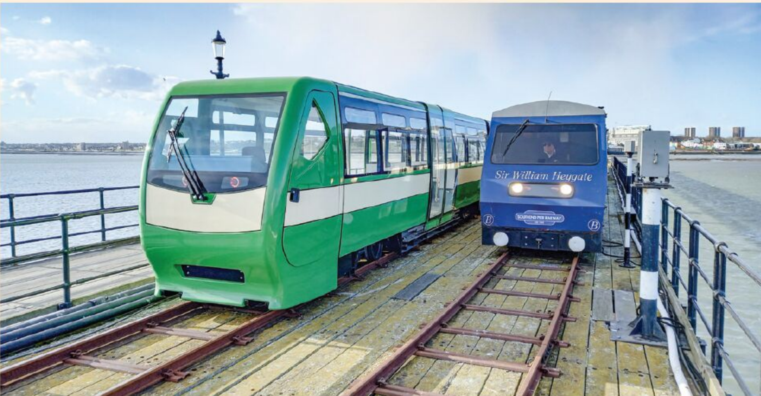
▲ A second March 2022 view, showing one of the new battery-electric trains (left) passing one of the c.1986 trains (right). All photographs by Kevin Weston. (All were taken while on duty and either with no trains running or with appropriate lookout protection.)
