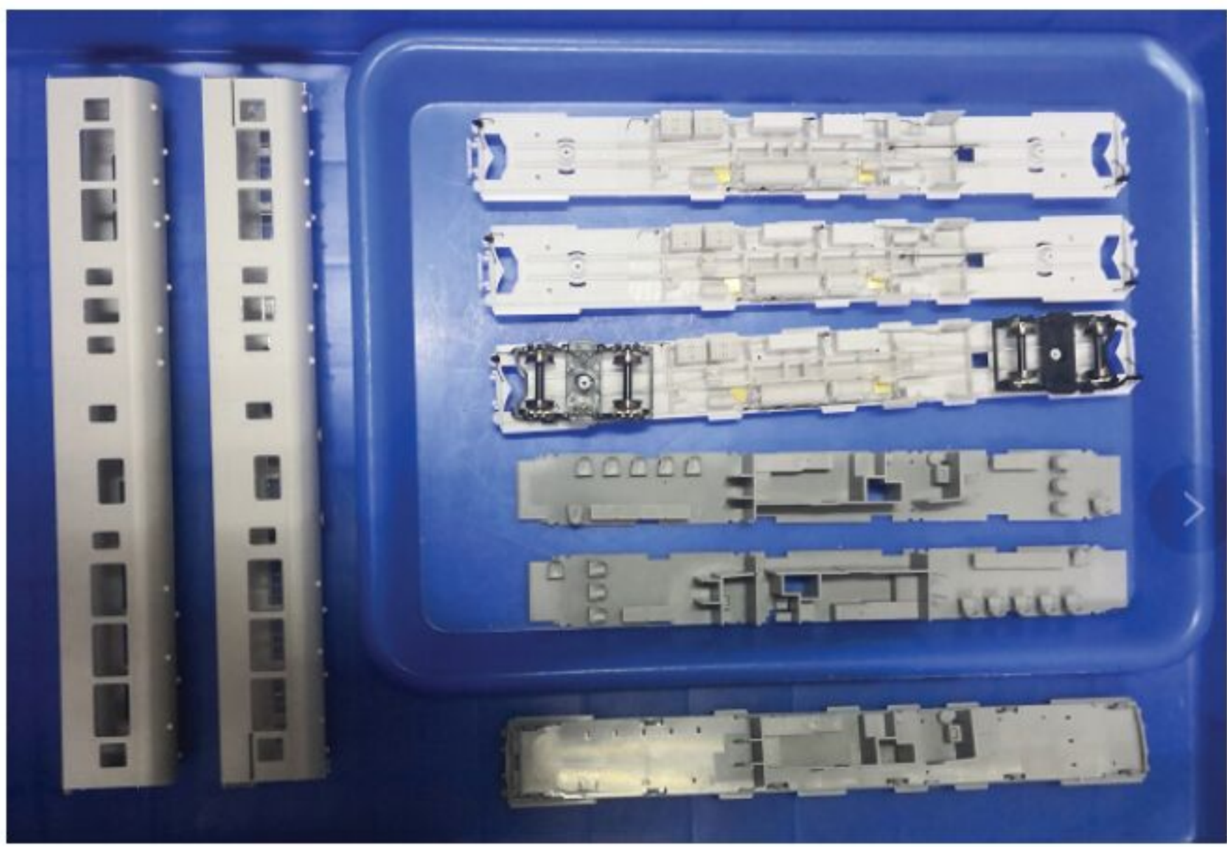
▲ Examples of some of the 'first shots' produced from the mould tools.
