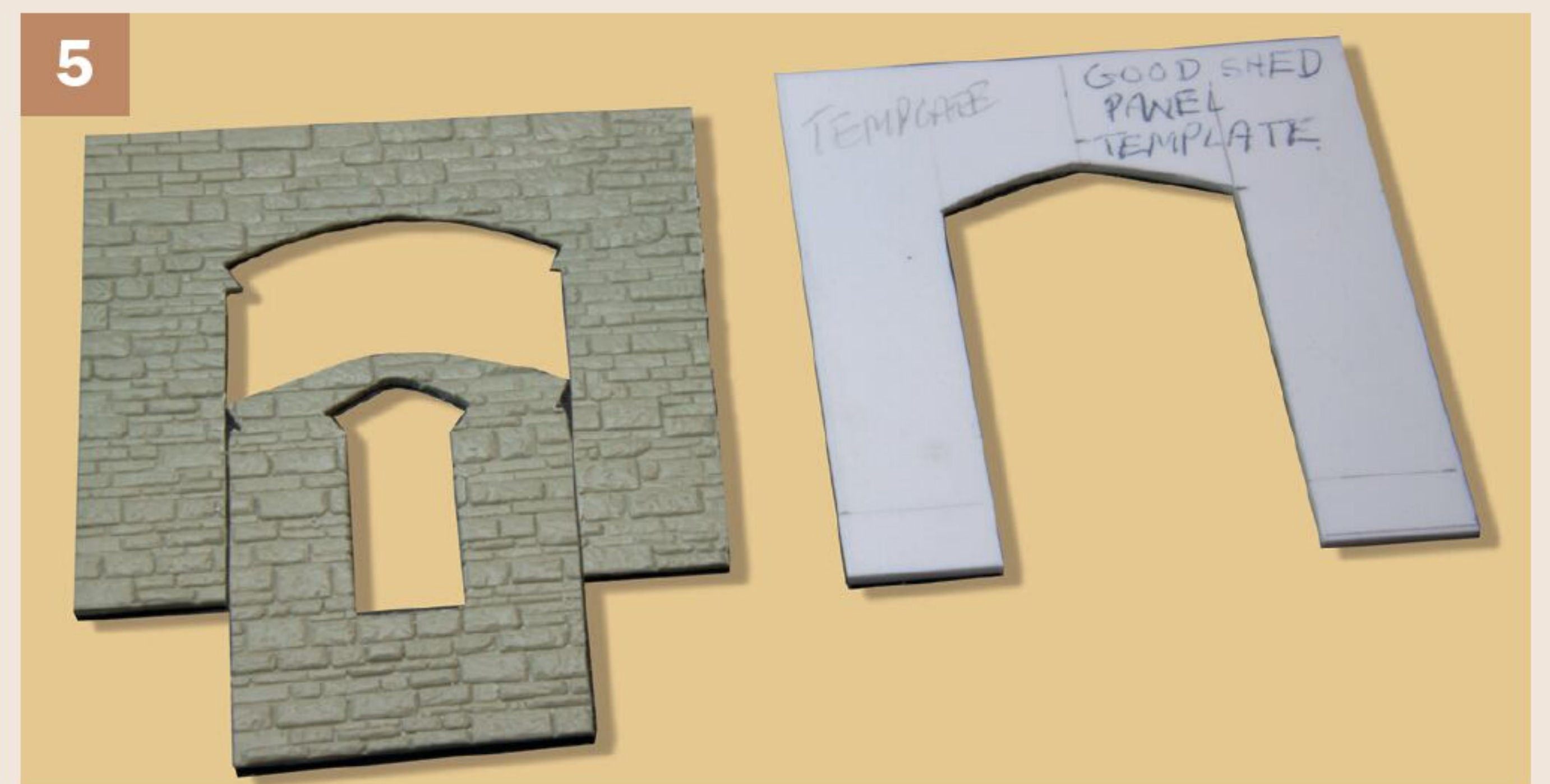
▲ To maintain consistency I made templates for the basic door and recessed panel openings (they are all the same size) and also for the windows and stone arches, a combination of razor and piercing saw work.
