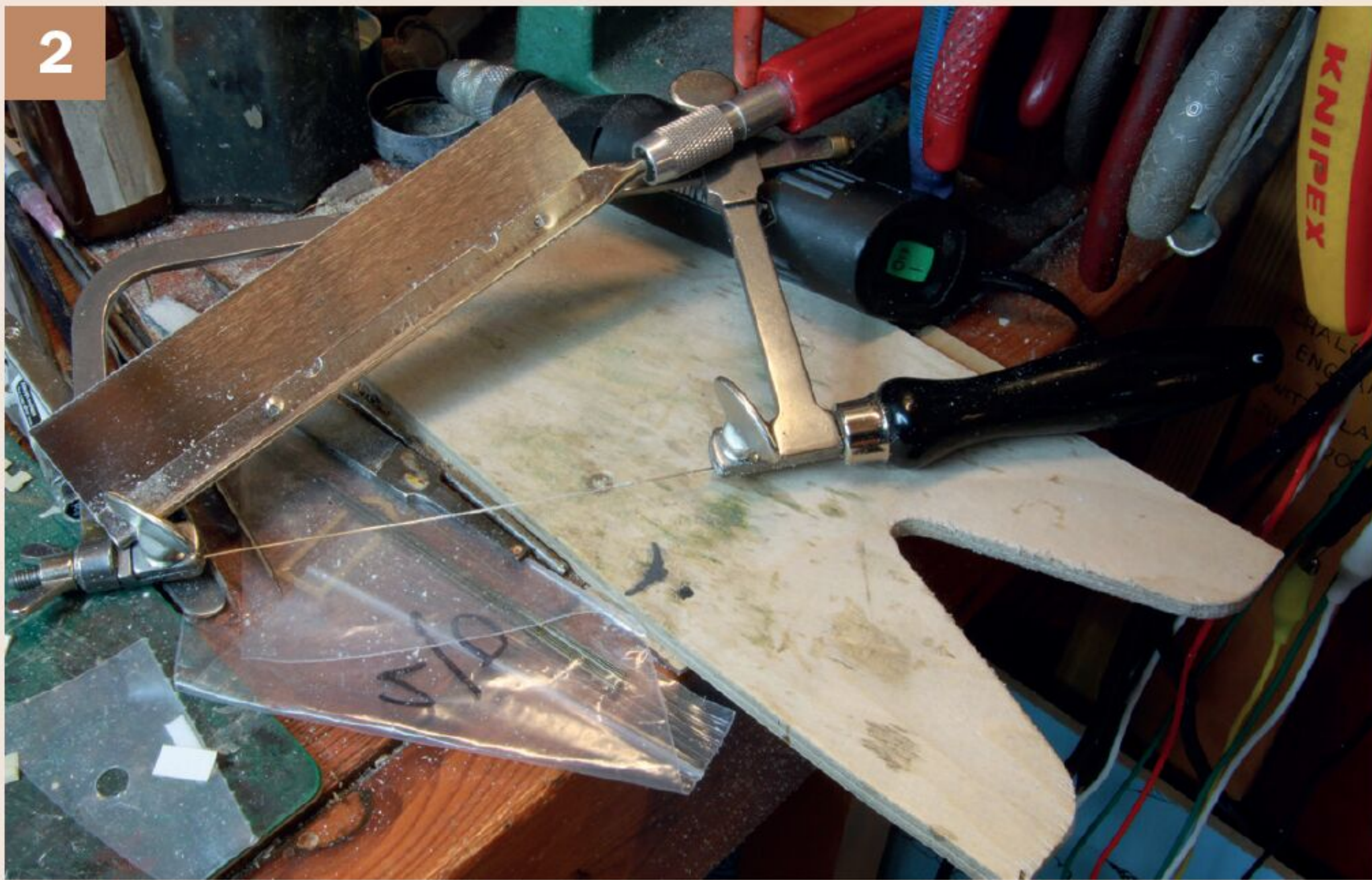
▲ Tools of the trade. For thicknesses of plasticard of 60thou and upwards a razor saw, such as this X-Acto one, or a jeweller's piercing saw can be preferable to a Stanley knife for cutting the sheets, although the last has myriad other uses.
