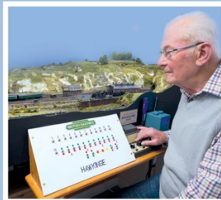
▲ The author at the controls, which takes the form of a Gaugemaster twin-track unit. Point and section switches are provided on the panel.
