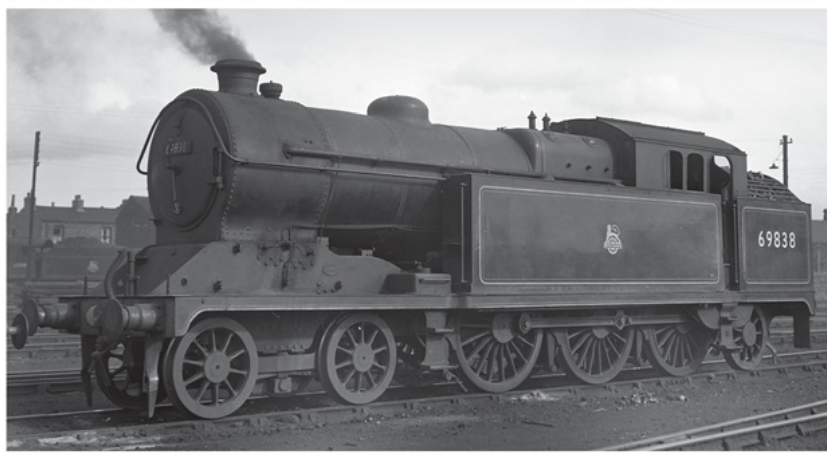
▲ Class A5/2 No.69838, pictured at Darlington on 4 August 1953, displays the different shape of the front framing under the boiler – to make the inside motion more accessible – and a riveted smokebox. Photo: Transport Treasury
