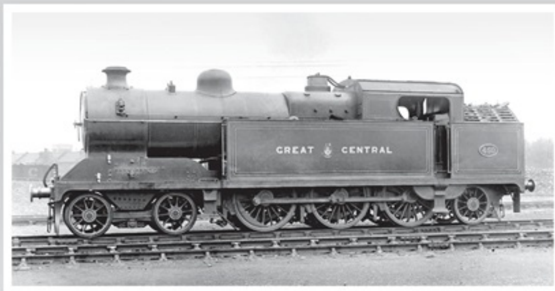
▲ GCR Class 9N 4-6-2T No.450, in original condition before the cab was modified with side windows. Note also the boiler top feed in front of the dome and the superheater discharge valve on the side of the smokebox. Photo: Mike Morant collection
