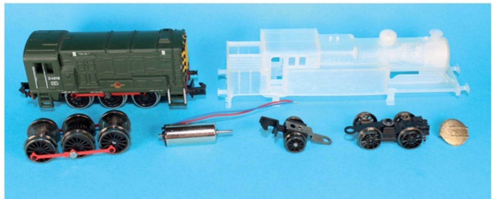
▲ The component parts for the project: clockwise from top left, a Farish Class 08, Recreation21 3D printed Class A5 body, smokebox door from N Brass Locos, Graham Farish/Bachmann Class A1 bogie and '6100' trailing truck, Tramfabriek five-pole coreless motor, and replacement blackened wheels for the 08 chassis.
