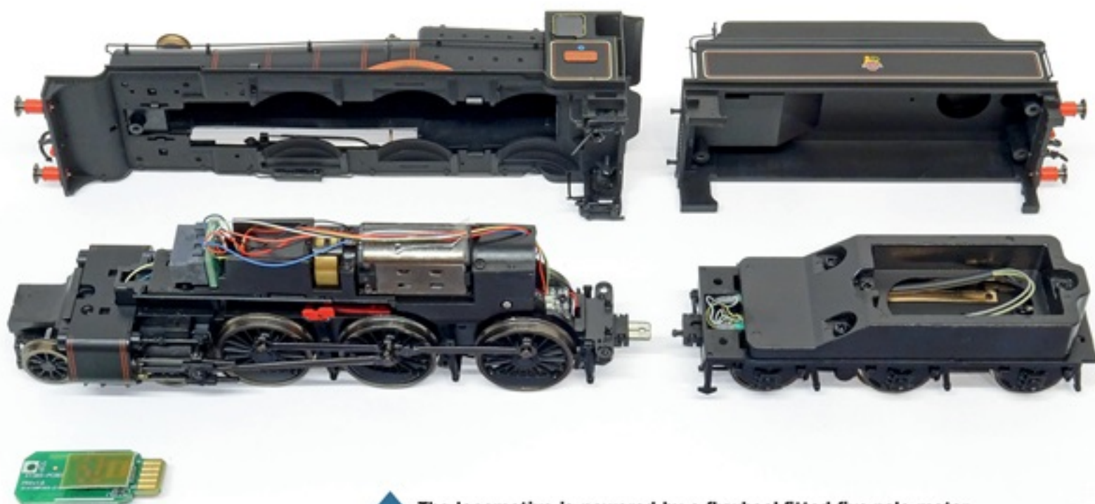
▲ The locomotive is powered by a flywheel-fitted five-pole motor.
