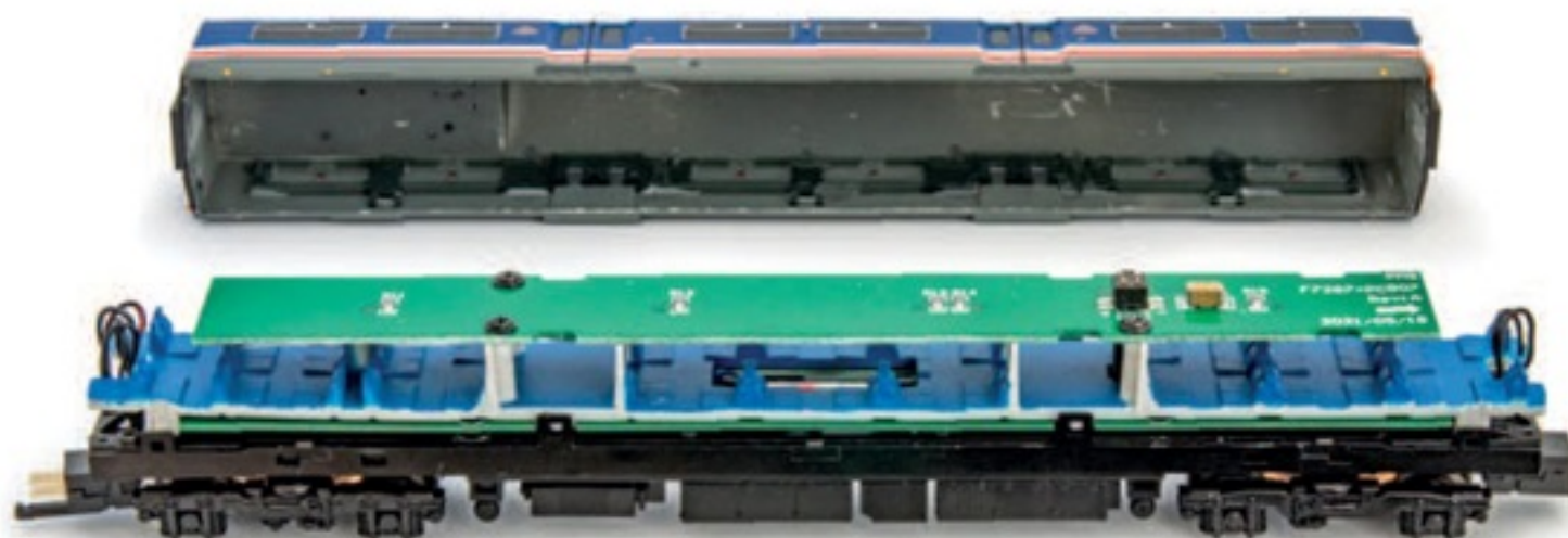
▲ The MSO houses a central motor that drives both bogies. The upper PCB provides interior lighting.
