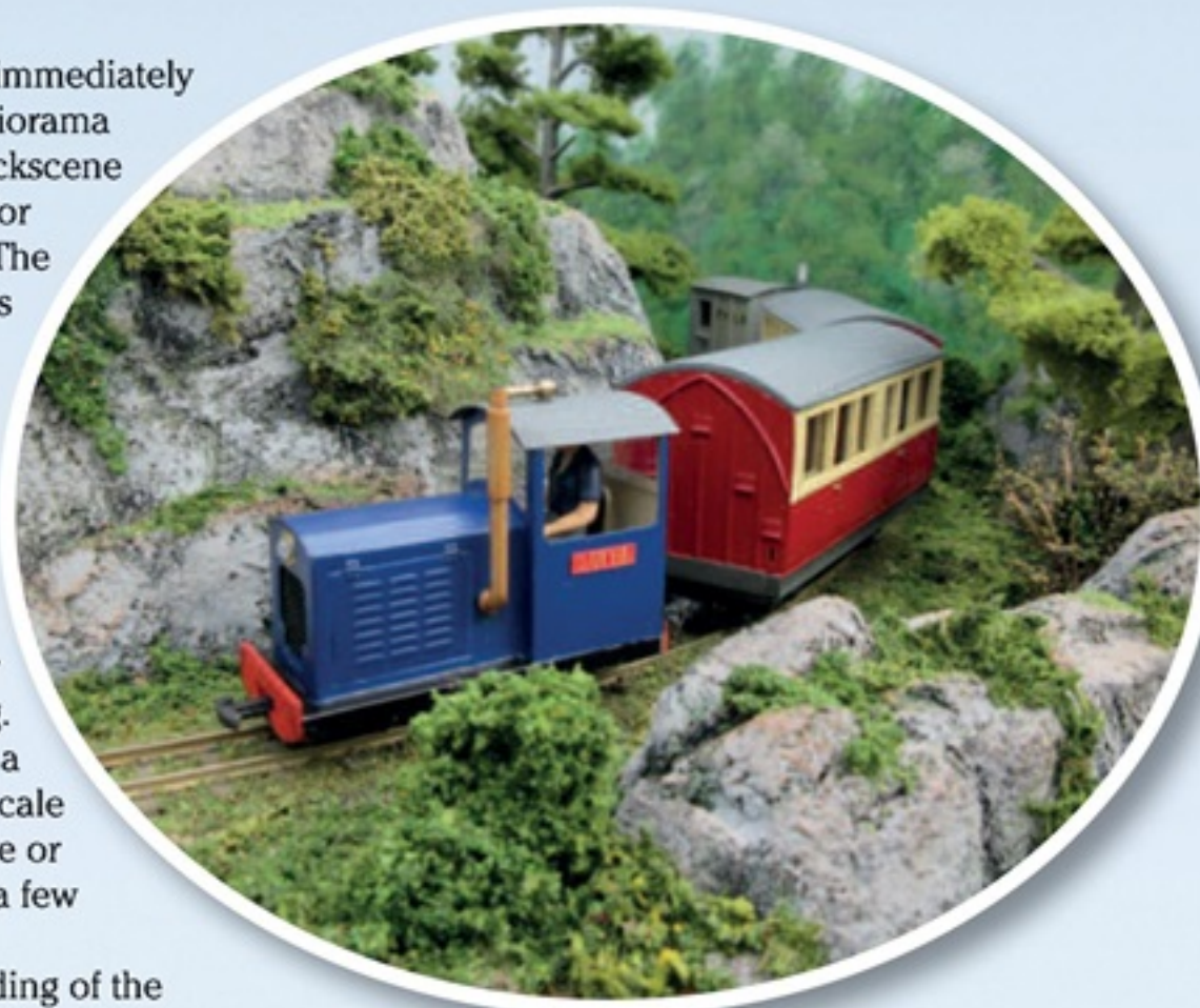
▲ Satyr hauls the first two 7mm coaches that the author made, which are modified Hornby OO gauge four-wheelers on Peco OO9 bogies.
