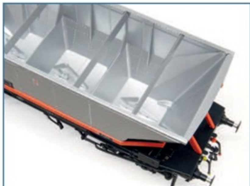
▲ The hopper bodies include internal strengthening bars.
