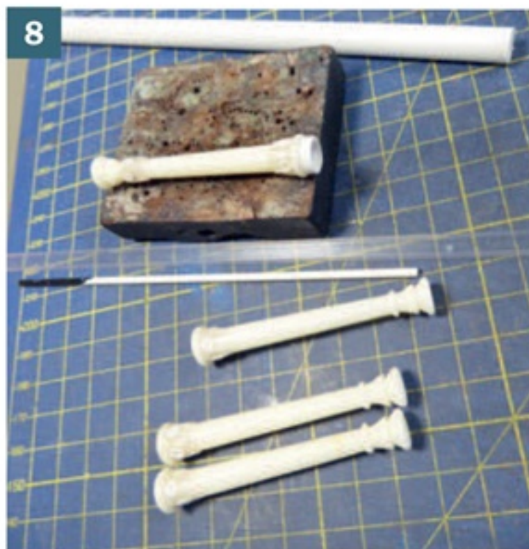
▲ I was doubtful that I could produce eight completely identical columns, so I enlisted the help of York Modelmaking to produce eight 3D printed 65mm long columns with the feather details on the top.
