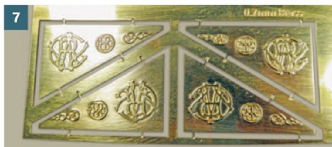
▲ The finished etches of the decorative scrollwork were produced in 0.7mm thick brass.
