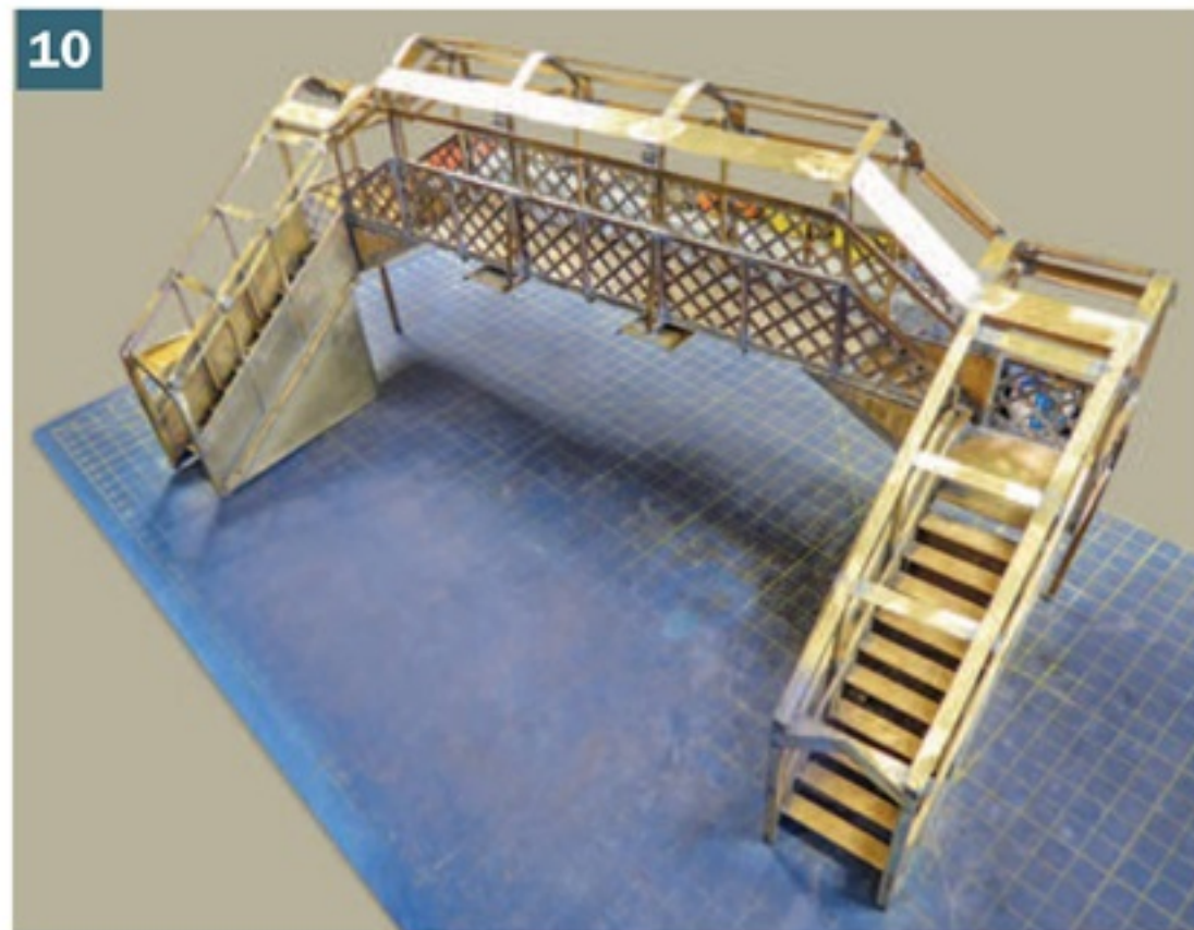
▲ Additional brass strip from old waste fret was soldered in place to provide the skeleton for the plasticard roof.
