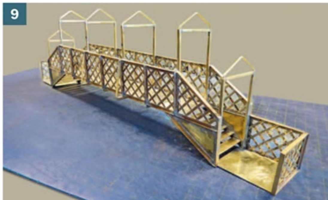
▲ The roof consisted of a temporarily removable brass framework built from 2mm square section and 1.5mm rod.
