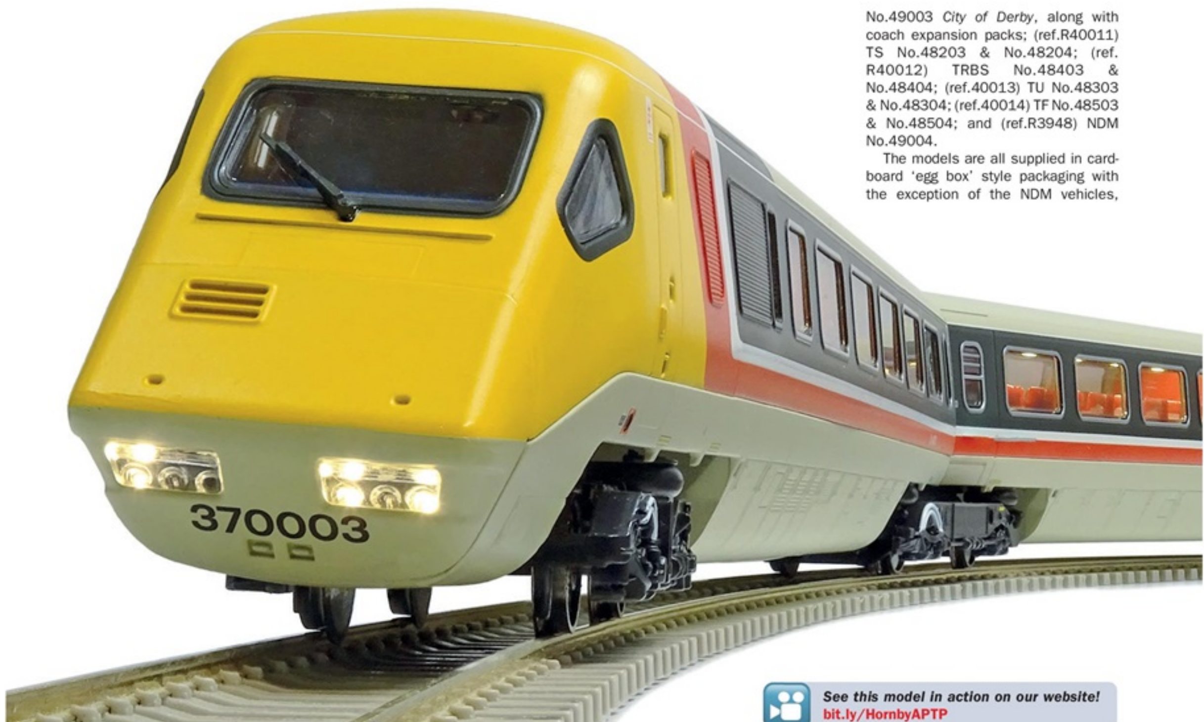
▲ A ball and socket on the articulated bogies allows the body to tilt.
