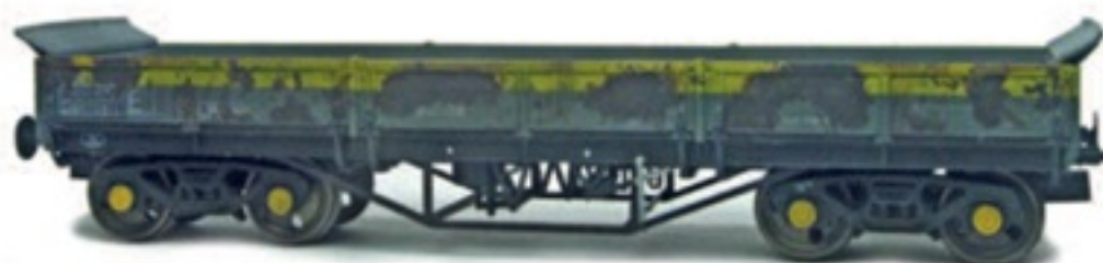
The colours inside and outside the wagon have been toned down with Humbrol black using an airbrush. Using paint washes would also achieve the same effect.
