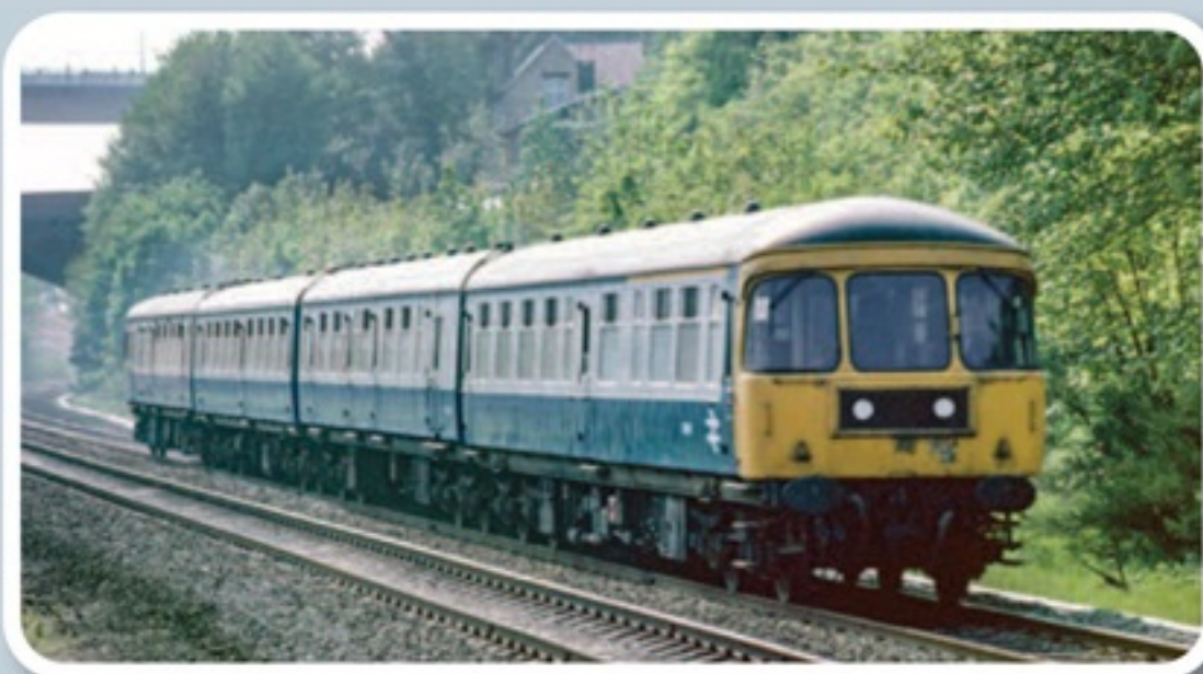
▲ This eastbound service seen approaching Hesse station in May 1982 illustrates one of the four-car 'hybrid' sets with a 124 Driving Motor Composite leading and 123 Driving Motor Brake Second at the rear. The second vehicle is a de-engined 124 Non-driving Motor Brake Second.
