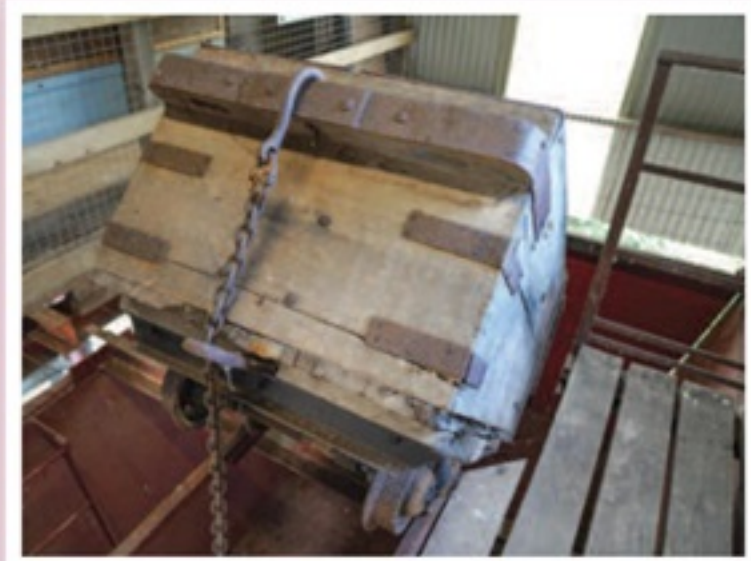
▲ The clay was then end-tipped into the narrow gauge side-tipping wagons marshalled below the hopper for onward transshipment to Furzebrook.
