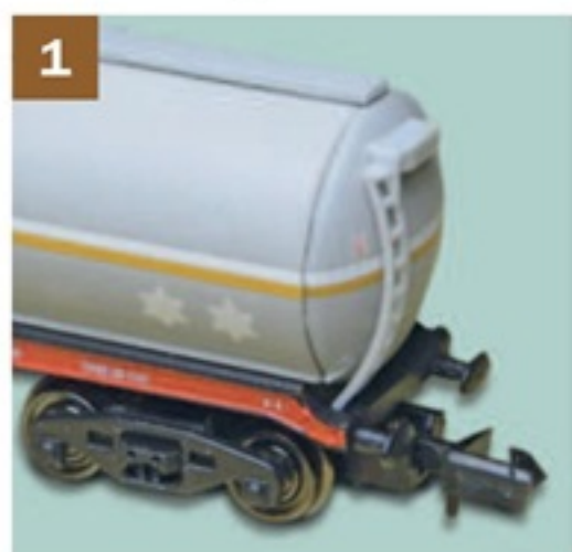
A close up of the Farish TEA bogie tanker which shows the incorrect pattern bogies and rather chunky plastic ladder, although the livery finish and solebar lettering is to a good overall standard.
