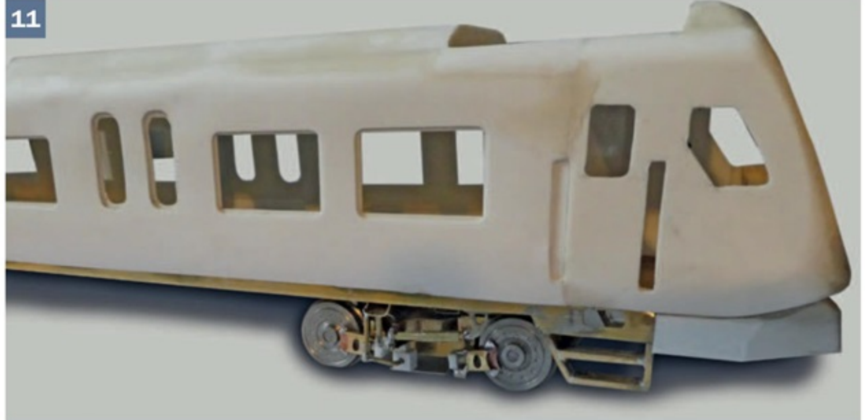
This view shows trial fitting of the bogie to check ride height. Also illustrated is the window construction with a 1mm wide ledge formed by cementing plasticard strips around the insides of the window apertures. The resultant recesses were painted black before inserting the glazing.
