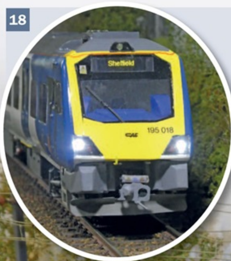
One of the completed cabs showing the distinctive shapes of the anti-climbers below the headlights, the obstruction deflector and the coupling assembly.
