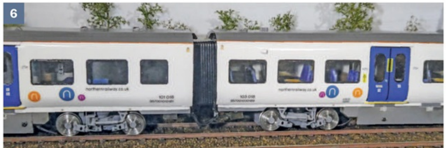
6 The jumper cables, which are just visible here, were made from thin black elastic material and strung between the two cars underneath the gangway. The gangway was built as a separate pivoting section and allows the pair of units to traverse sections of curved track with ease.
