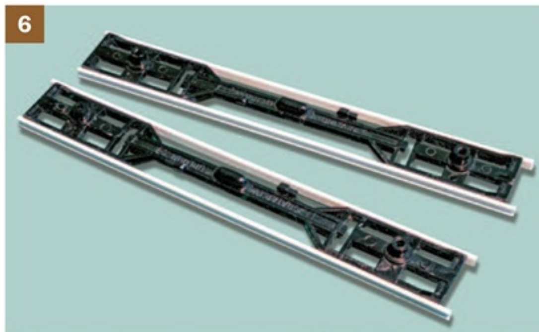
6 Evergreen U-channel was used to fabricate new solebars, which here have been fixed in place using cyanoacrylate adhesive.
