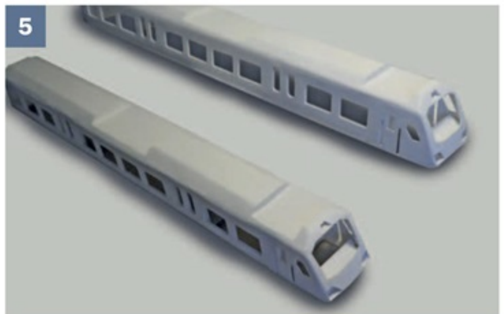
5 The two body shells were sprayed with Halfords white primer. Doing this showed up any areas where sanding or filling of the surface was necessary.
