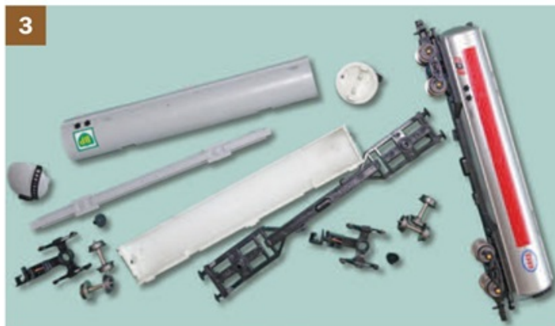
A pair of Graham Farish TEA tanker wagons, one of which has been dismantled into its component parts.
