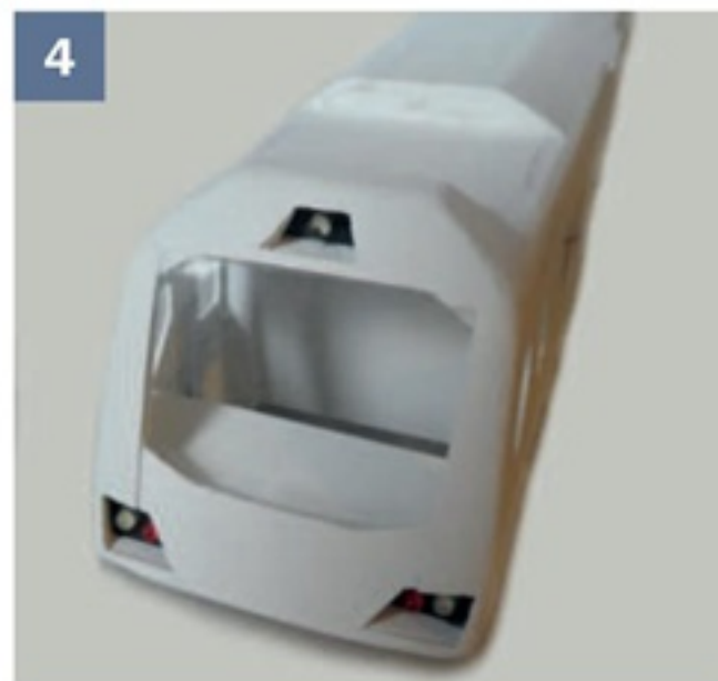
4 Black plastic was used as backing for the LEDs. These were recessed from the front and glazed after painting.
