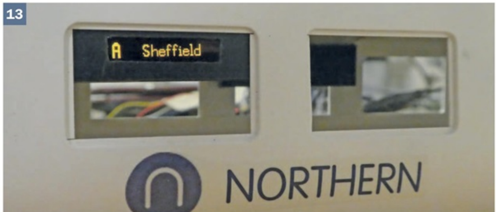
Trial fitting of one of the programmable side destination displays. These utilise OLED (Organic Light Emitting Diode) displays built into black boxes, which are obtainable from specialist electronics suppliers.
