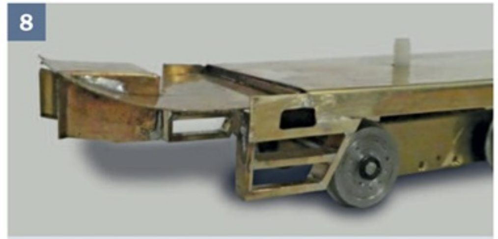
8 The upward sweep at the front was formed by using a separate sheet of brass attached to the main chassis. The box for the coupler can also be seen in this view.
