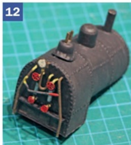
The boiler was made from a length of 35mm copper tube. Scrap materials were used to make the backhead fittings.
