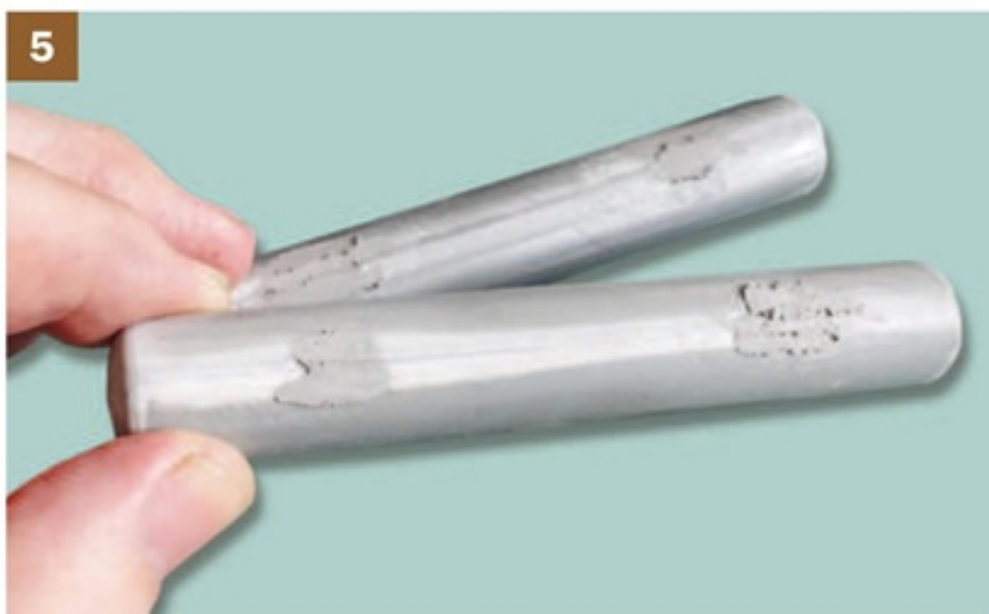
5 Any gaps and holes were filled, along with the tank filler hatch areas. Once dry the surfaces were then filed smooth.
