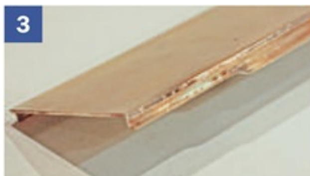
3 The forward ends of the solebars had to be split and reduced in height to accommodate the motor bogie in a reverse curve – similar to that seen on the Gresley style of locomotive footplate.
