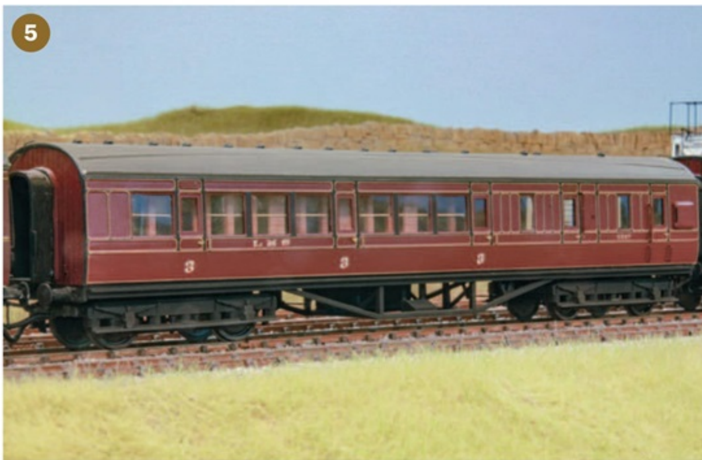
▲ LMS Period III Stanier 57' Open Third No.9012 to Dia.1904, one of the 50 constructed in Lot 805 by The Birmingham Carriage & Wagon Company in 1934. Being an etched Perseverance kit with equalised bogies this ranks as the most hi-tech of the eight coaches in this rake. It was also the most challenging... No doubt because I found myself entering new territory regarding structural technique at times, but it has turned out as a neat model not available (at the time of writing) from any of the major ready-to-run manufacturers. Precision Paints and HMRS lining, logo and number transfers complete the model.
