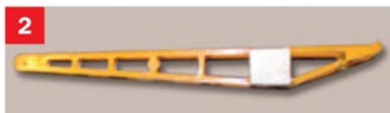
2 Modification was carried out to the jib, with the addition of an off-centre box to provide the pivot point.
