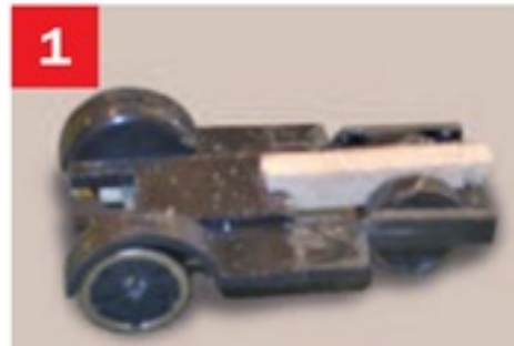
1 The modified chassis with the Teamsterz wheels. The balsa support for the rear deck was later hidden by the casing round the motor compartment.
