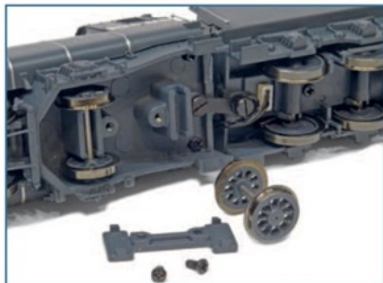
▲ Substitute flanged wheelsets are supplied for fitting in place of the flangeless versions if layout curvature allows.
