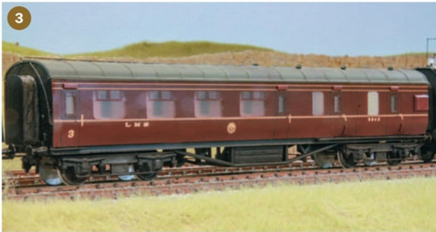
▲ Another MAJ kit, only adorned with the simple LMS lining, and this time a Corridor Brake Third, No.5943, from a batch of 44 built as Lot 911 to Dia.1905 at Wolverton in 1936. The usual extras are provided, and I must say that MAJ coaches run smoothly and freely.
