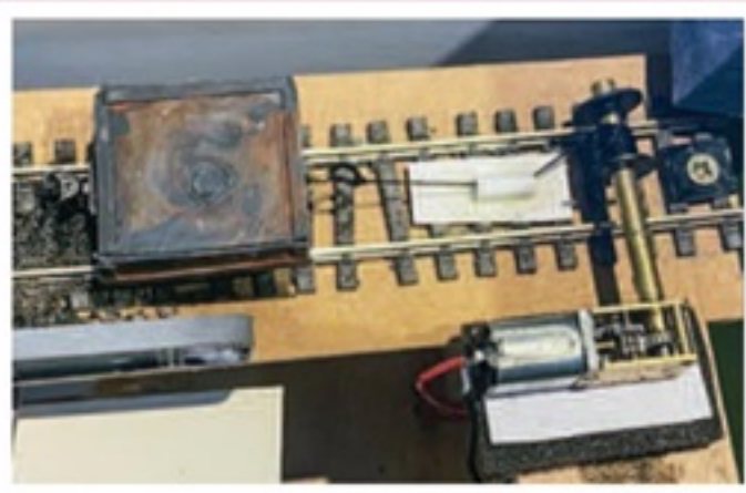
▲ The rope-worked incline is operated using this small electric motor and gearbox.
