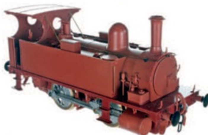
▲ Engineering sample of an Adams B4 0-4-0T in O.
