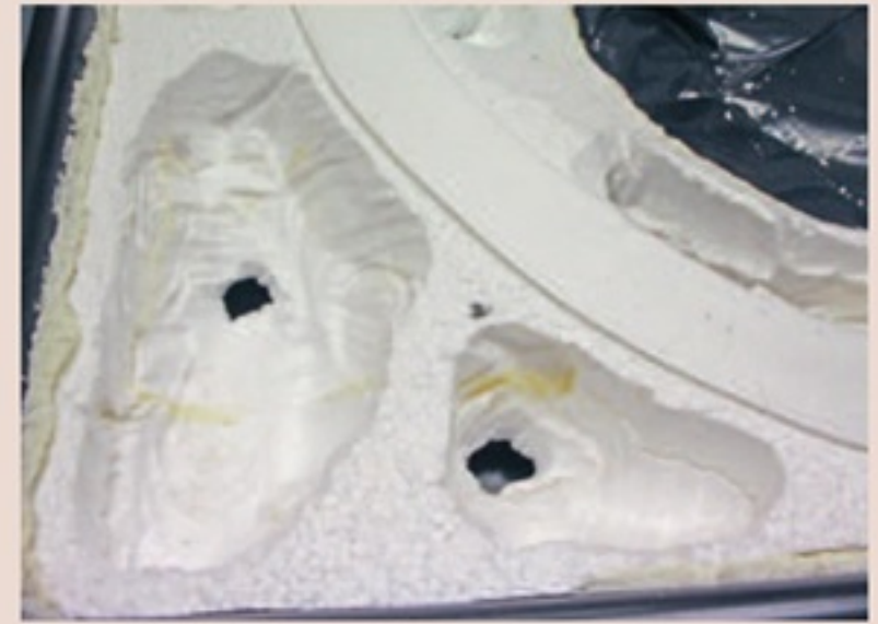
▲ Cavities were carved out of the polystyrene sheet, together with water drainage holes, to accept the plants and trees.
