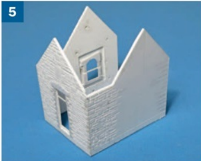
5 Each outer wall was reinforced by laminating a second layer of 40thou plasticard to the reverse, with small holes drilled to facilitate the application of the solvent. This view shows clearly how the window frames were constructed from individual parts.
