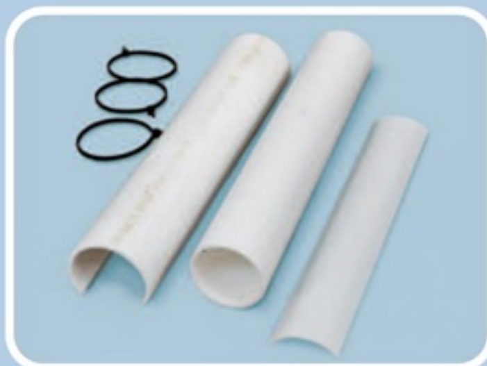
▲ The component parts of the home made 'moulding tool' from left; the slip on cable ties; the split length of pipe to act as an outer top clamp; the inner pipe former around which the plasticard is held; a curved piece of plasticard fresh out of the mould after cooling.
