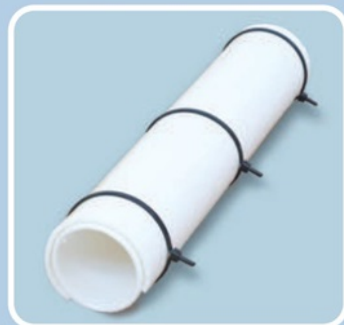
▲ The mould assembled with the plasticard inserted, all ready for the heating stage.
