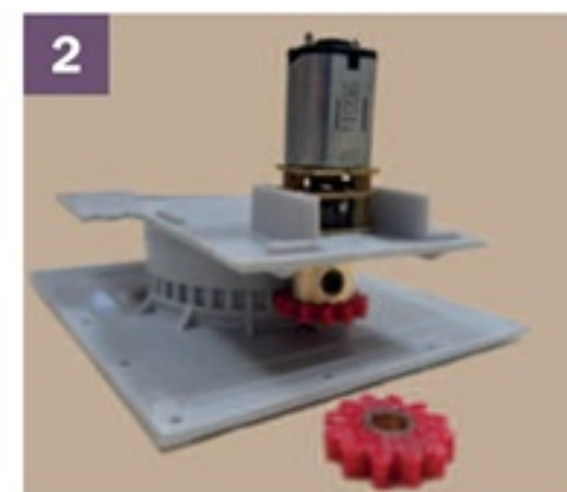
The cab rotating motor fitted with the modified Technobots pinion spur gear which was halved in thickness by cutting through with a fine razor saw – the offcut shown went in the scrap box.
