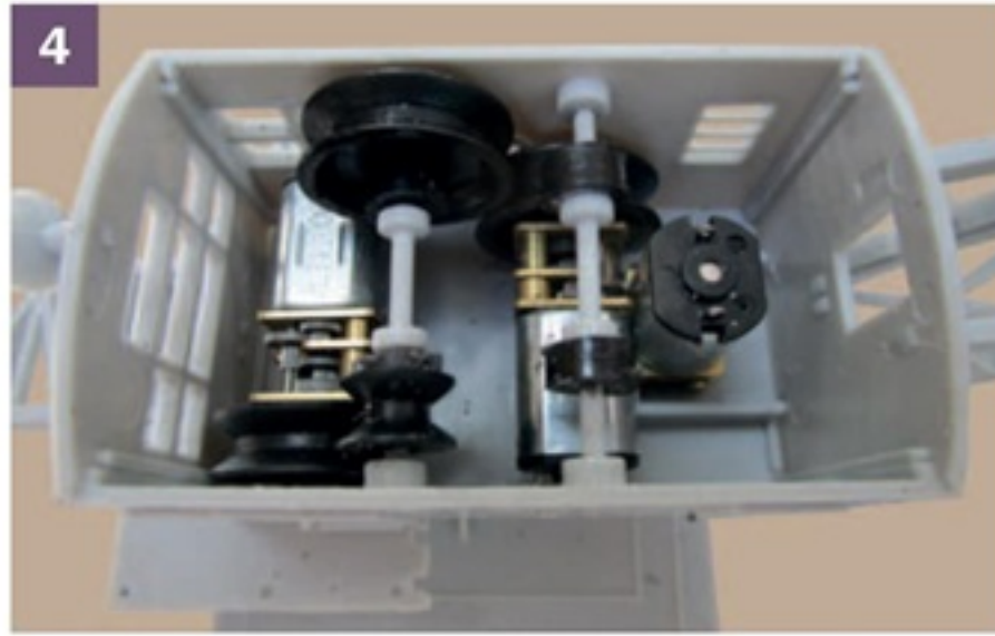
The kit spindles with additional collars and pulley wheels fitted to act as guides for the cotton 'cables'. It should be noted that the moulded-on spindle bearing collars had to be repositioned to achieve this modification.
