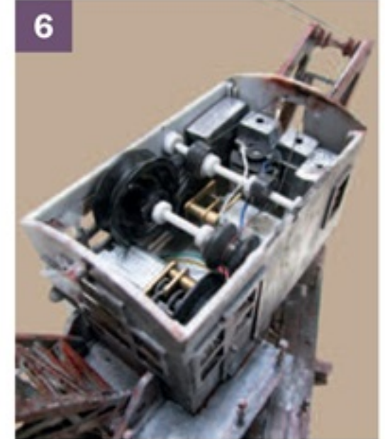
Lead fishing weights were cut to size and glued in place to help balance up the cab.
