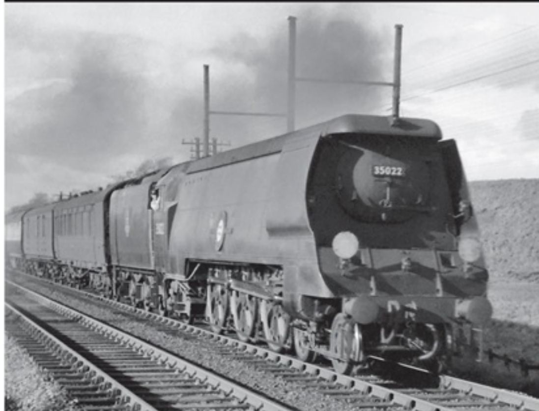
▲ Bulleid 'air-smoothed' Merchant Navy Pacific No.35022 Holland America Line is pictured near Skipton on the Settle & Carlisle line in January 1954 during blastpipe trials that were being conducted at the Rugby test plant. Note the small sections of fairing fitted in front of the cylinders. Photo: Mike Morant Collection
