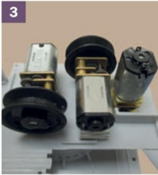
The cab base plate is pictured here with the jib and hook motors fixed in position and the pulleys fitted to the shafts.
