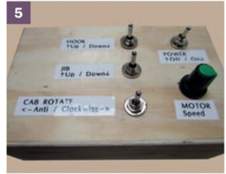
The control box for the motors. Centre biased double-pole toggle switches control the direction of the motors. Speed can be adjusted by turning the potentiometer knob (bottom right).
