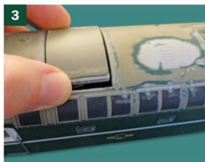
3 The roof clips were removed, and the prominent roof moulding lines were smoothed off. The new loose section was cleaned, filled, and trial fitted.
