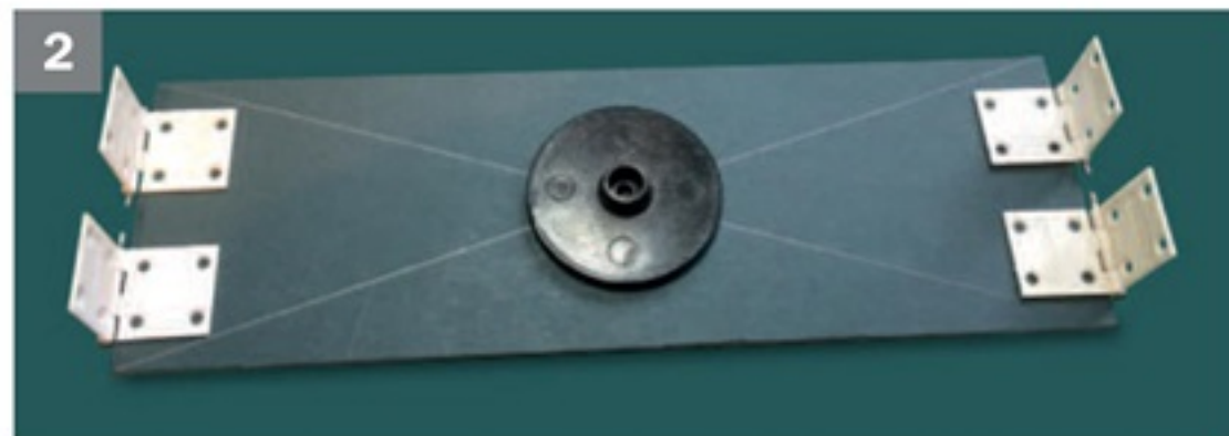
▲ The turntable deck is seen here under construction using a sandwich of plastic sheet, together with a plastic collar and hinges from recycled radio control equipment (recovered during a house clearance).
