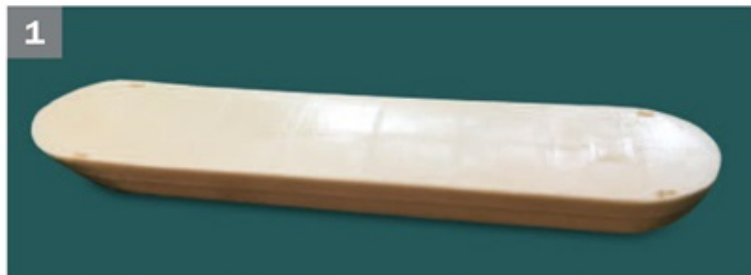
▲ Hulls are always tricky to construct and the basis of this model is a resin Maintenance Barge hull from Anyscale Models which provided a solid supporting structure upon which to construct the upperworks.
