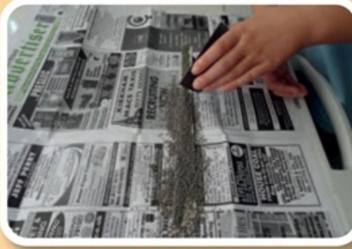
8. A sprinkling of 00 gauge ballast granules was glued to the cut card strip with a generous coating of PVA.
