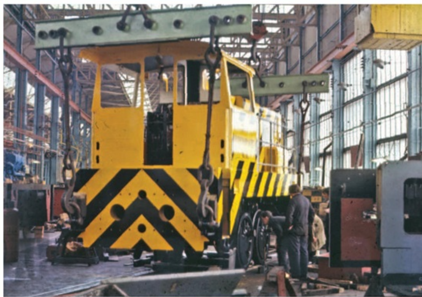
▲ A scene in Hunslet's Leeds Works erecting shop, with a 75tonne BSC locomotive being lowered and the axleboxes aligned with the horn guides – a process that has been recreated on the model.
