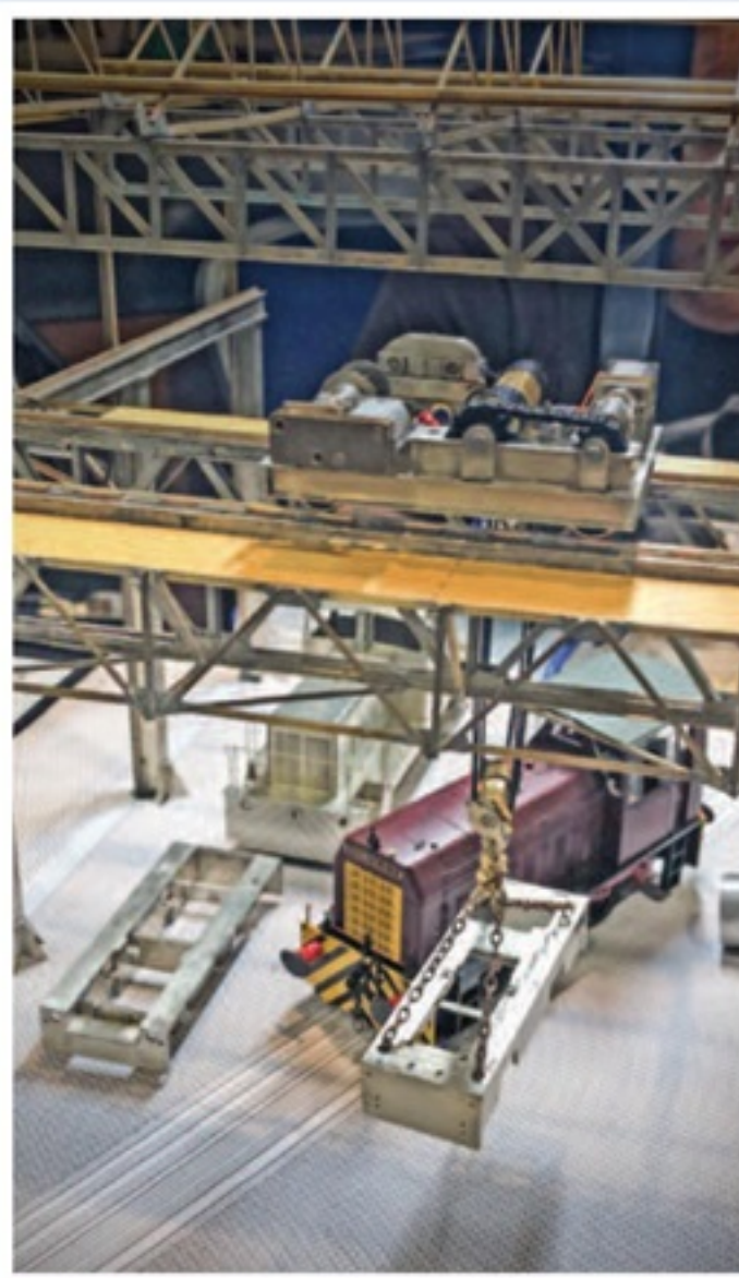
▲ The 2019 York exhibition and one of the first lifts with the crane under full DCC control. Note the gear case cover is not fitted so we could check the chain drive for the hoist was not fouling or jumping. The etched shunter in the background is a 388hp type loaned by Mike Edge to fill some space.
