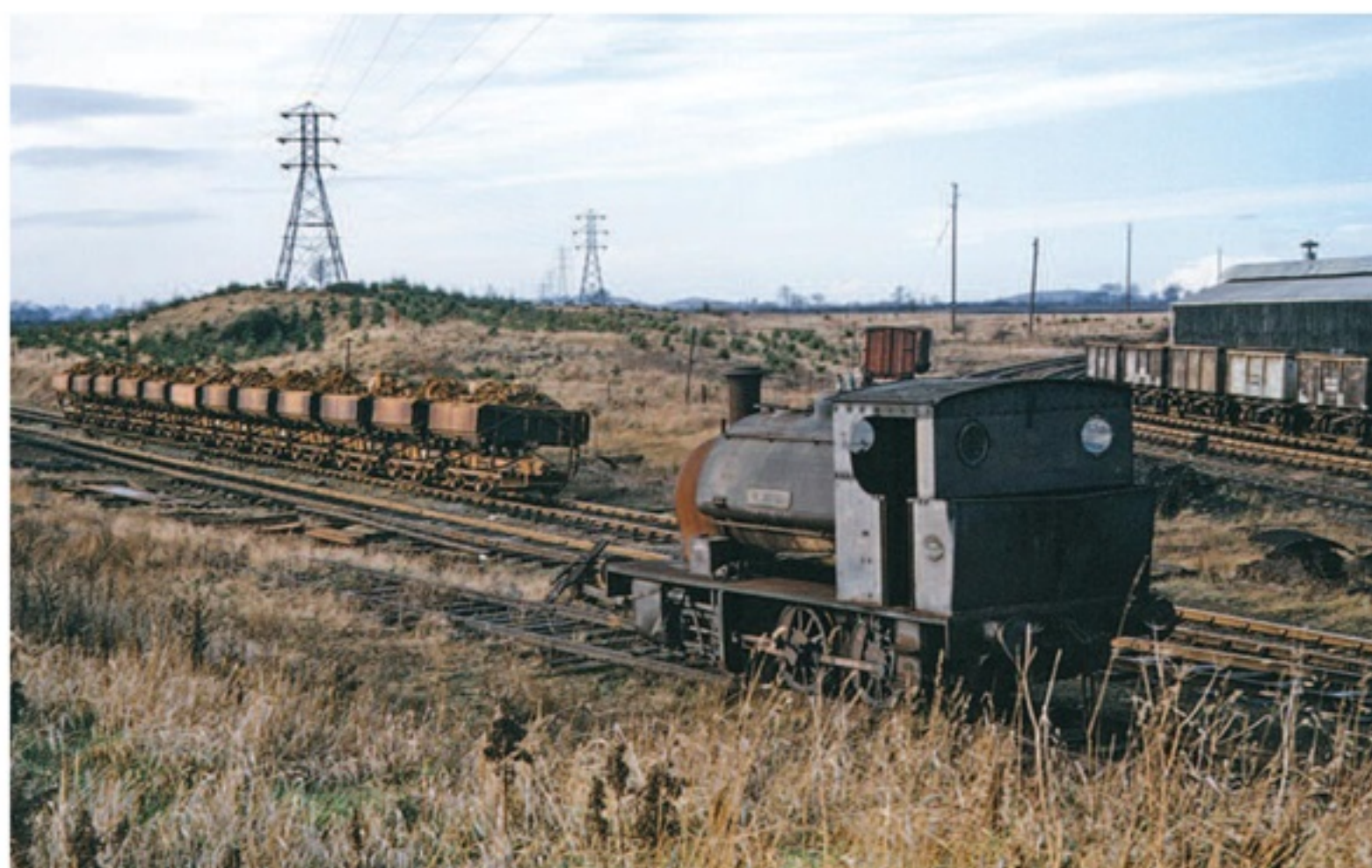
▲ The Oxfordshire Ironstone Railway was one of the last mineral lines to be built on any scale in the UK. This is a view of the line at its main works at Wroxton in November 1964. Of note are internal user side-tipping ore wagons, a 4mm kit of which is available from RT models. In the foreground is withdrawn Hunslet 0-6-0ST The Bursar of 1930. Photograph: John Cosford
