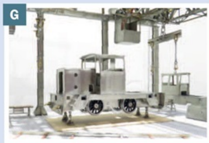
▲ The loco is positioned on the stands and the lifting gear is then detached.
