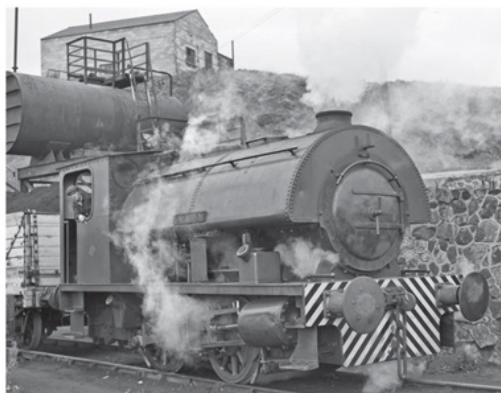
▲ 0-4-0ST Hawarden , a Bagnall built engine of 1940, is seen at the Shelton Iron and Steel Co. works in Etruria, Stoke on Trent in 1962. It is fitted with a reduced height chimney, steam dome and cab, possibly since new. Hawarden is preserved at the Foxfield Railway pending restoration. Photograph: N W Skinner/J W Armstrong Trust
