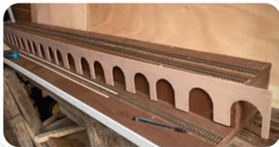
▲ The arches are cut into the plywood, first by using a hole cutter for the tops of the arches and then a fine saw to make the vertical cuts.
