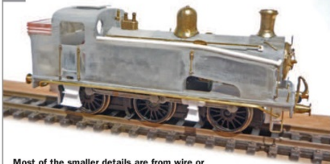
Most of the smaller details are from wire or plastic sheet and rod.
