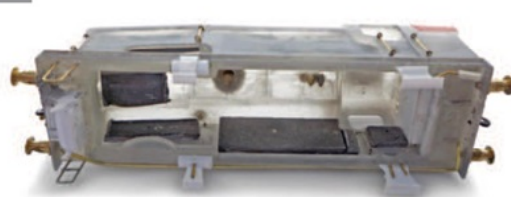
The steps were formed from styrene using a Silhouette Portrait cutter. Note the small pieces of sheet lead, which have been fixed to the insides of the tanks to bring the overall weight to equal that of the original Farish 3F model.
