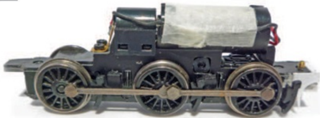
The modified Bachmann Farish 3F 0-6-0T chassis showing the plasticard extensions to the frame. The PCB has been removed to allow for fitting into the 3D printed body.
