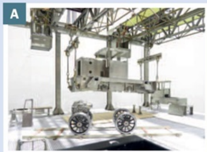
▲ The loco is picked up using the two cranes, demonstrating a 'double lift'.
