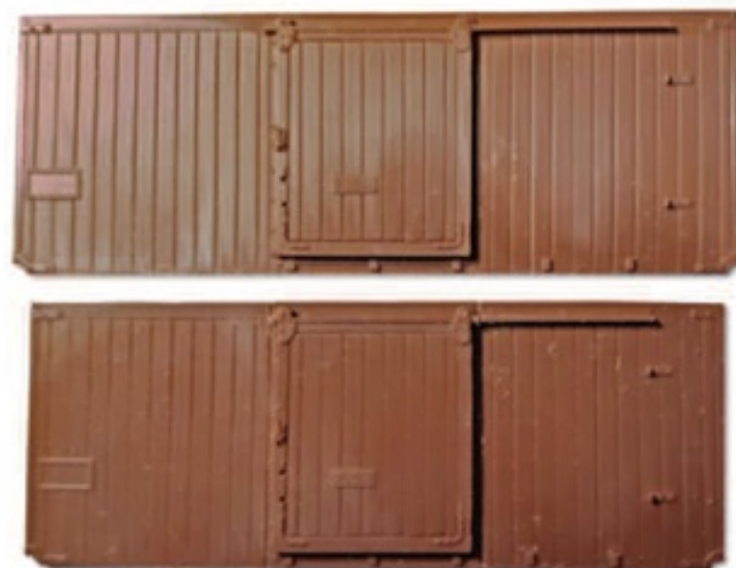
The shortened side seen next to the other side still in original condition, for comparison.
