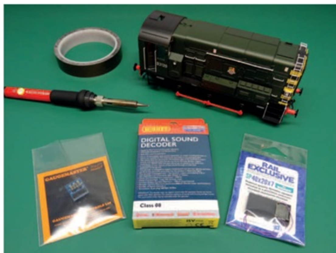
▲ The three items that were sourced to install DCC sound; a 21-pin to eight-pin adapter, a TTS sound decoder and an alternative speaker.
