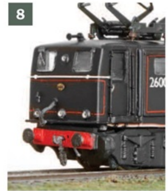
▲ A close up of the cab showing the electric lamps which replicated the conventional train headcode discs widely used at that time.
