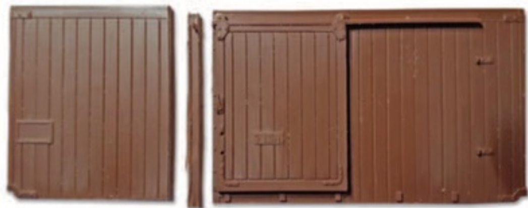
One plank has been removed to the left of the door. A similar cut will be made to the right of the door.
