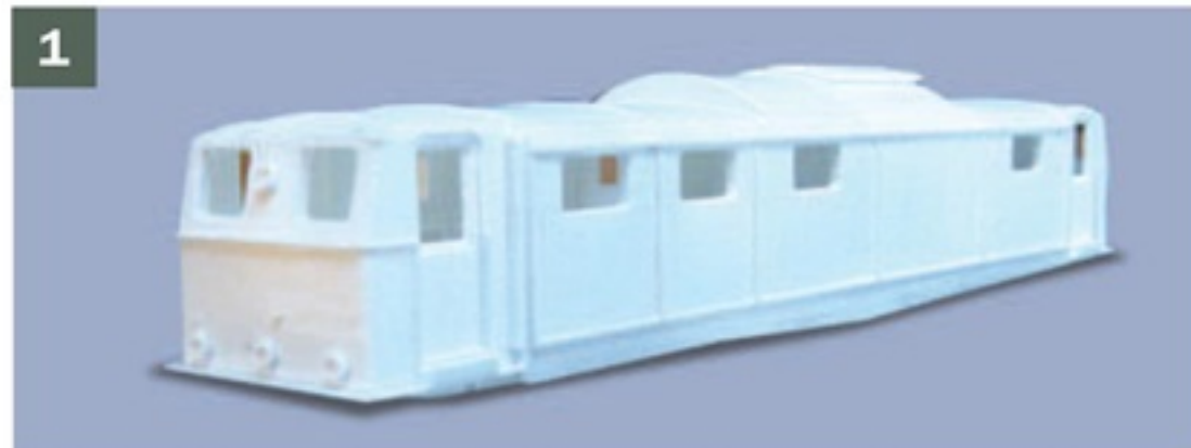
▲ As supplied the 3D print shows the strata lines of the layered printing process. These were smoothed off during the build process.
