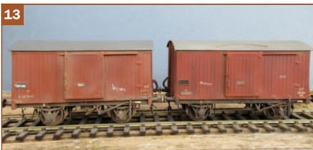
The shortened Dia.083 on the left, alongside a Dia.134 van, with the longer wheelbase previously made from the same kit, but built as intended.
