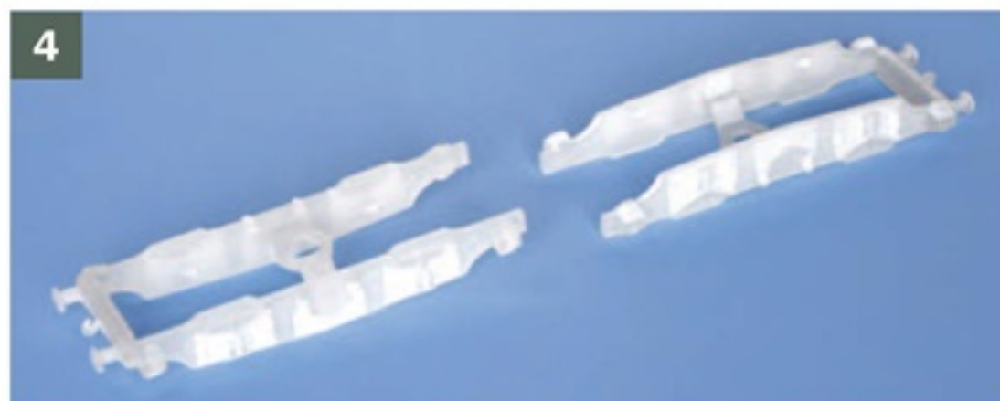
▲ Each bogie framework (shown upright and inverted) comes as a one piece 3D print, complete with buffer beam. The mounting plate is not required for this conversion and was removed.
