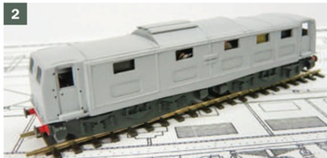
▲ In grey primer and following several passes with some fine emery paper, the print lines are invisible.
