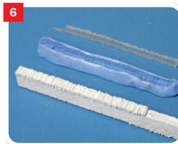
▲ The mock-up or 'master' plasticard wall with the slate copings alongside the latex mould and a length of cast resin copings.
