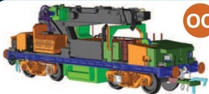
Plasser GPC 12t Crane
