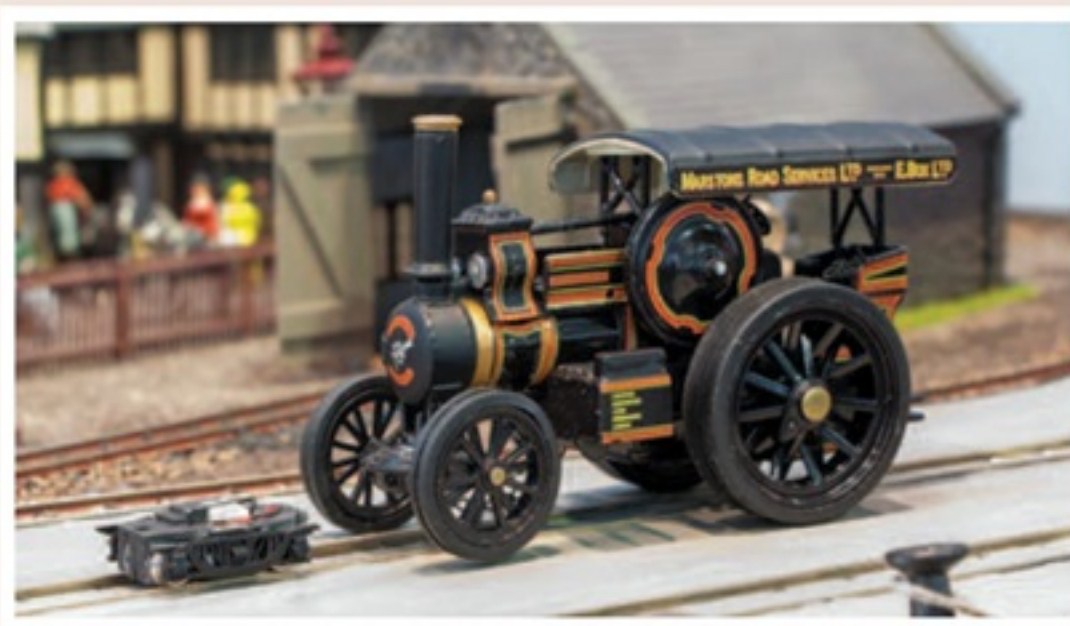
▲ The tiny powered bogie from a Kato Portram N gauge tram model.
