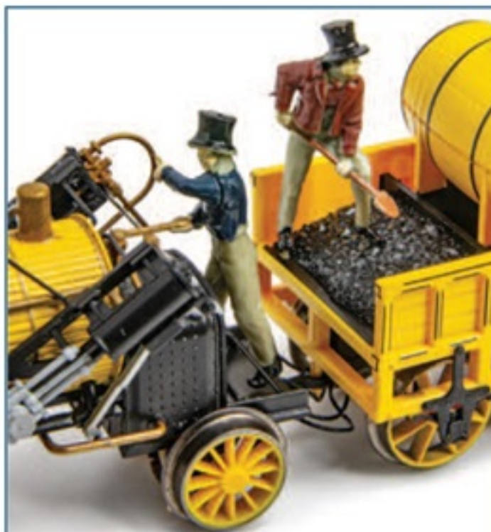
▲ The supplied crew figures have spigots on their feet that engage in holes on the model.
