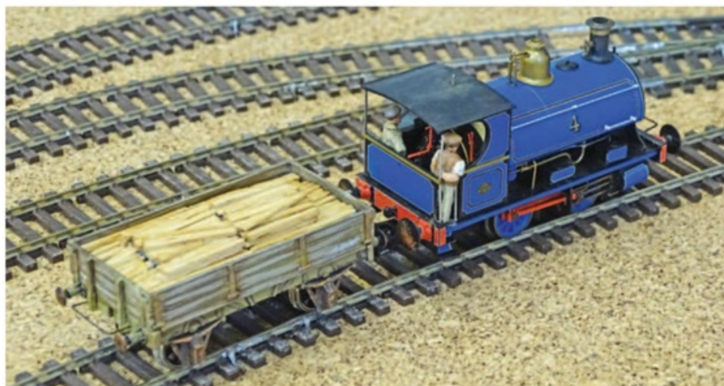
▲ Peckett 0-4-0ST No 4 seen with its runner wagon. The wires and the permanent coupling link are virtually invisible from normal viewing distances.
