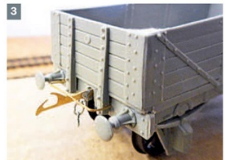
▲ Modified Sprat & Winkle couplings are used for wagons which must be uncoupled.
