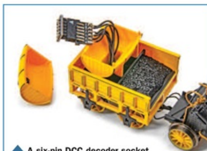
▲ A six-pin DCC decoder socket is housed in the water barrel on the tender.
