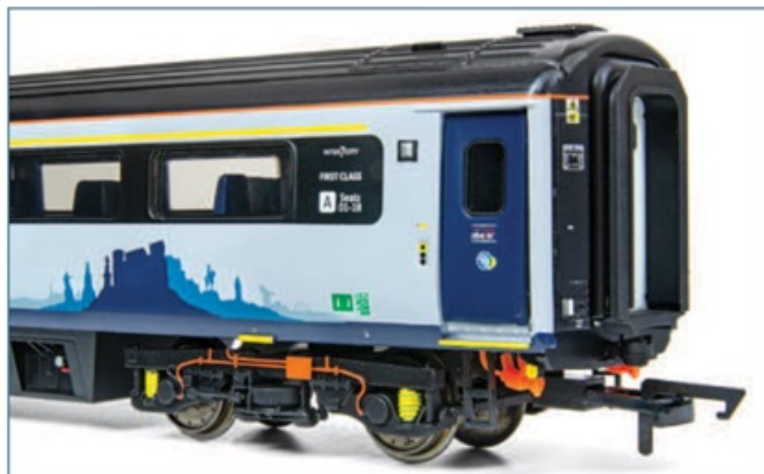
▲ A detail view of the TGFB. Models are supplied with tension lock couplings in body-mounted NEM pockets.
