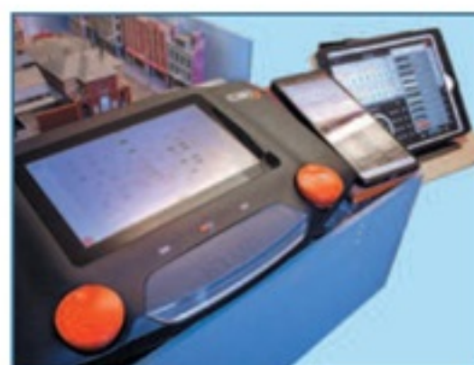
▲ CS3 control operations can be replicated on remote devices like mobiles and tablets via Wi-Fi.
