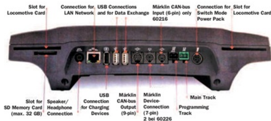
▲ Rear connections include LAN, USB, power, DIN and speaker sockets.
