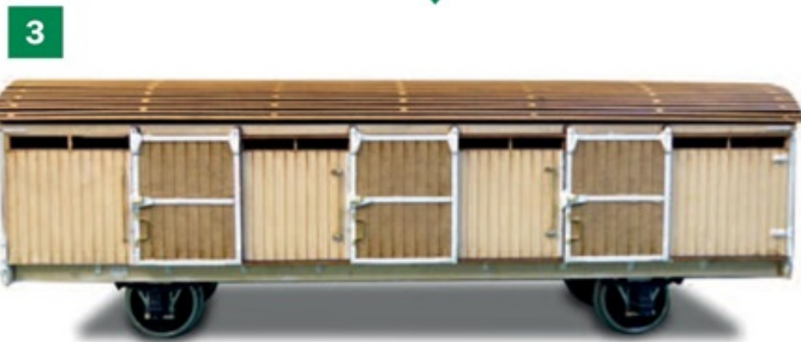
▲ The bodywork is glued and clamped to ensure squareness.
