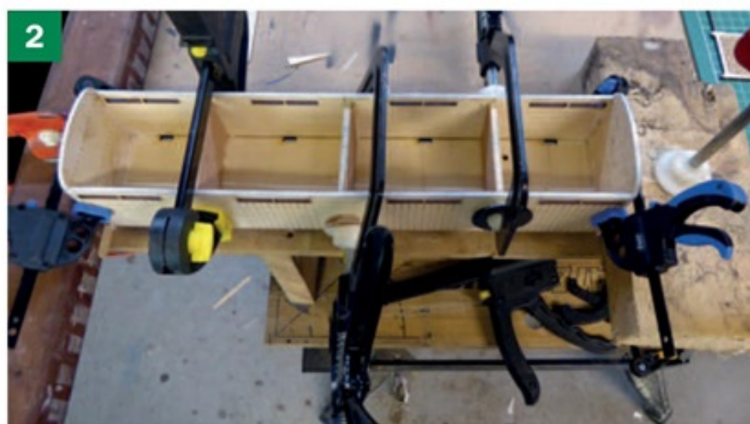
▲ The bodywork is glued and clamped to ensure squareness.
