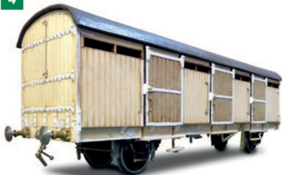
▲ Final detail parts are added and a roof covering applied and painted.
