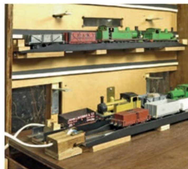
▲ This is the stock box with its lid lowered to provide a deck for the cassettes. Two items to spot here are the slide-out stop blocks which also cut track power, and the angle brackets in the stock box itself (top of photo) that support the train cassettes in transit.
