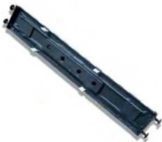
▲ Two lengths of rail were fixed to the underside to prevent the weight from bowing the frame.
