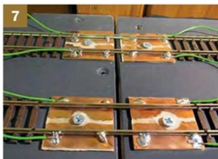
7 Screw the mica tiles down and solder the rails to the copper surface. Feed and return wires are also soldered at this stage.
