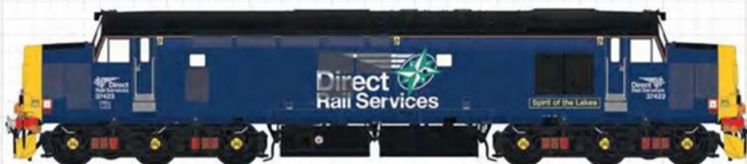
37423 'Spirit of the Lakes' DRS Simplified Compass (2018 onwards) - WIPAC light clusters, top headlight & MU socket on nose
