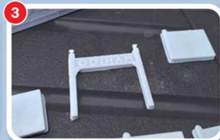
▲ The 3D printed running-in board and fencing prior to painting. Photos: author
