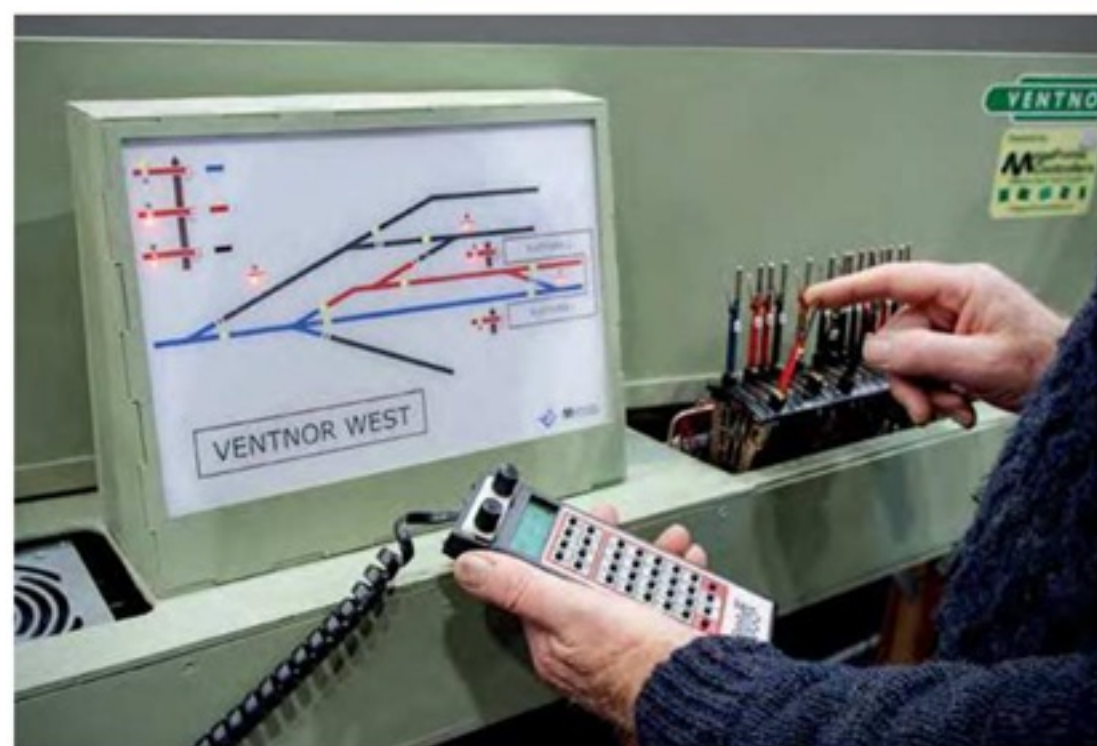
▲ A view of the mimic track diagram, lever frame (to operate the points and signals) and Digitrax DCC controller for train control.
