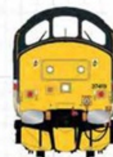
37419 'Carl Haviland 1954-2012' InterCity Mainline (2019 onwards) - LED tail lights, MU socket & plated bodyside window
