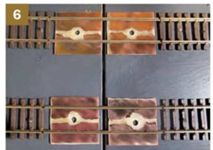
6 Grind away the copper layer in the middle (to isolate the rails from each other) and drill a securing screw hole in the centre.
