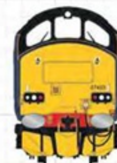
37423 'Spirit of the Lakes' DRS Simplified Compass (2018 onwards) - WIPAC light clusters, top headlight & MU socket on nose
