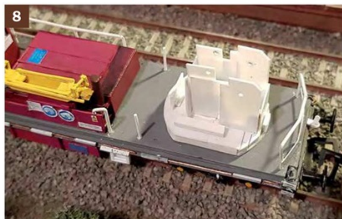
▲ The crane housing under construction, with jib holes drilled.
