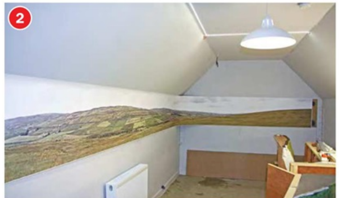
▲ A trip to Teesdale to take photographs and time on the computer stitching and 'Photoshopping' them produced a high-resolution backscene. The image was printed and suspended with double-sided tape along the top edge.
