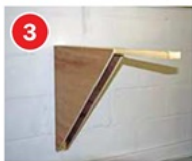
▲ Layout supporting brackets were made from plywood offcuts from the loft conversion and 2" x 1" timber from the layout-moving crates. This saved the obstruction of too many legs beneath the layout.
