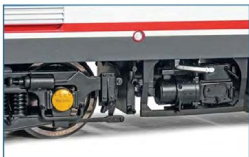
▲ The Westinghouse 3VC75 compressor is well modelled.
