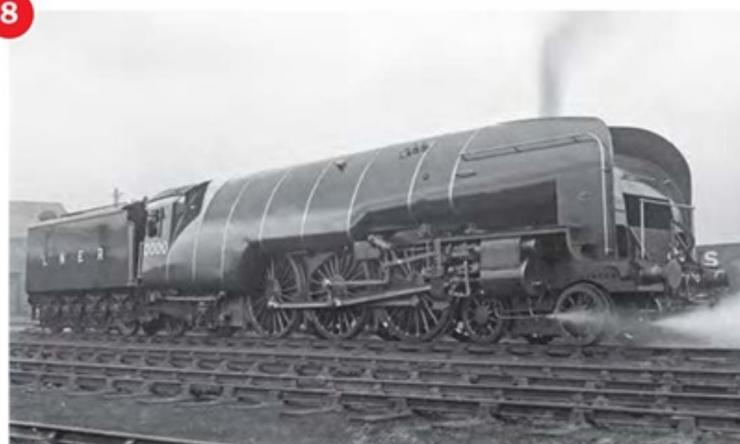
▲ The 'Hush-Hush' 4-6-4 No.10000 at Doncaster in 1930, with its original high-pressure water-tube boiler. Photo: Rail Photoprints Collection
