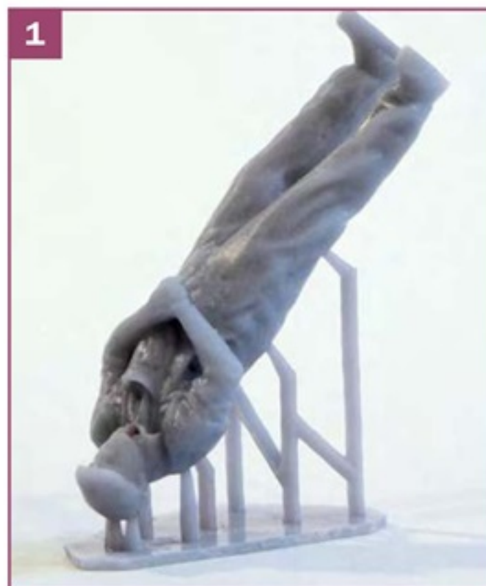
▲ The 3D printed figures from Hardy's Hobbies arrive with the support framework which has to be removed and smoothed with care.
