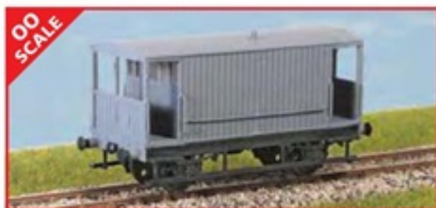
PC58 LMS (ex MR) 20 ton Goods Brake Van 849 built between 1924 and 1927. In general traffic they survived into the 1960s, while those in Engineer's fleet lasted into the 1980s.
