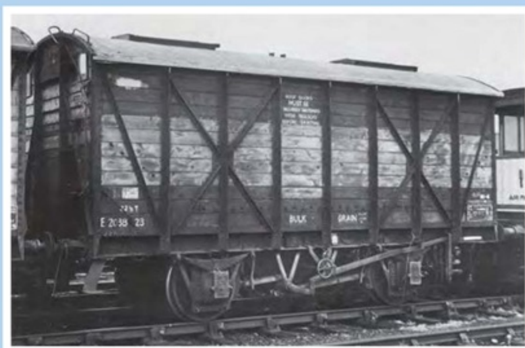
▲ The LNER wooden bodied grain van to Diagram 51 of 1929. This example No.E203823 is seen in rather careworn condition at Hull docks in 1969. The side hatch is absent and some of the bodyside planking appears to have been replaced. The lettering on the side says 'Roof doors must be securely fastened with padlocks before shunting'. I wonder if the padlocks had separate keys – and if so did they travel with the vehicle? Photograph: David Larkin
