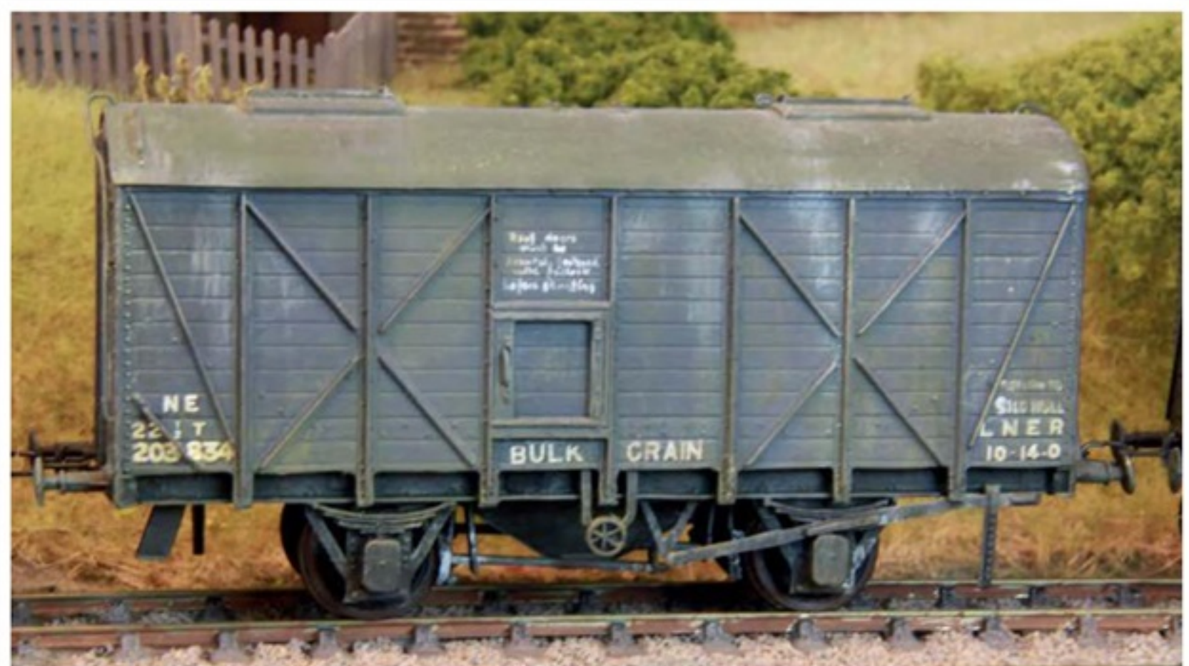
▲ In 1937 the LNER adopted a much smaller NE logo for its wagons. This change didn't affect the chosen livery colour of LNER grey, but it did coincide, fortuitously, with the upgrading of the weight to 22½ Tons, which was due to the fact that weight had been saved in construction of the later batches. Note that the inspection hatch, above the word BULK, appears on one side only of the wagon.
