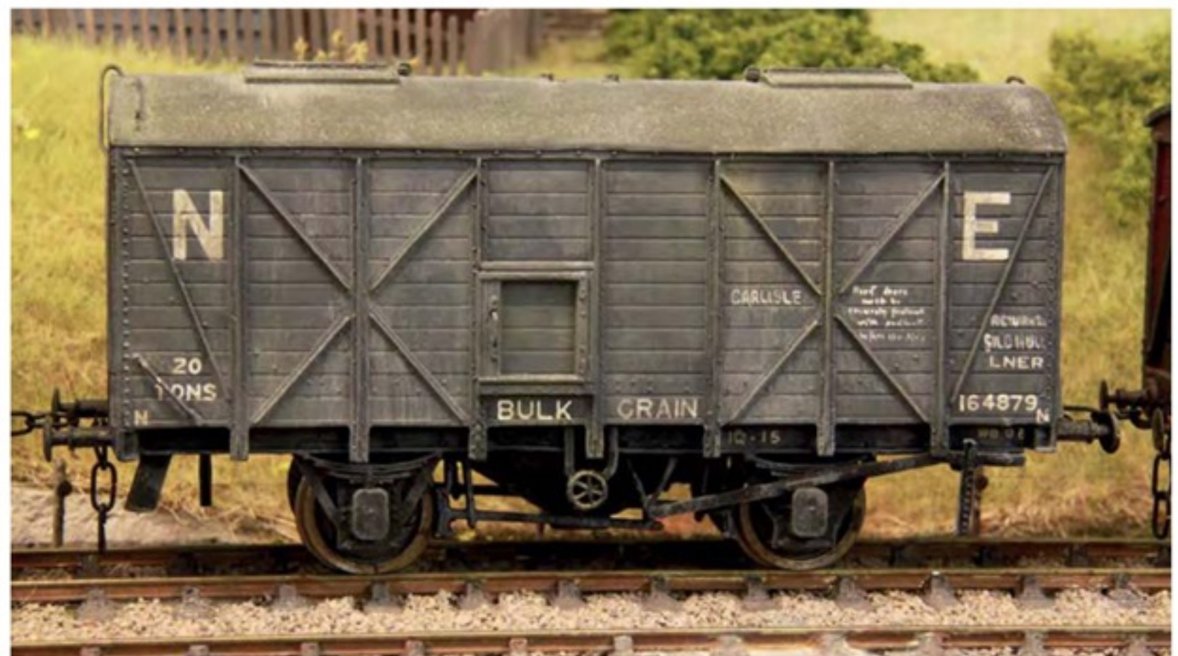
▲ The first of my Parkside kits in the pre-1937 livery, and thus rated 20 Tons. The tiny script to the right of the word Carlisle – my chalked destination for the van – reads 'Roof doors must be securely padlocked before shunting', or the nearest I could manage with my mapping pen and Pelican Plaka ink. I confess to not being utterly convinced by the axleboxes; they are neither the split RCH type, nor the classic LNER variation.
