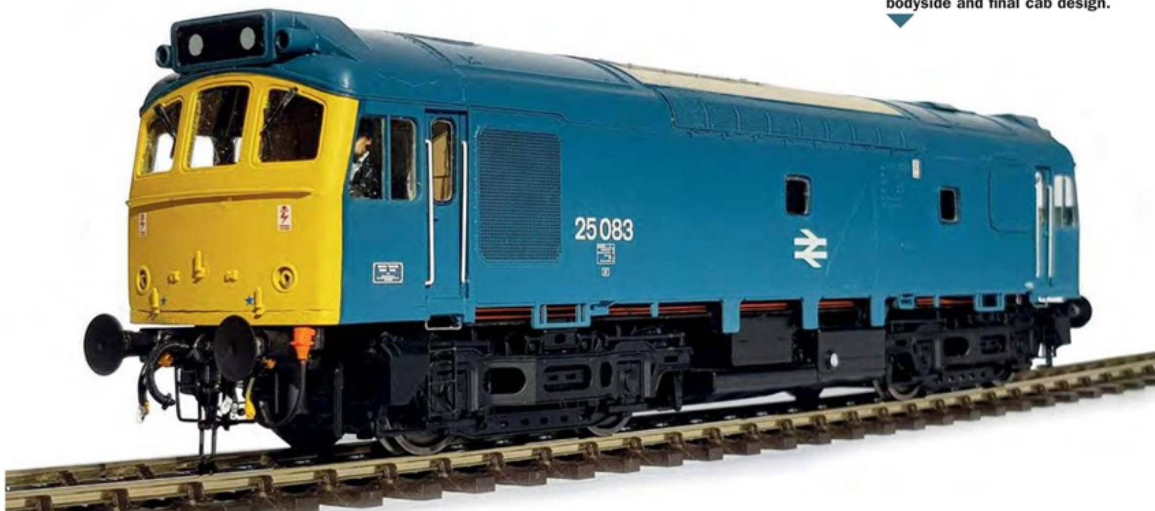
No.25 083 showing the flush bodyside and final cab design.
