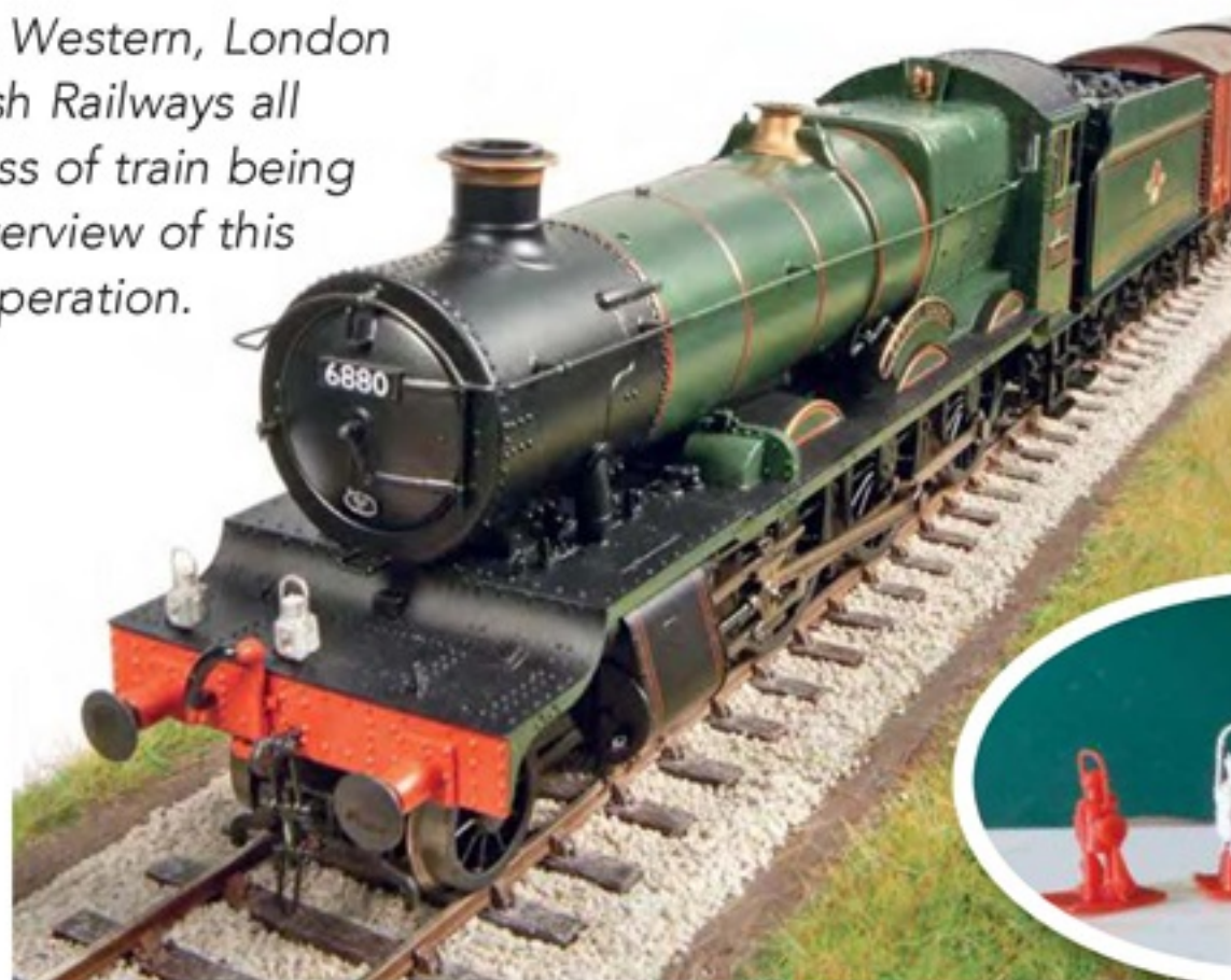
◀ A Hornby Collett Grange Class 4-6-0 displaying a Class C headcode, at the head of a fitted freight. The Modelu BR(W) lamps are 3D-printed in a red compound (inset), which are painted with white enamel before detaching from their bases.
