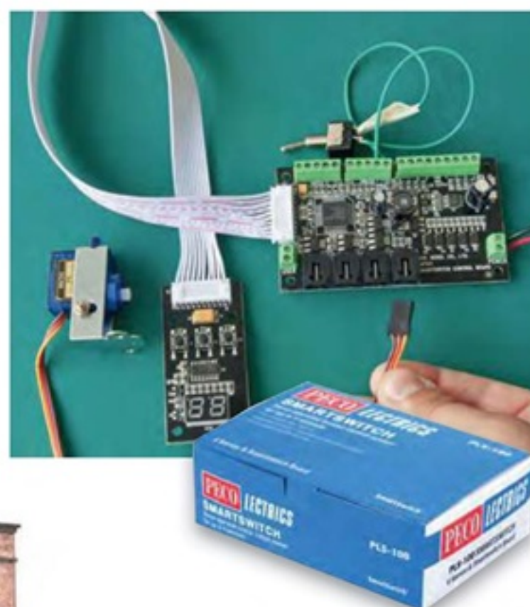
From rods and cranks to electronic control for points and signals. The Peco SmartSwitch offers plug-and-play ease of installation.
