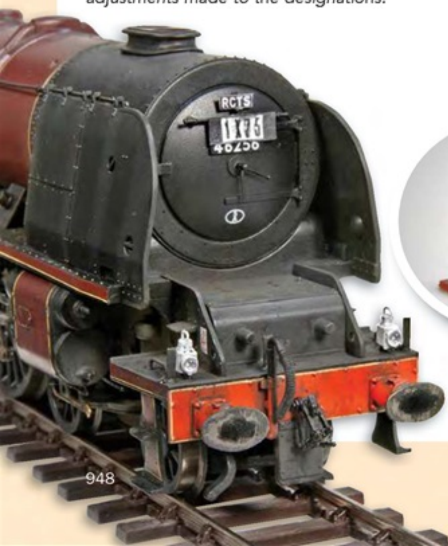
◀ A Coronation Pacific displaying a Class A (express passenger) headcode using Modelu BR(M) lamps; these are supplied with separate self-adhesive lenses, attached after painting.
