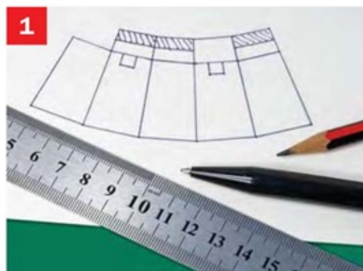
The template was used to mark out the whole of the tower base onto a sheet of card (recycled from a cereal packet), which included gluing tabs for assembly.
