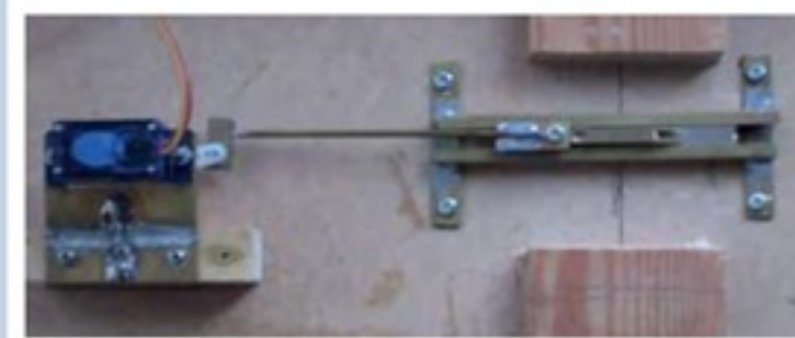
▲ On-off control of the buses is effected by a servo-movable magnet under the board.
