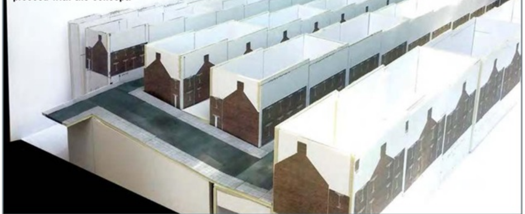
The mock-up to test the concept of forced perspective. It was not part of the pre-build for the TV show but a trial to see if our ideas were sound. The result gave us the impetus to proceed with the concept.
