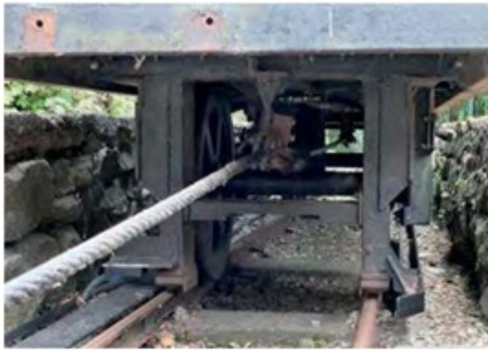
▲ The cable is secured firmly to each end of the cars. Guard rails keep the rail heads clear.
