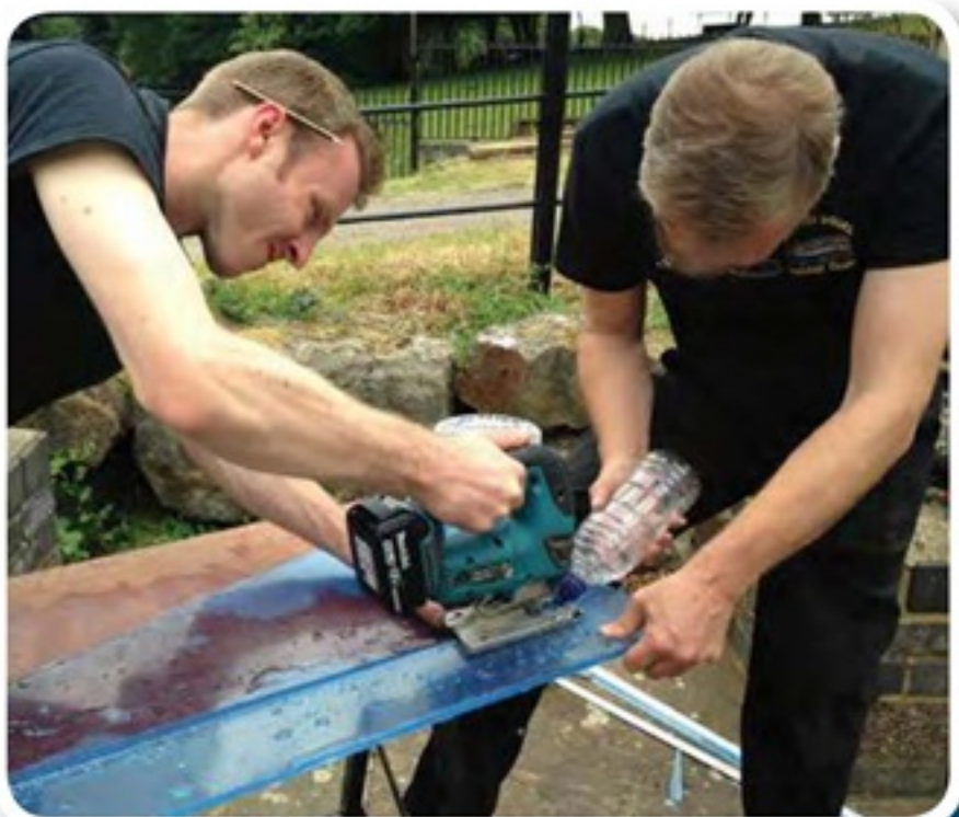
◀ Fin and Karl hard at work creating the invisible sky track out of Perspex using an ad hoc cutting blade water cooling system.
