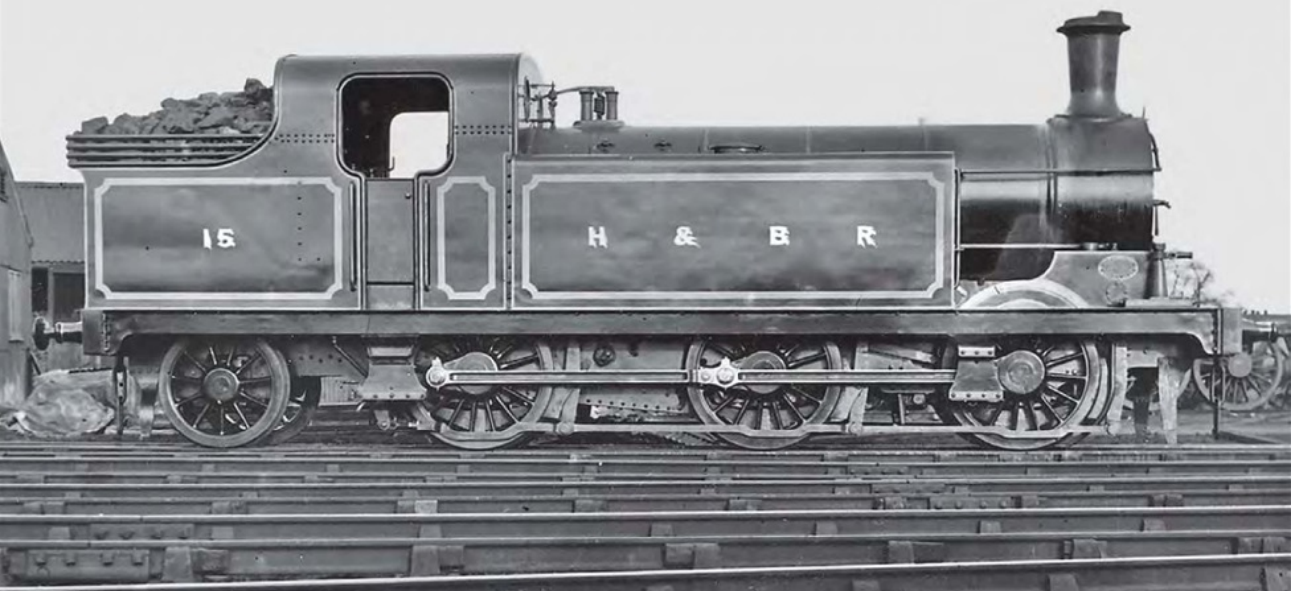
▲ F3 No.15 in original condition seen at Springhead c.1913. It clearly shows the panelled lining and the fine trim lining (although the monochrome film does not differentiate between the ultramarine and vermilion shades). The device attached to the front buffer beam (and not shown on the drawing) is a re-railing jack which was often carried by H&BR locomotives. Photo: Mick Nicholson collection
