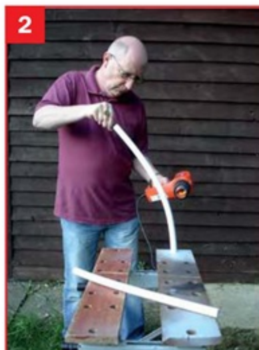
Pipe bending – me demonstrating the pipe bending technique used for getting the curve in to the main arches.
