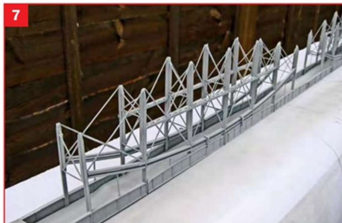
Once back at home I could concentrate on all the fine construction details without the pressure of a deadline. In place is the bridge deck, the vertical trusses, suspension chains and cross bracing.
