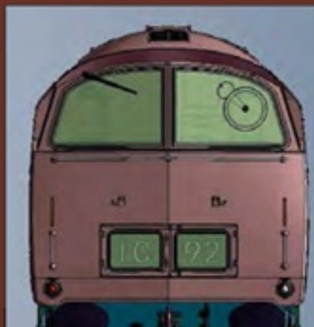
A CAD drawing showing the Clear View Screen as fitted to D1039.
