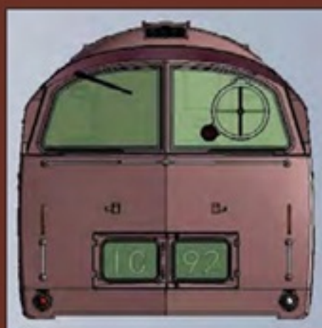
A CAD drawing showing the Clear View Screen as fitted to D1006.
