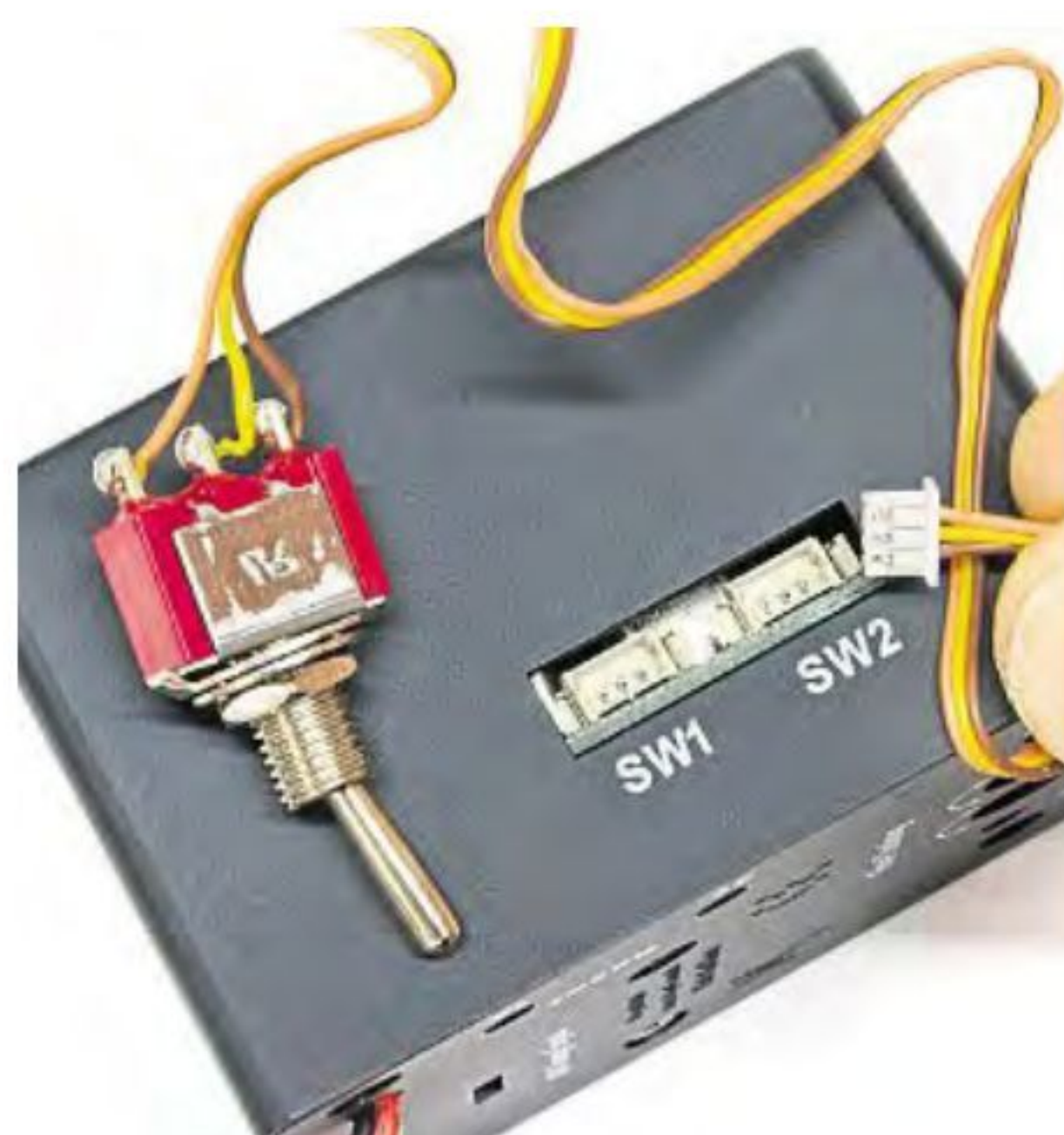
Pre-wired double pole, double throw switches are supplied with the signals and plug into the 'Power Base'.
