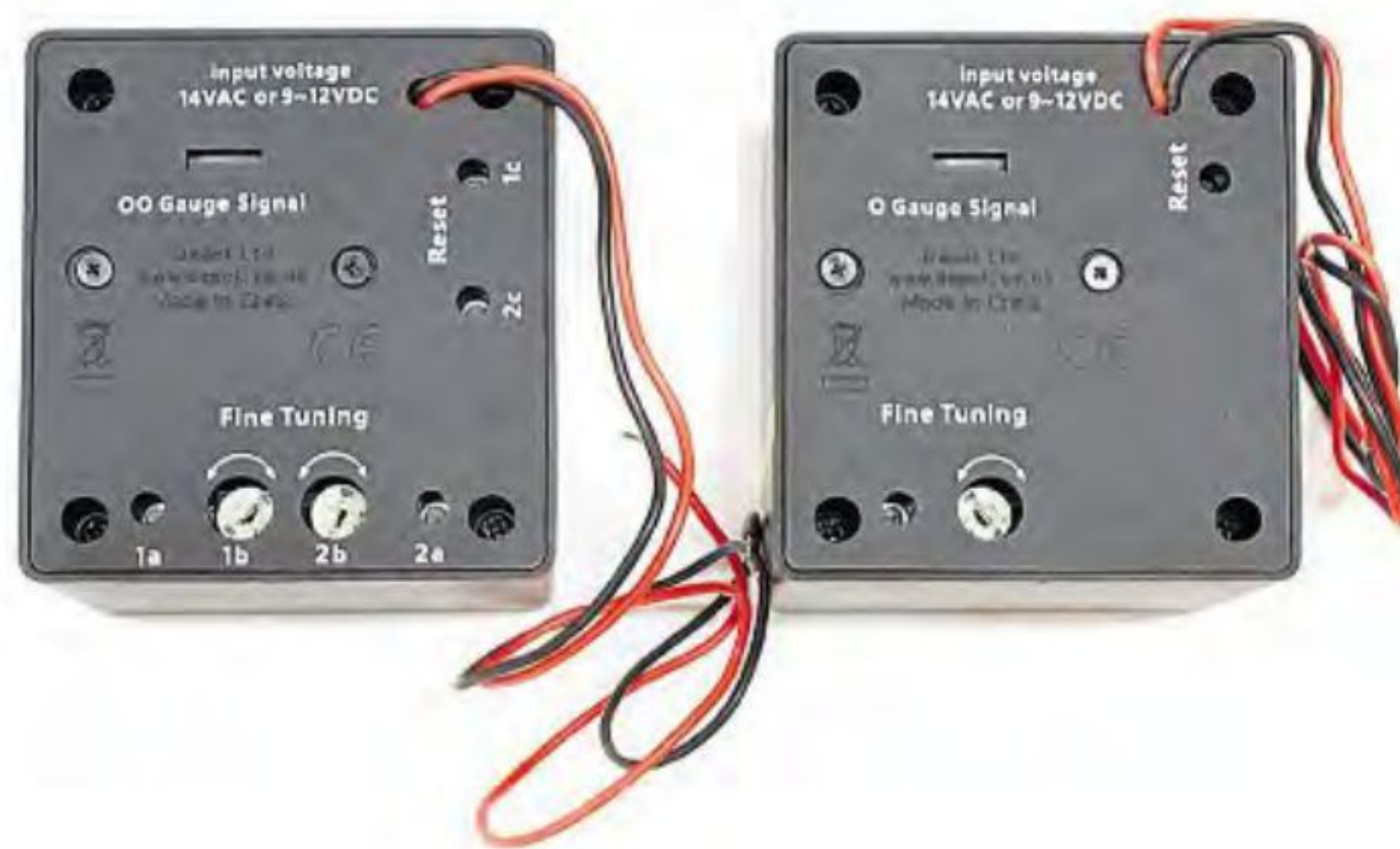
Fine-tuning controls are situated on the underside of the 'Power Base' box, making adjustment easy when signals are installed on the layout, with the box located under the baseboard. The various controls are clearly labelled and the enclosed instructions explain how to fine-tune the signals and reset the controls to factory default settings.
