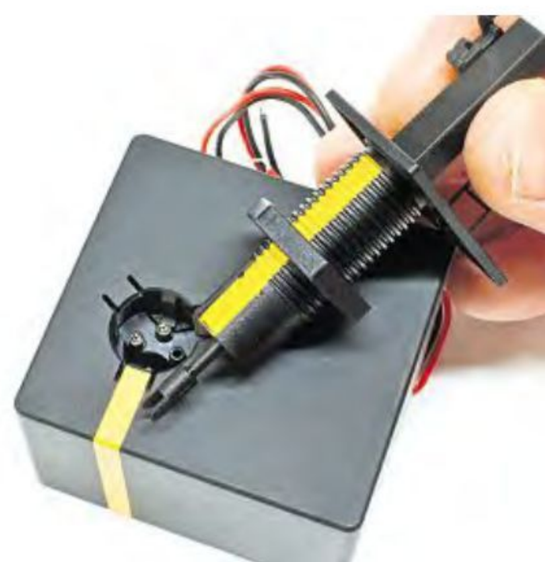
The signals are worked with a new servo control unit, the 'Power Base'. The signal plugs into the base, making both mechanical and electrical connections to operate the arms and illuminate the oil lamps.
