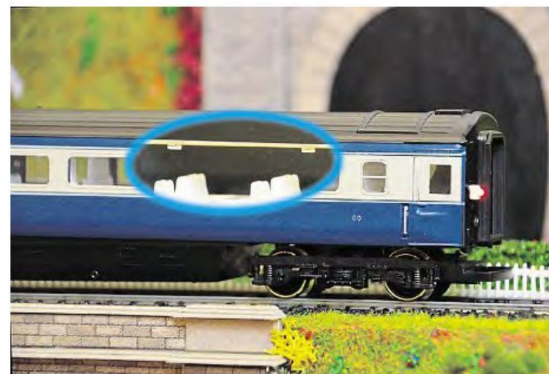
Fitting Train-Tech coach-lighting strips requires just the temporary removal of the roof. Note also the carriage's tail-light.
