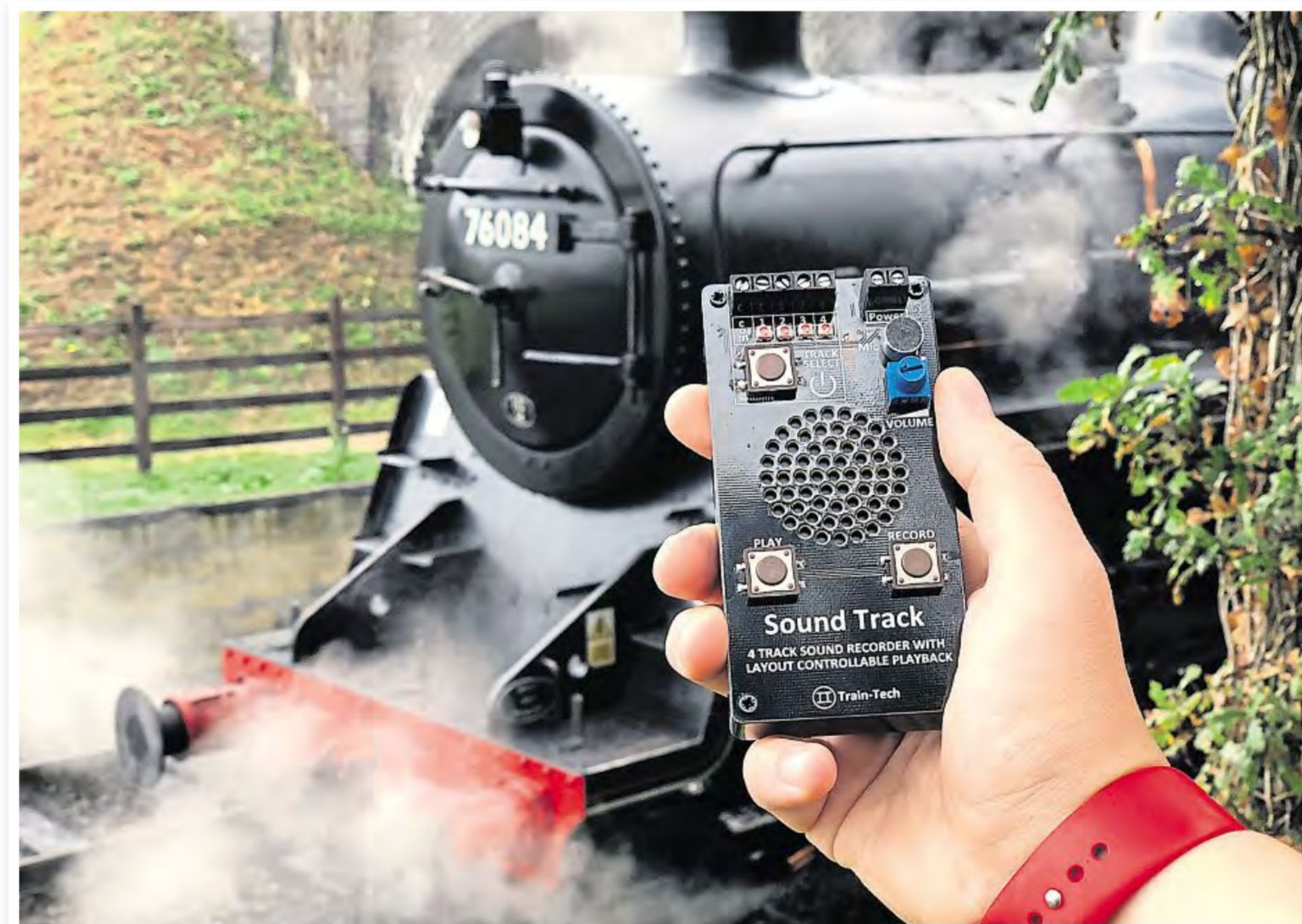
Train-Tech's Sound Track recorder (SR1 Sound Track, £69) is seen in use at the North Norfolk Railway. The recorder enables modellers to record their own sounds, take them home and replay them automatically on their layouts.
