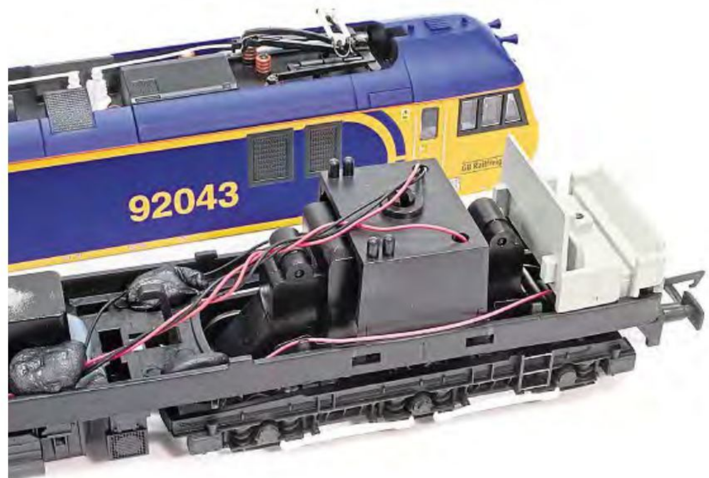
A single self-contained drive bogie fitted with a five-pole skew wound motor is fitted at one end of the model.
