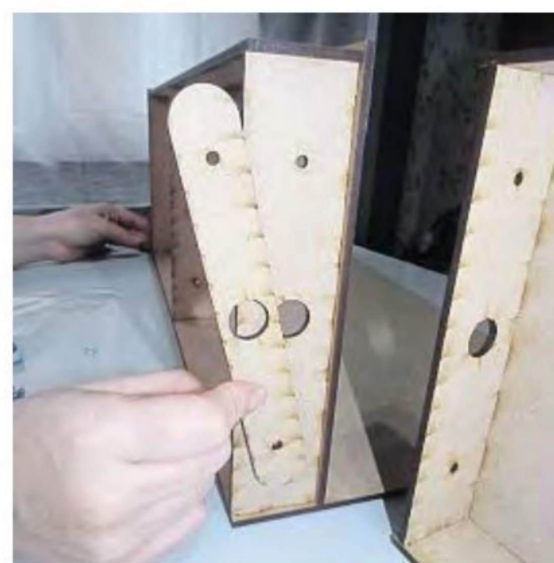
The bottom plinths are joined together at the centre using the spacers, M5 nuts, bolts and washers provided.
