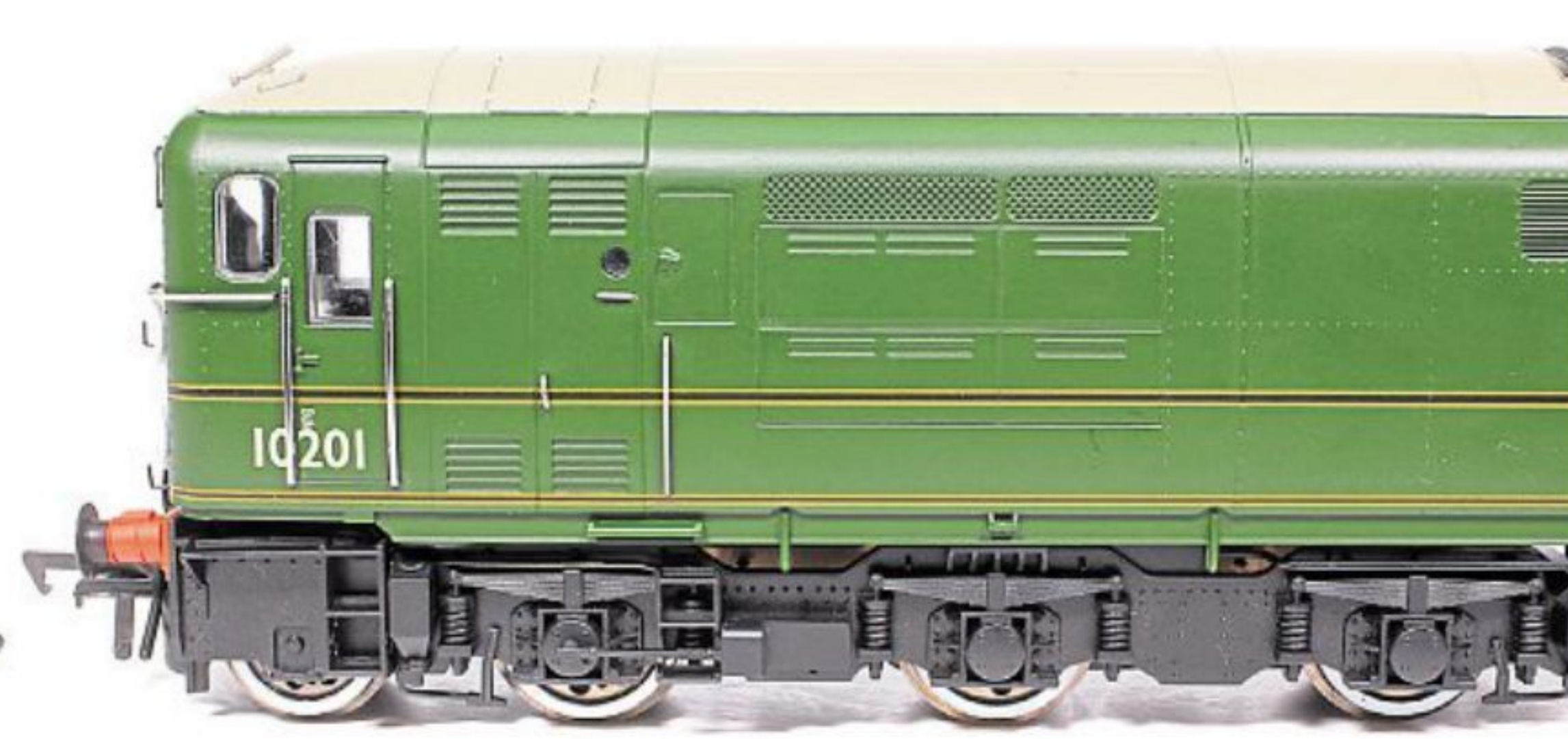
This view shows how the model sits on its bogies. Despite the small gap which is very close to prototypical appearance, the bogies rotate freely.
