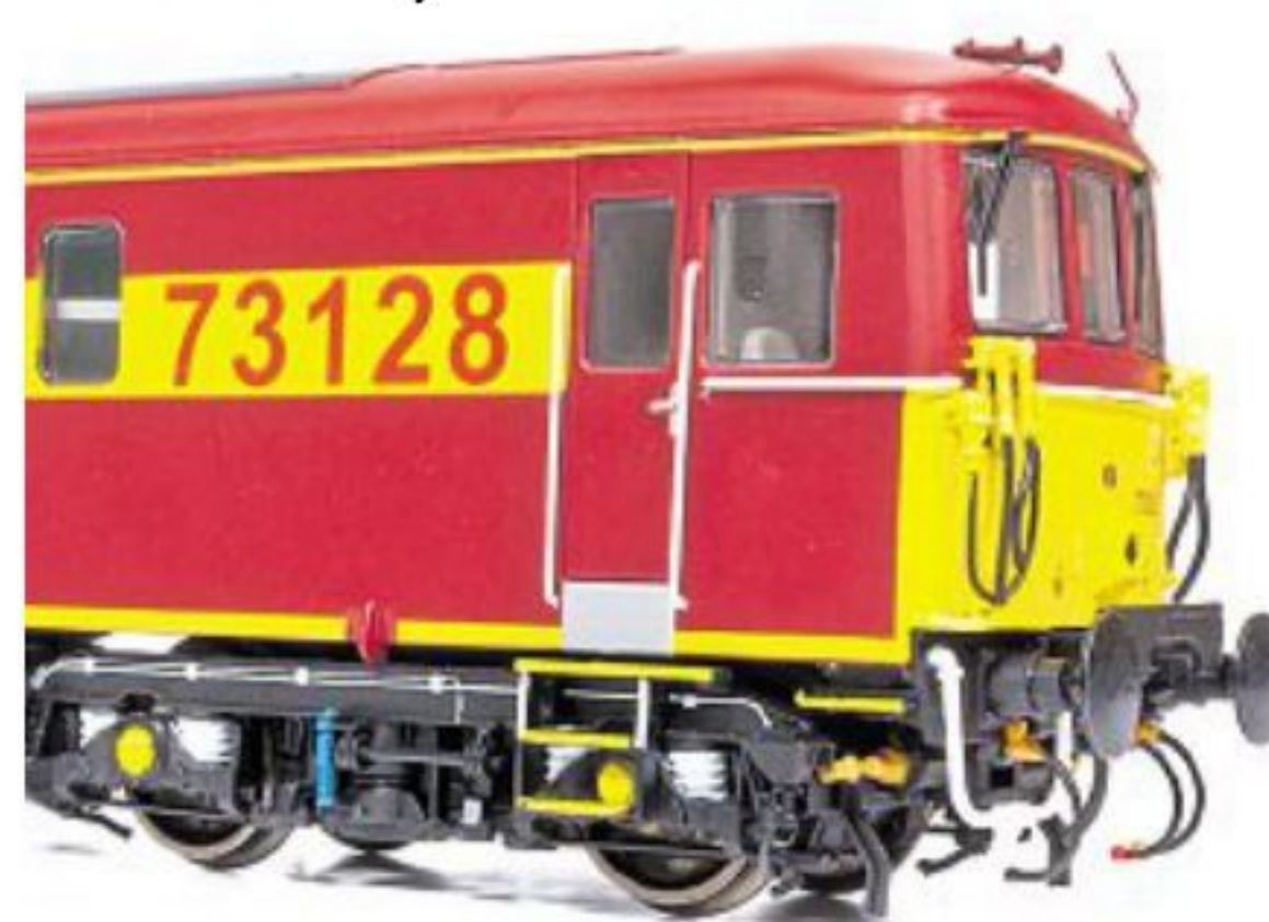
Detail on the bogies has been picked out in different colours including the footsteps, springs and axle box covers.
