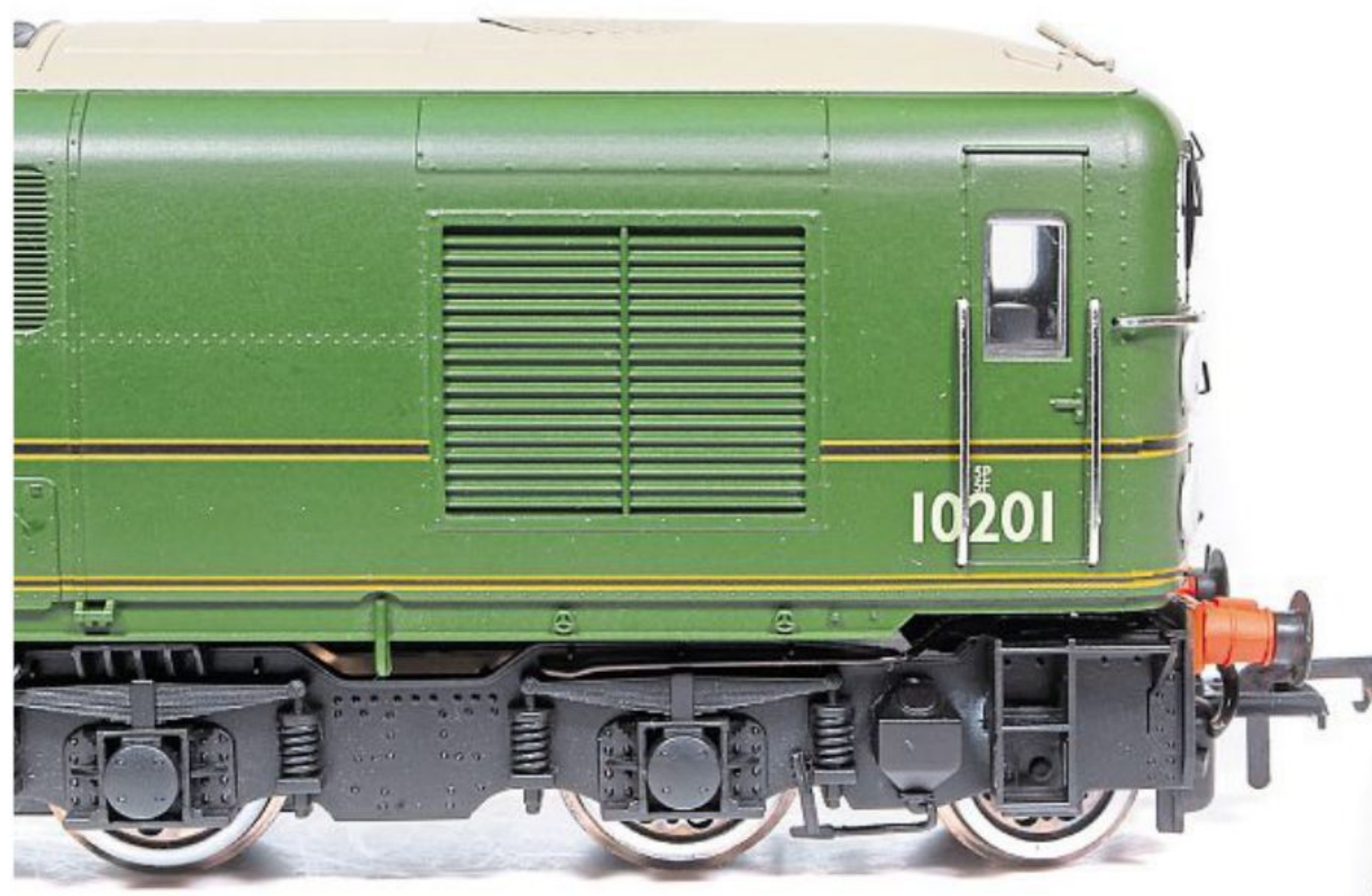
Radiator grille detail can be seen in the body sides.
