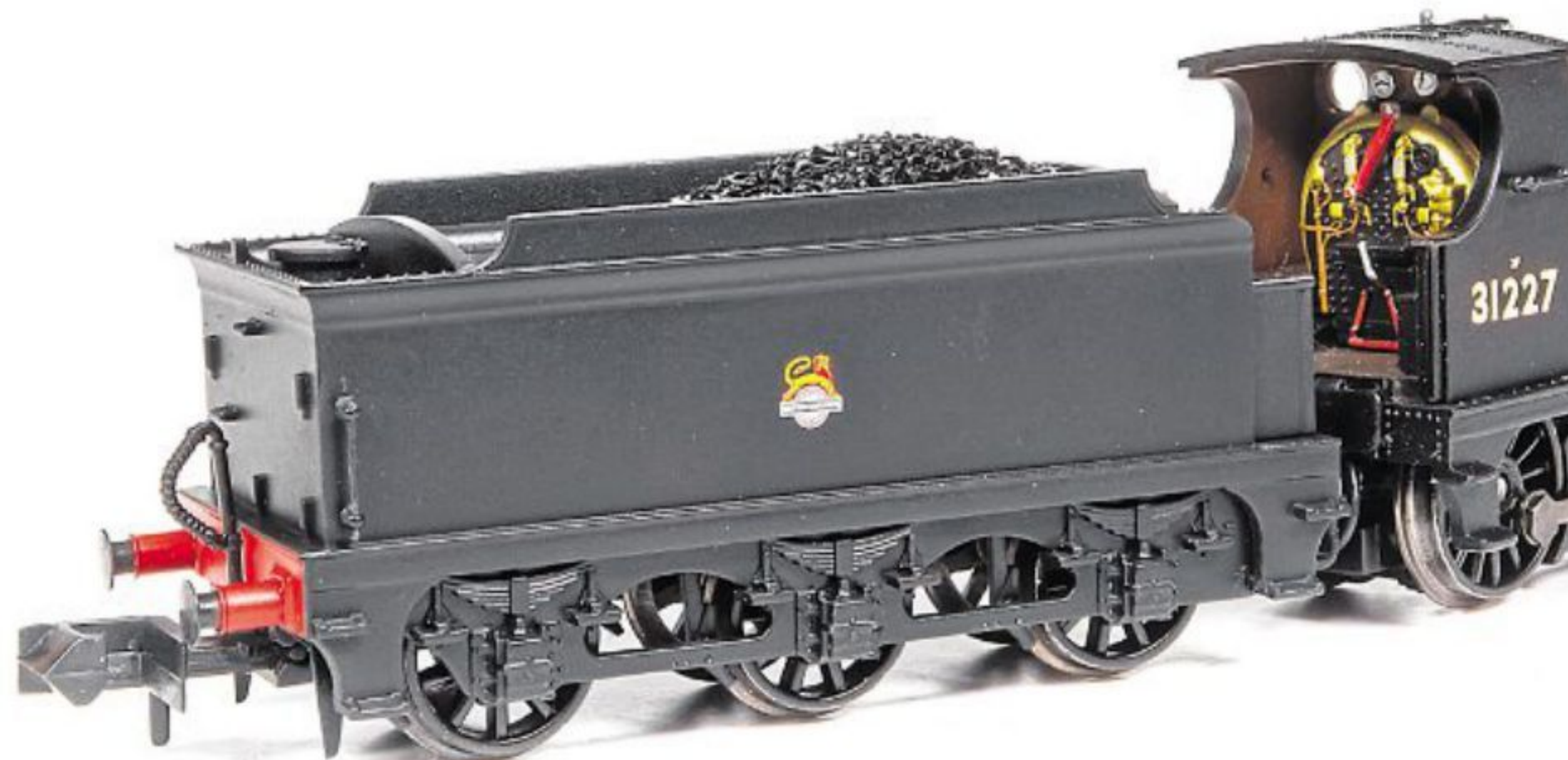
The detailed cab back head includes individually fitted dials, sight glasses, driving controls and firebox door equipment, all painted neatly with appropriate colours.
