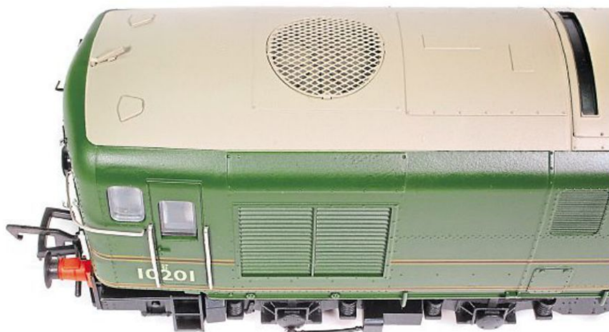
The cooling fan is composed of etched metal allowing a view of the fan grille fitted behind it.
