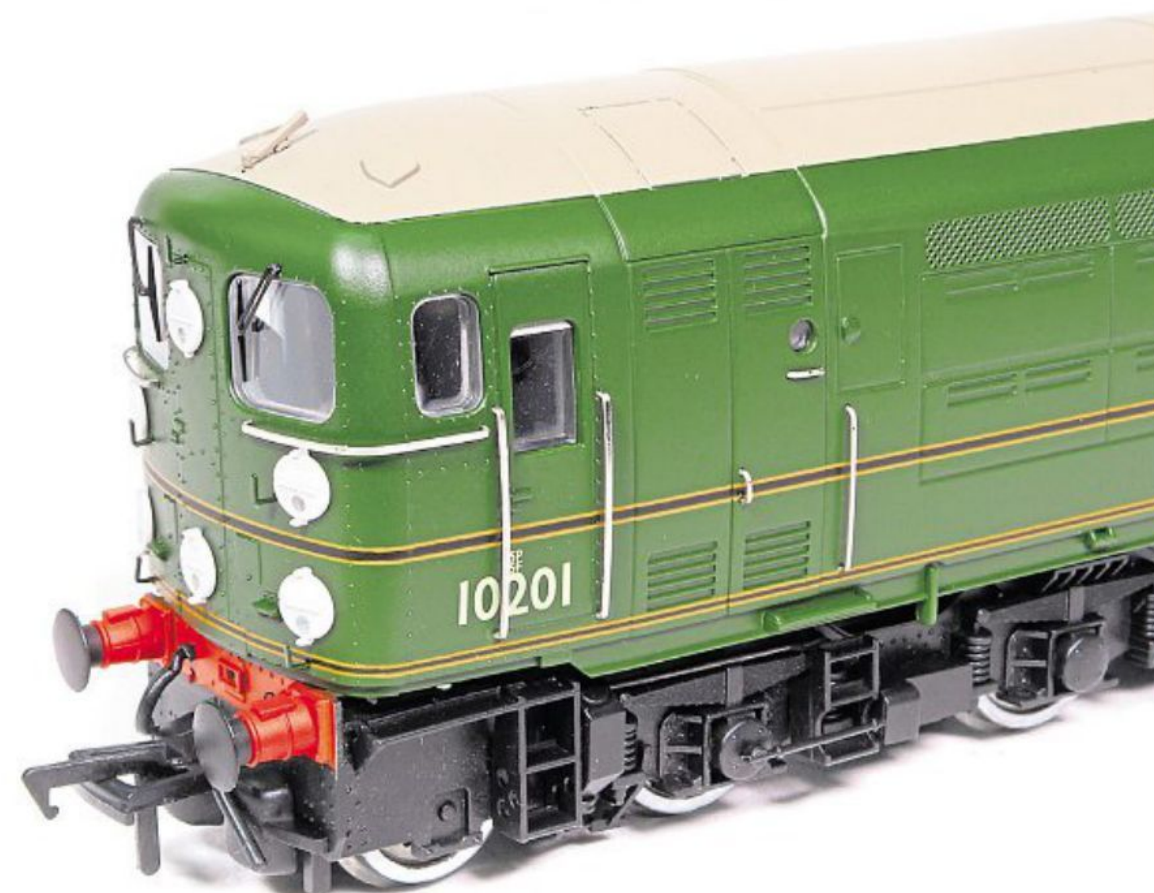
Small details applied to the cab fronts include separately moulded train reporting discs and windscreen wipers. Power classification was 5P5F, the same as a 'Black Five' 4-6-0.
