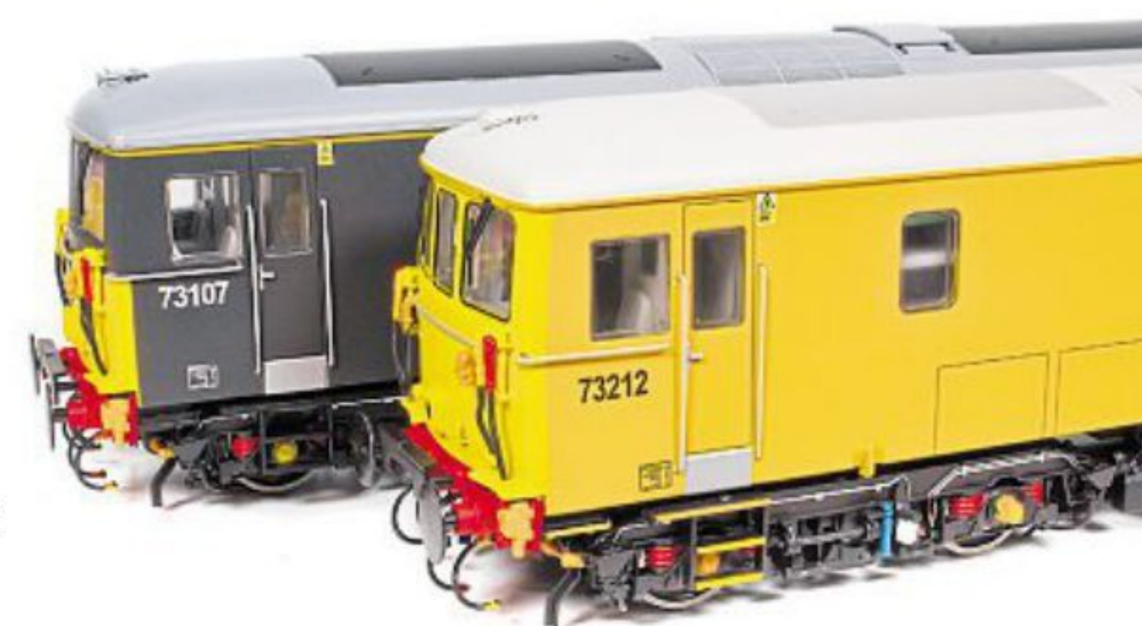
Right: Detailing of the Dapol OO-gauge Class 73s includes accurately moulded parts for the waist-height air pipes and multiple working cables.
