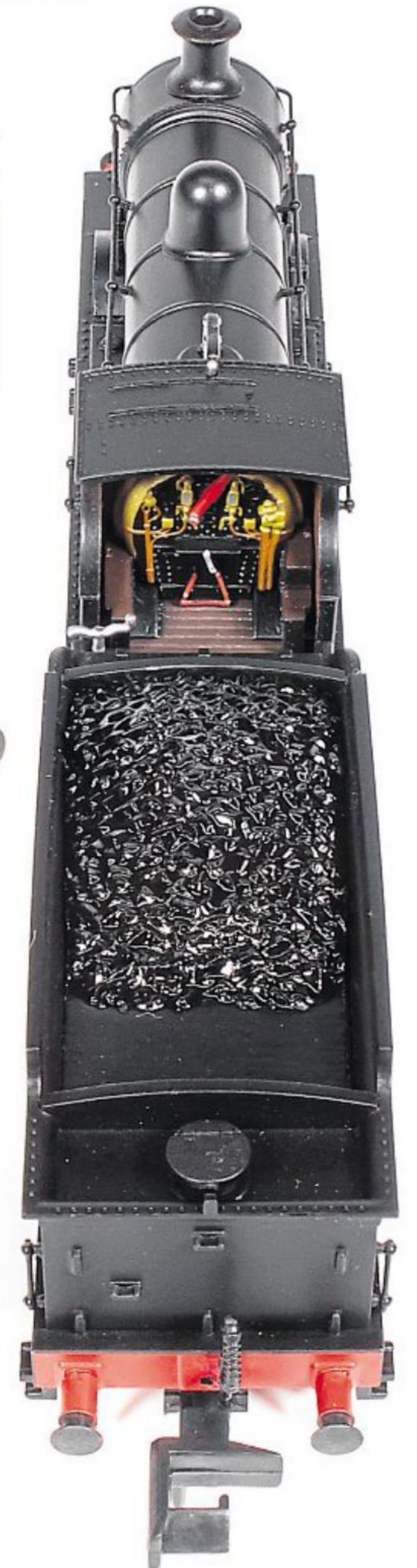
This view from the tender shows the removable coal load and detailed cab. The use of a small coreless motor means that no visible parts of the mechanism intrude into the cab.
