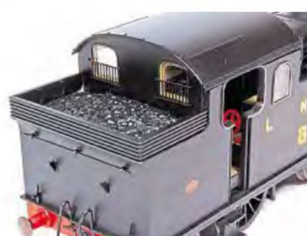
The coal bunker has plastic coal rails and load. Note the fine glazed windows with their coal guards.
