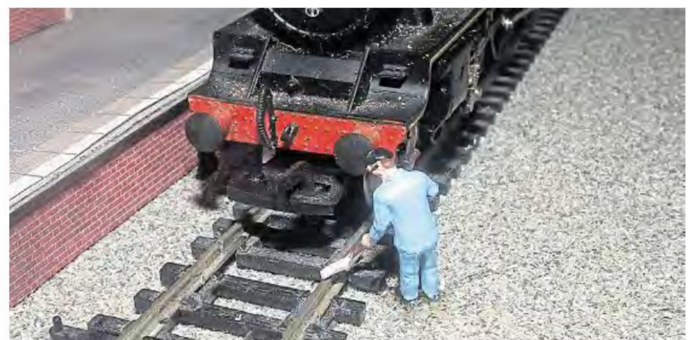
A member of the permanent way gang noticed that every time he rested his spade on one of the rails, the loco started to move. The problem was solved – a loose rail-joiner had moved so that the two rail ends were no longer actually joined!
