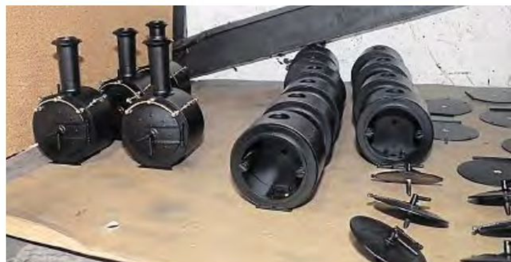
Smokebox castings await their incorporation into the new 0-4-4-0 live steam models.
