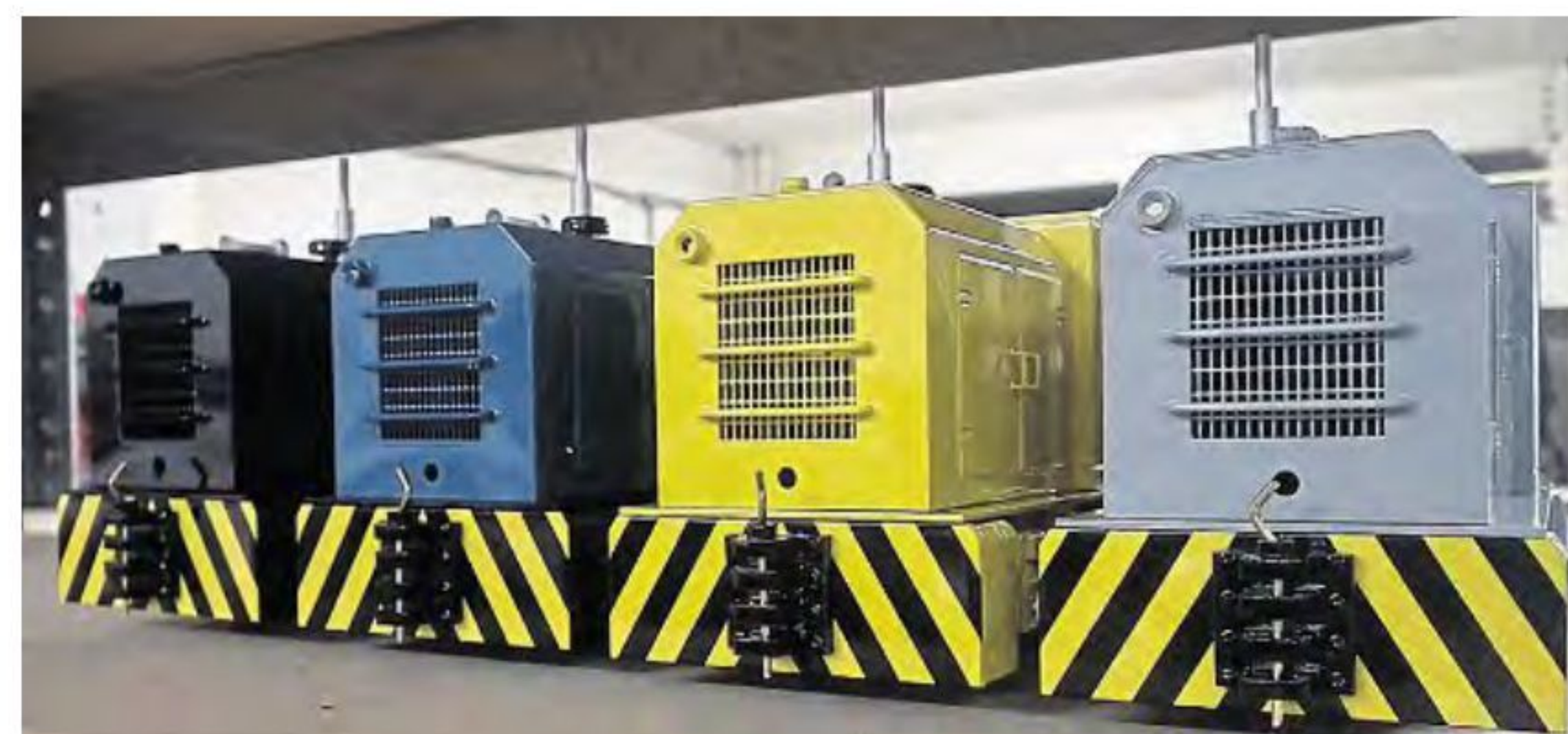
'Hercules' battery-electric diesel shunters waiting to go.
