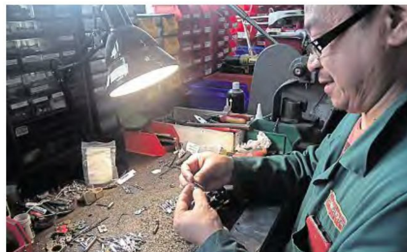
Marou painstakingly builds up one of the bogies for a double Fairlie.
