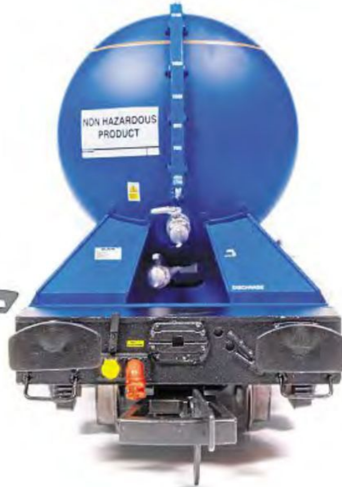
Headstock detail includes the multiple working wiring sockets allowing the trains to be run in top and tail formation with two compatible locomotives.
