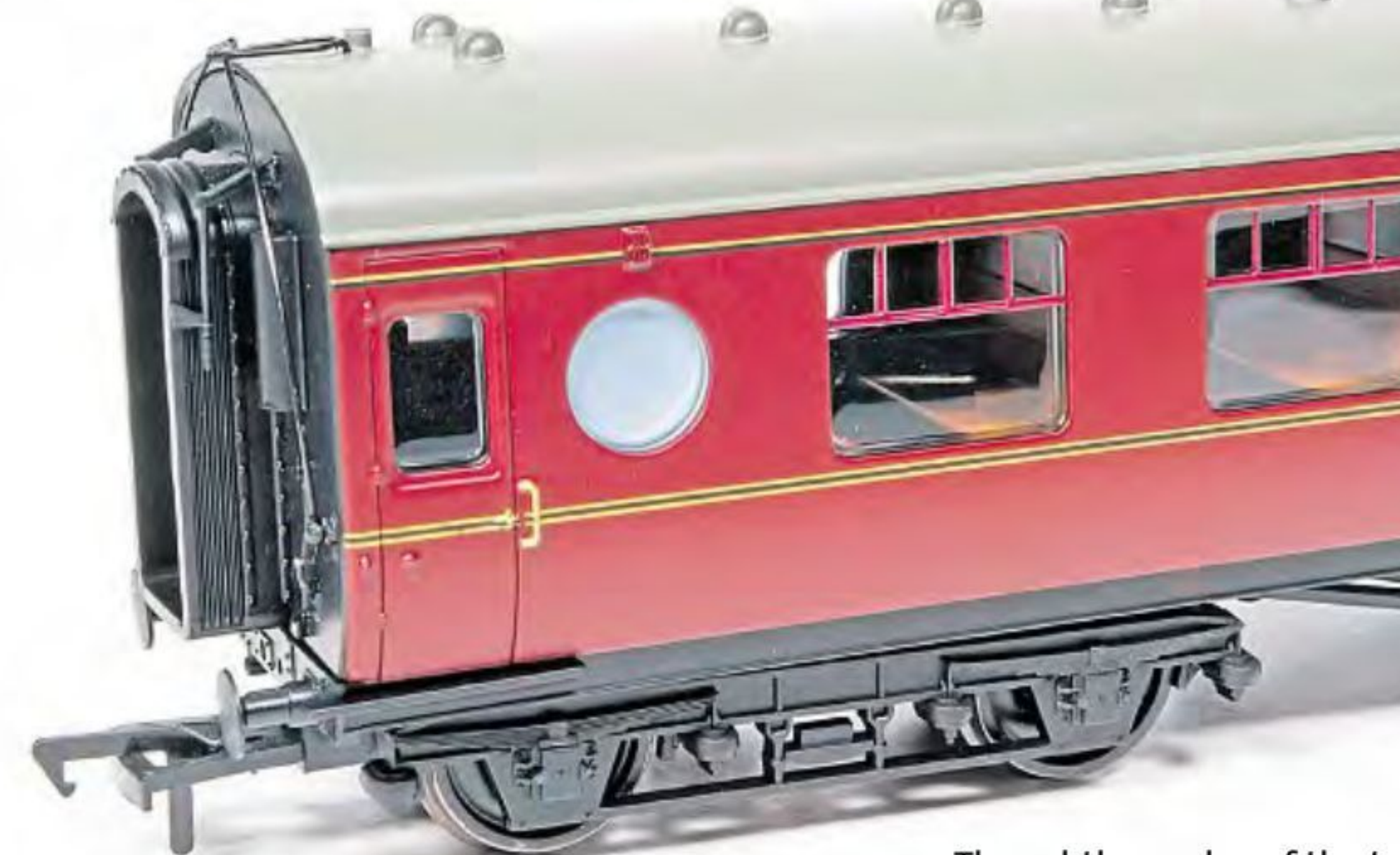
The subtle overlap of the top of the solebar is represented on the Corridor Composite coach.
