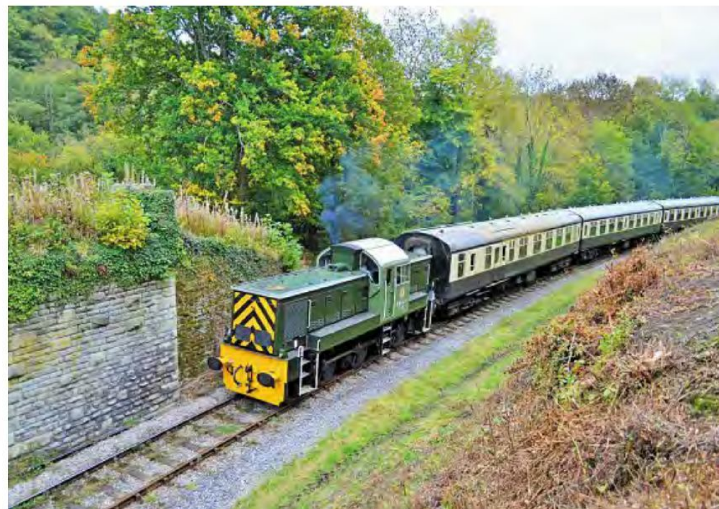
Class 14 0-6-0 diesel-hydraulic No. D9555 is seen at the DFR's Abutment with a train of BR Western Region carriages.
