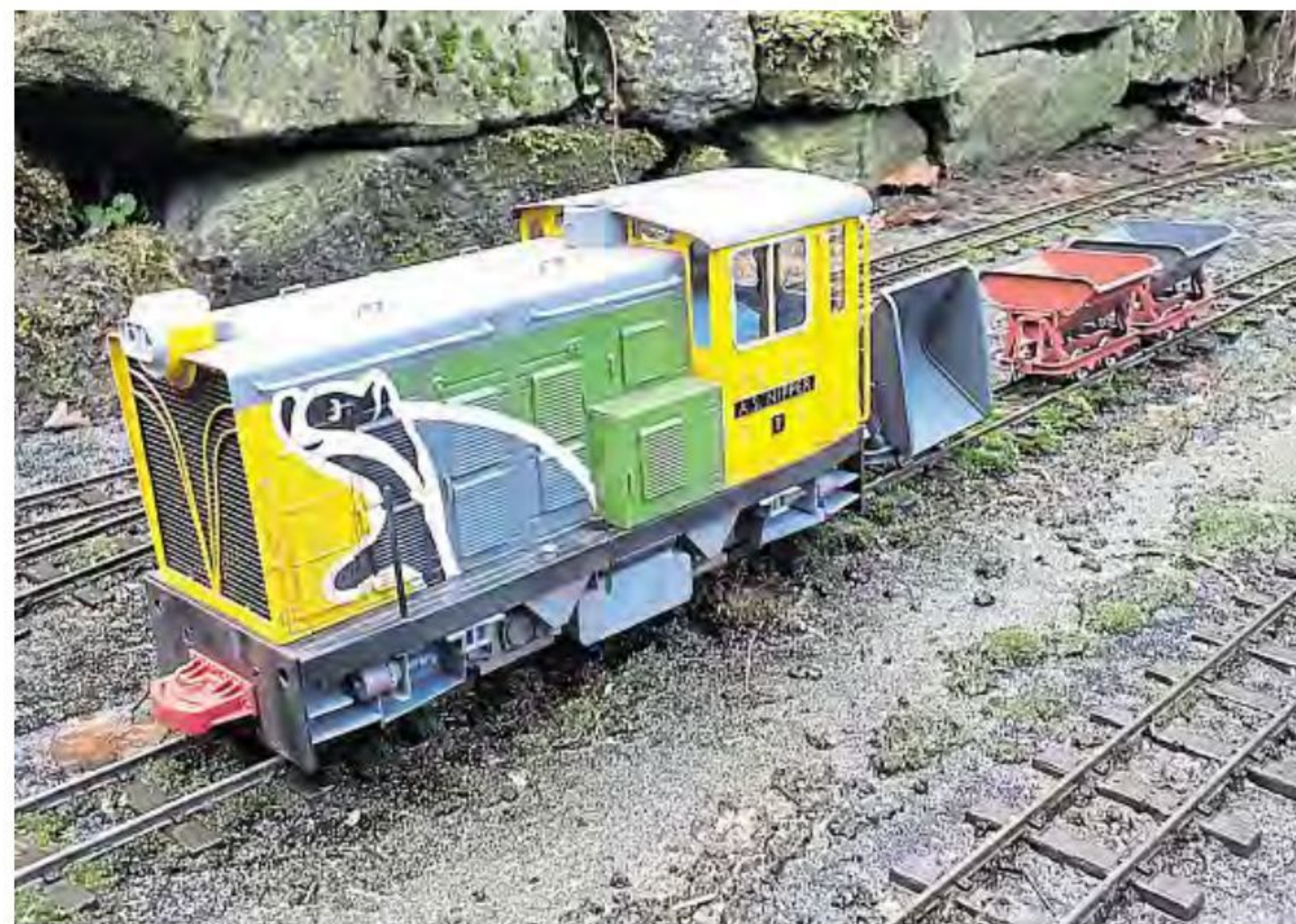
Battery-powered, radio-controlled and with a sound card, this customised Roundhouse NDM6 can be up and running in moments and is powerful enough for 'Thunderbird' duty rescuing broken-down steamers!
