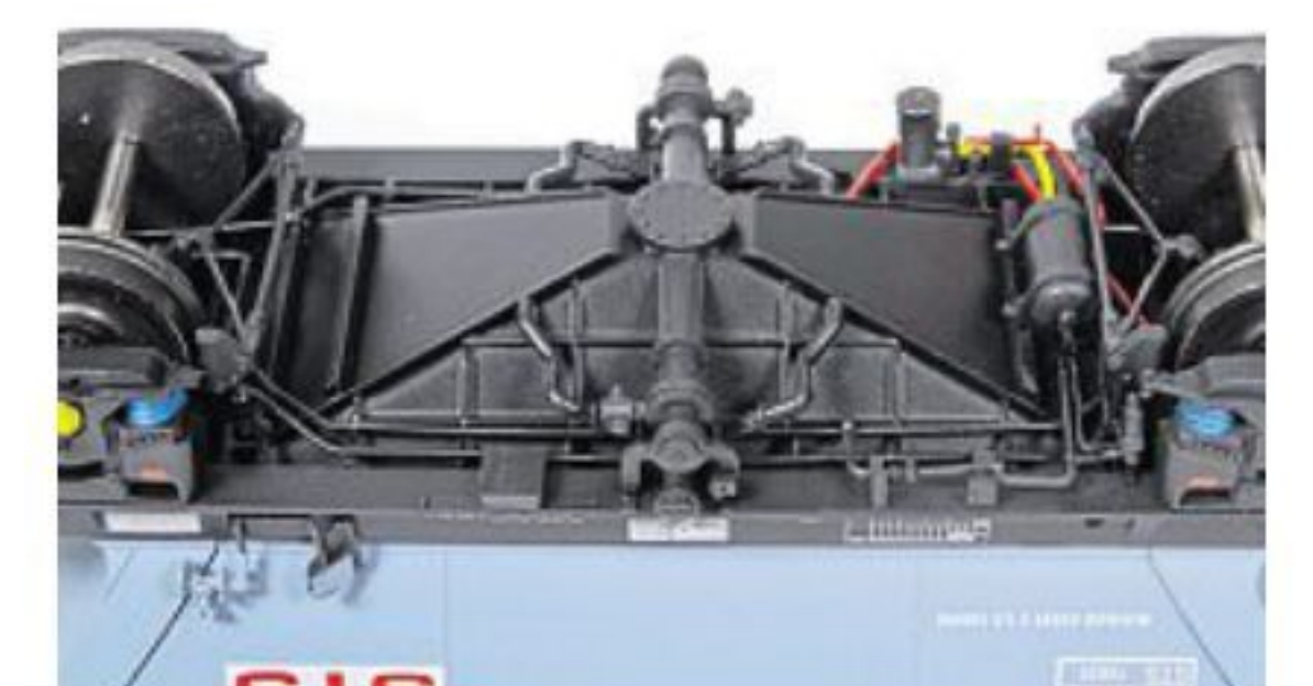
Note the pipe runs around the congested area of the discharge chute and around the brake equipment. It's not a particularly large wagon, so fitting this level of detail into such a confined area is particularly commendable.
