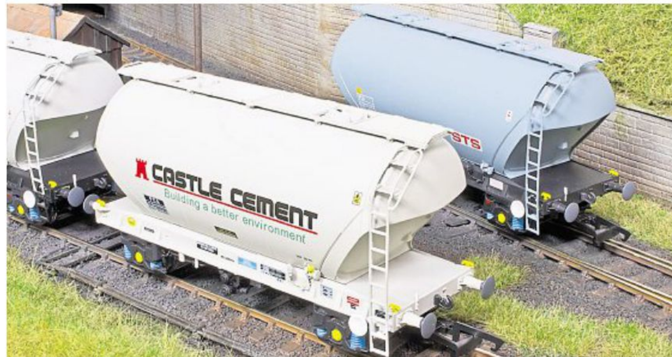
The character of the 1980s air-braked wagons is clearly seen in the models, including neatly modelled air-brake equipment, Gloucester suspension and Oleo buffers. More 1970s and 1980s wagon models of this quality are needed, and for a variety of different commodities too.
