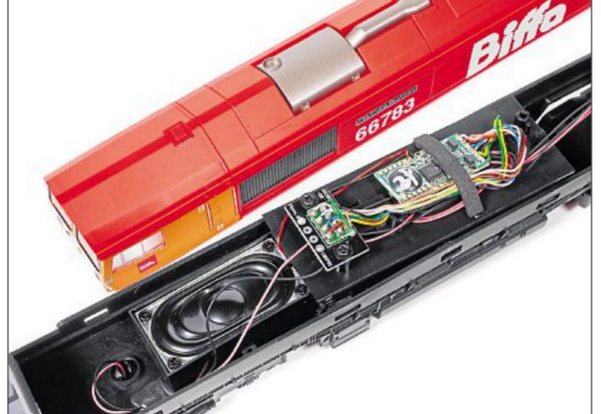
Hornby offers a DCC TTS decoder for its Class 66 model which fits in the large body shell with ease. The supplied speaker does not do the recordings justice, however.
