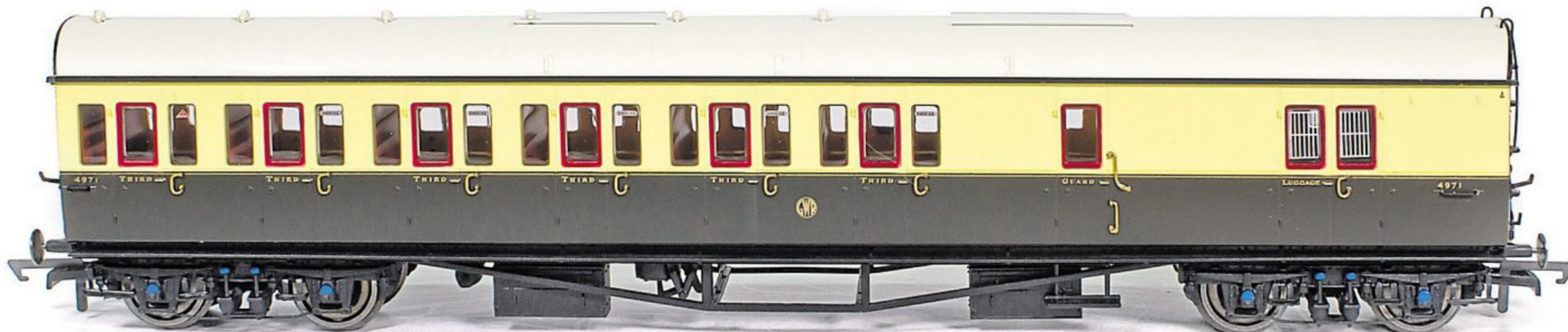
This is the model of Diagram D98 six compartment Brake Third coach No 4971.
