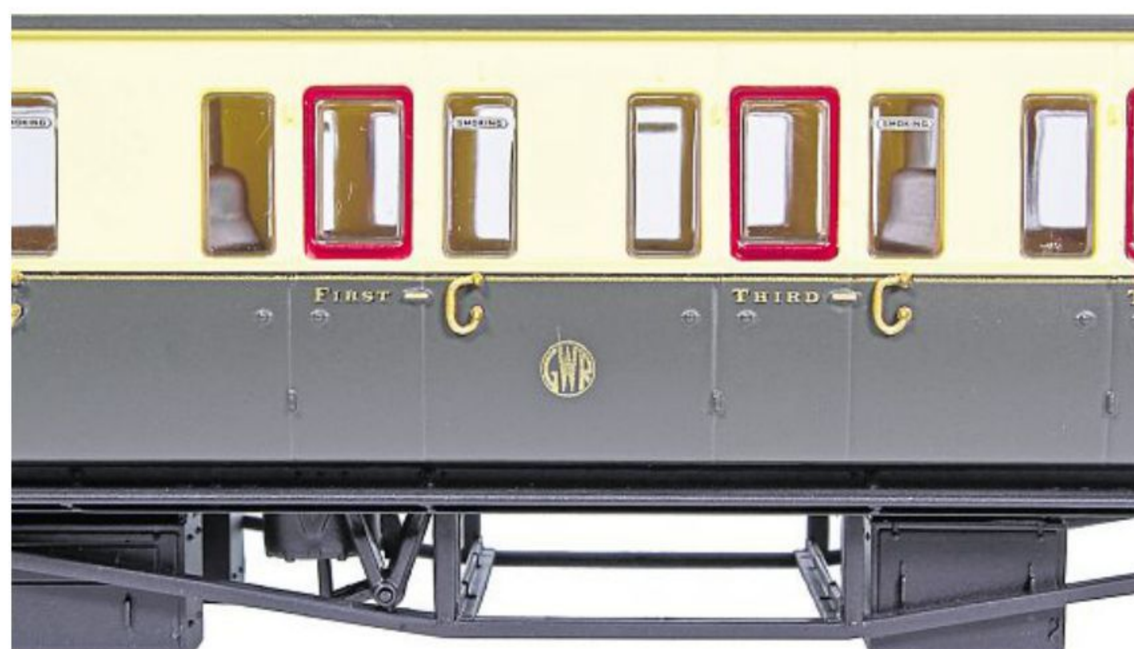
A close-up of the GWR motif, the separately applied plastic commode handles, flush glazing and door details.
