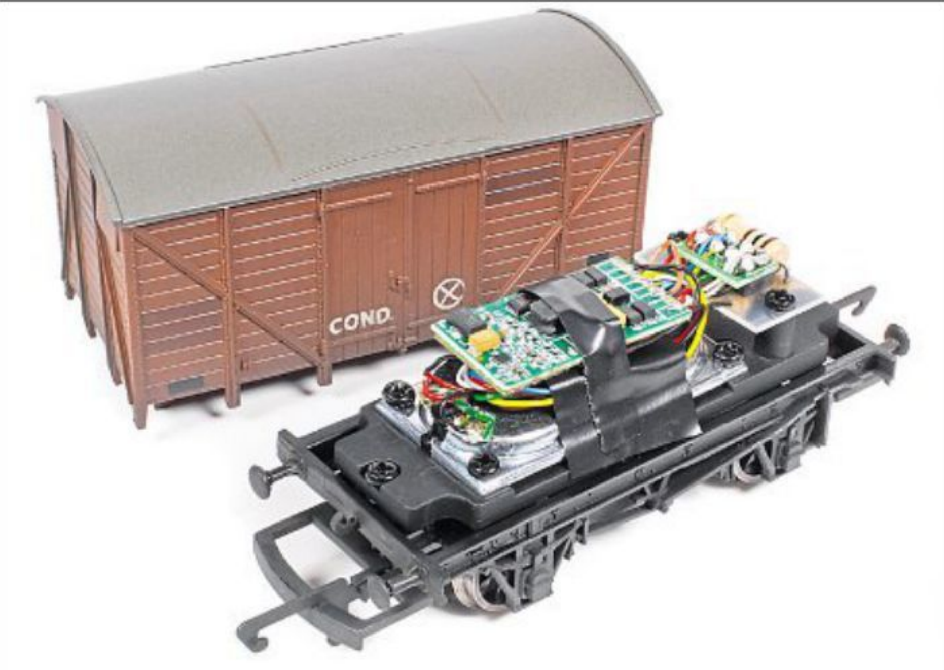
A neat idea from Hornby is the ambient sound wagon which has a DCC sound decoder fitted, together with a speaker set face-down in the underframe. It is loaded with controllable railway, atmospheric and street sounds.
