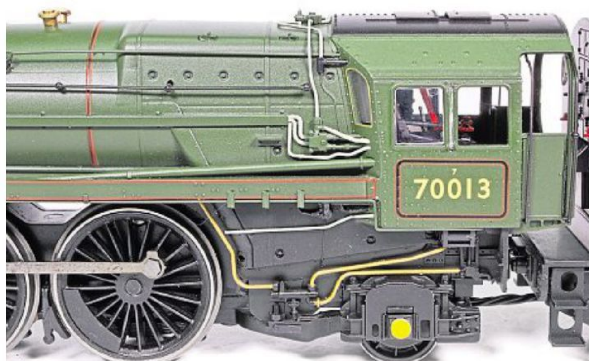
Detail applied around the cab, including separate pipe runs and flush glazing.
