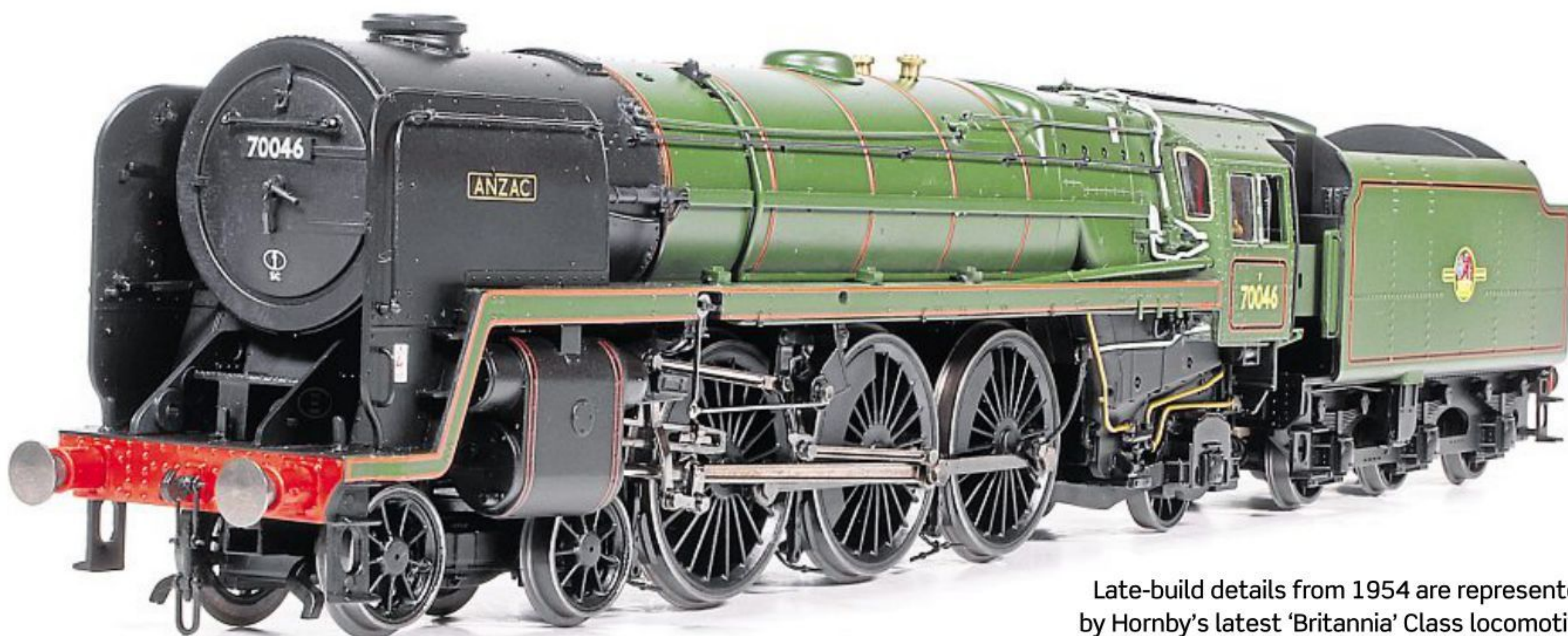
Hornby's modelling of the Walschaerts valve gear is neatly done, and it works with a smooth action that's best enjoyed at slow speed. Note the slight rusting effect applied to the con rod and coupling rod.
