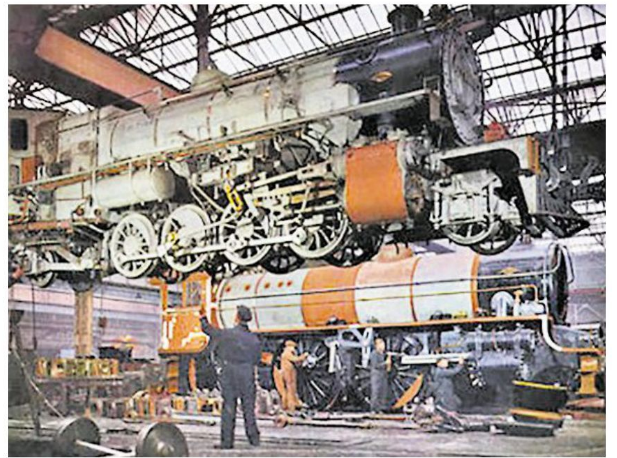
Two steam locomotives with very different destinations are seen under construction in the erecting shop at the North British Locomotive Company's Queen's Park Works in 1952. A Class 29 2-8-2 destined for East African Railways & Harbours is hoisted on a crane, and behind it a B1 4-6-0 is being built for British Railways.
