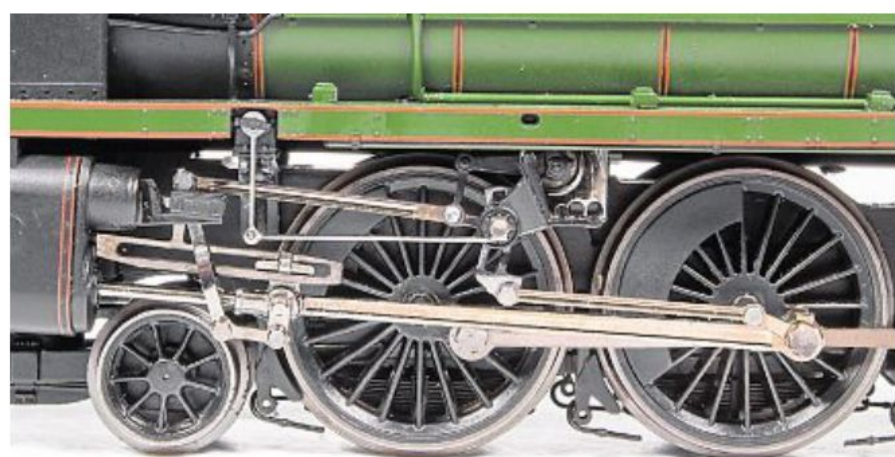
Hornby's modelling of the Walschaerts valve gear is neatly done, and it works with a smooth action that's best enjoyed at slow speed. Note the slight rusting effect applied to the con rod and coupling rod.
