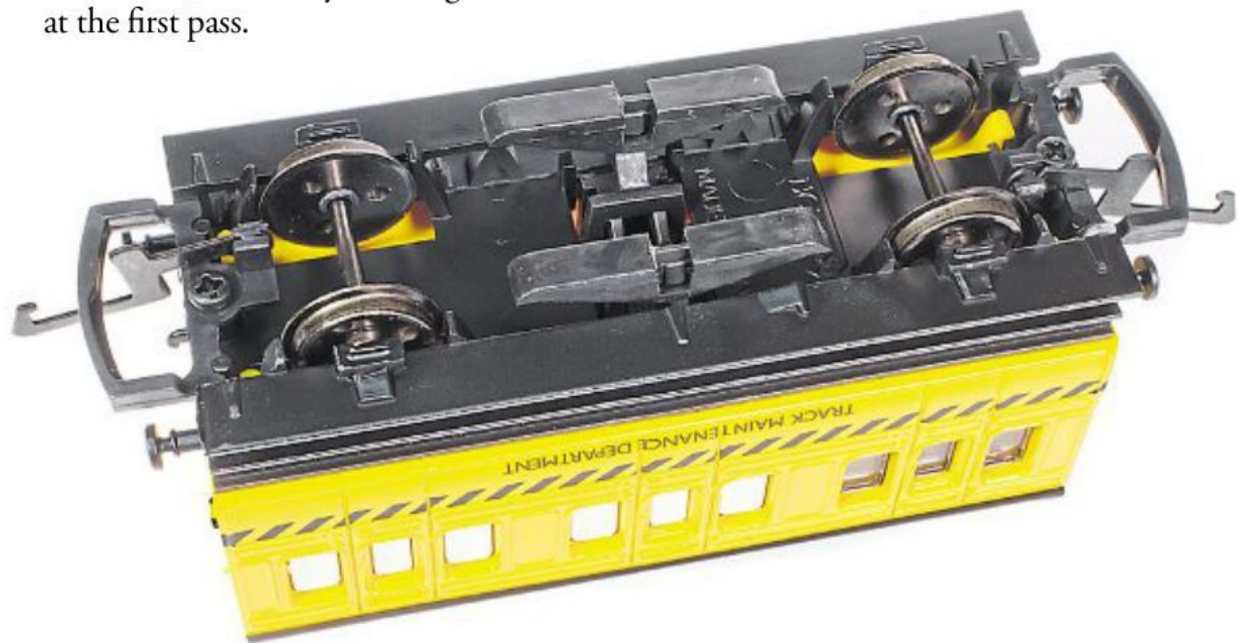
The cleaning mechanism consists of two pads fitted to sprung arms which apply gentle pressure on the rails. The cleaning action is through self-adhesive pads fitted to the bottom of the arms.
