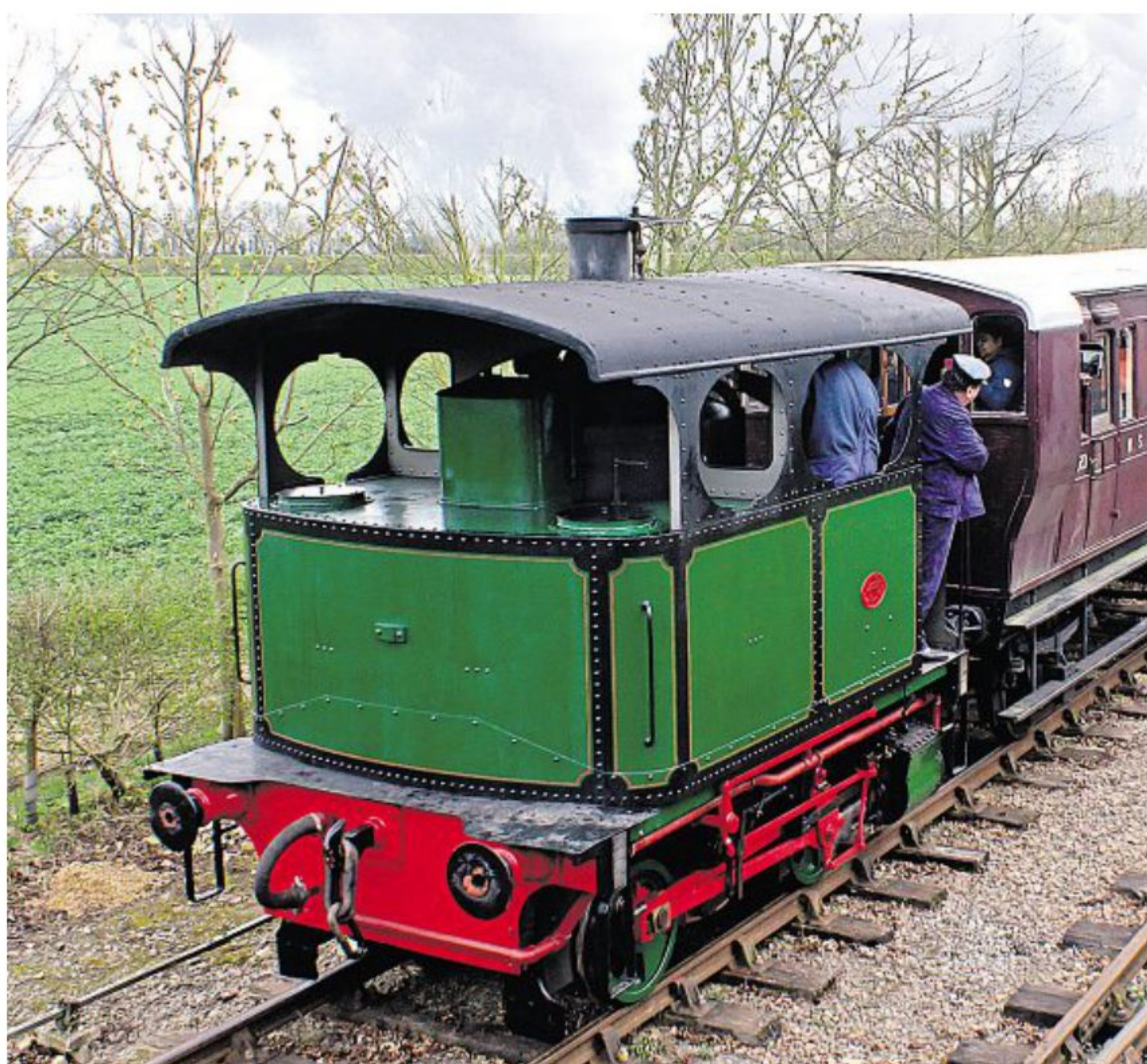
1906 Cockerill 0-4-0WT tram locomotive No. 2525 was built in Belgium for shunting and light tramway work, but looks very much at home on the 'Middy', where it can raise steam much more quickly than conventional steam locomotives.
