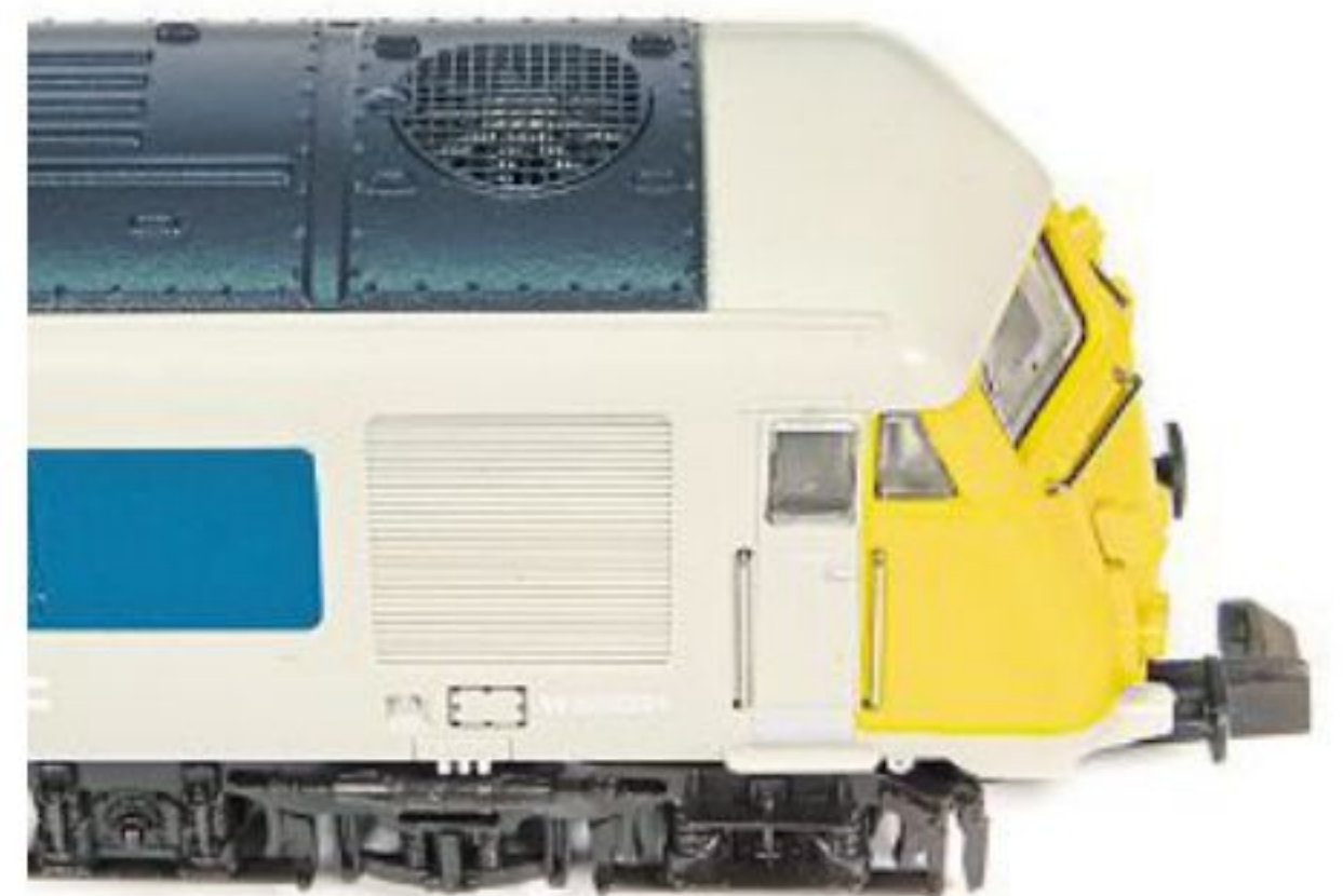
Roof details on the power cars include an etched metal cooling fan grille and fan detail.
