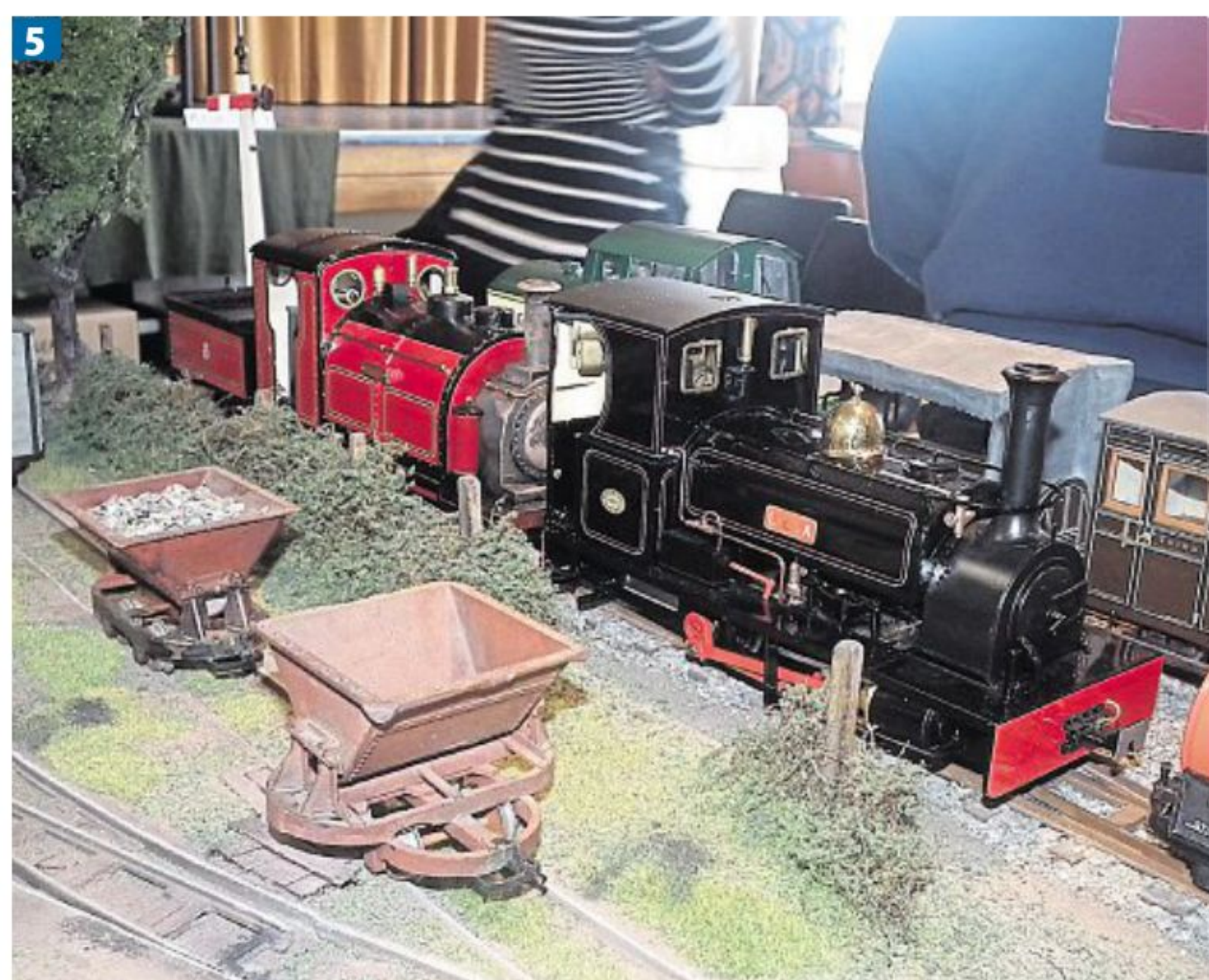
5. These two lovely saddle-tanks, which will be familiar to anyone who loves the Welsh narrow-gauge railways, were found on an SM32-scale layout called 'Ffuglen' at Altrincham, featuring battery-powered locomotives on O-gauge track. In the native tongue, ffuglen roughly translated means 'fiction'!
