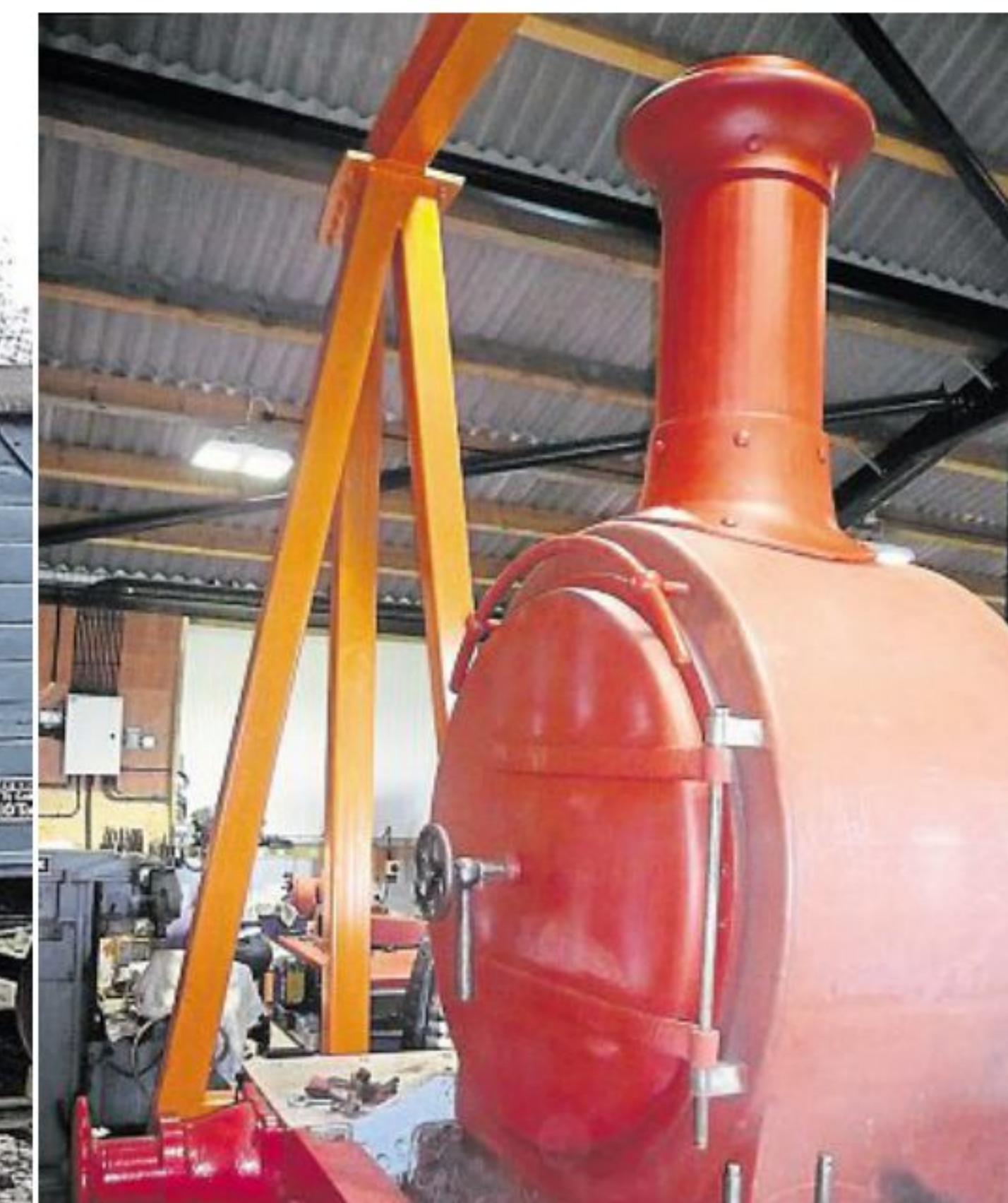
Under restoration in a lottery-funded shed is Hudswell Clarke 0-6-0T No. 1604, which already has a new chimney and smokebox.
