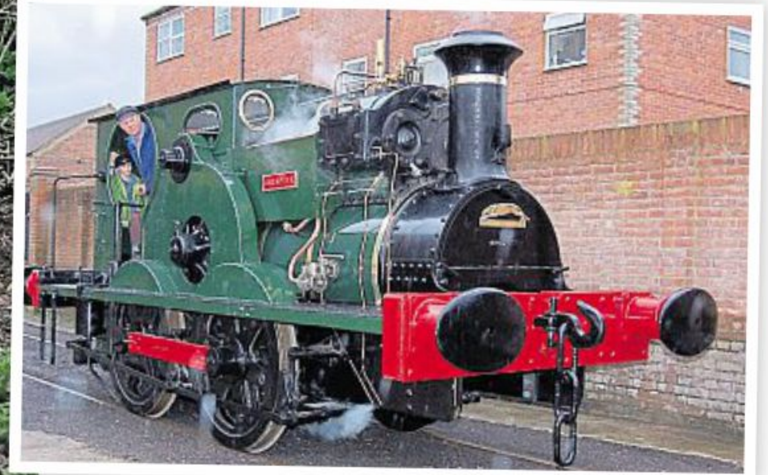
The Mid-Suffolk Light Railway's guest locomotive for this season is Sirapite , a 1906 Aveling & Porter 0-4-0WT that's really a traction engine on rails. It was the works shunter at Garrett's of Leiston for more than 30 years, and this will be its first working visit to another railway.
