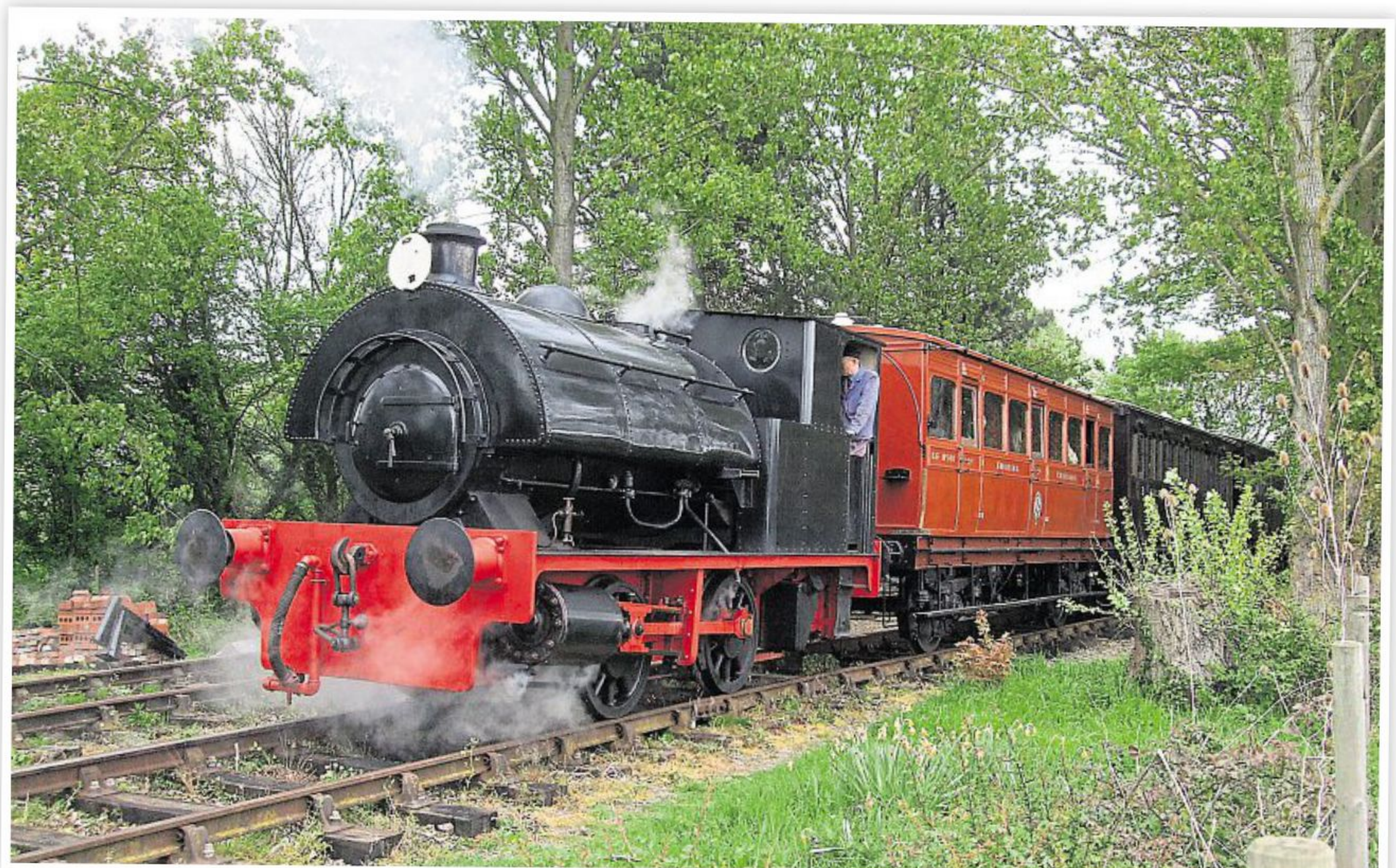
This classic Bagnall 0-4-0ST industrial shunting engine was built originally for the Central Electricity Generating Board in 1936, but has now been fitted with vacuum braking equipment and is a regular performer on passenger trains at the MSLR.
