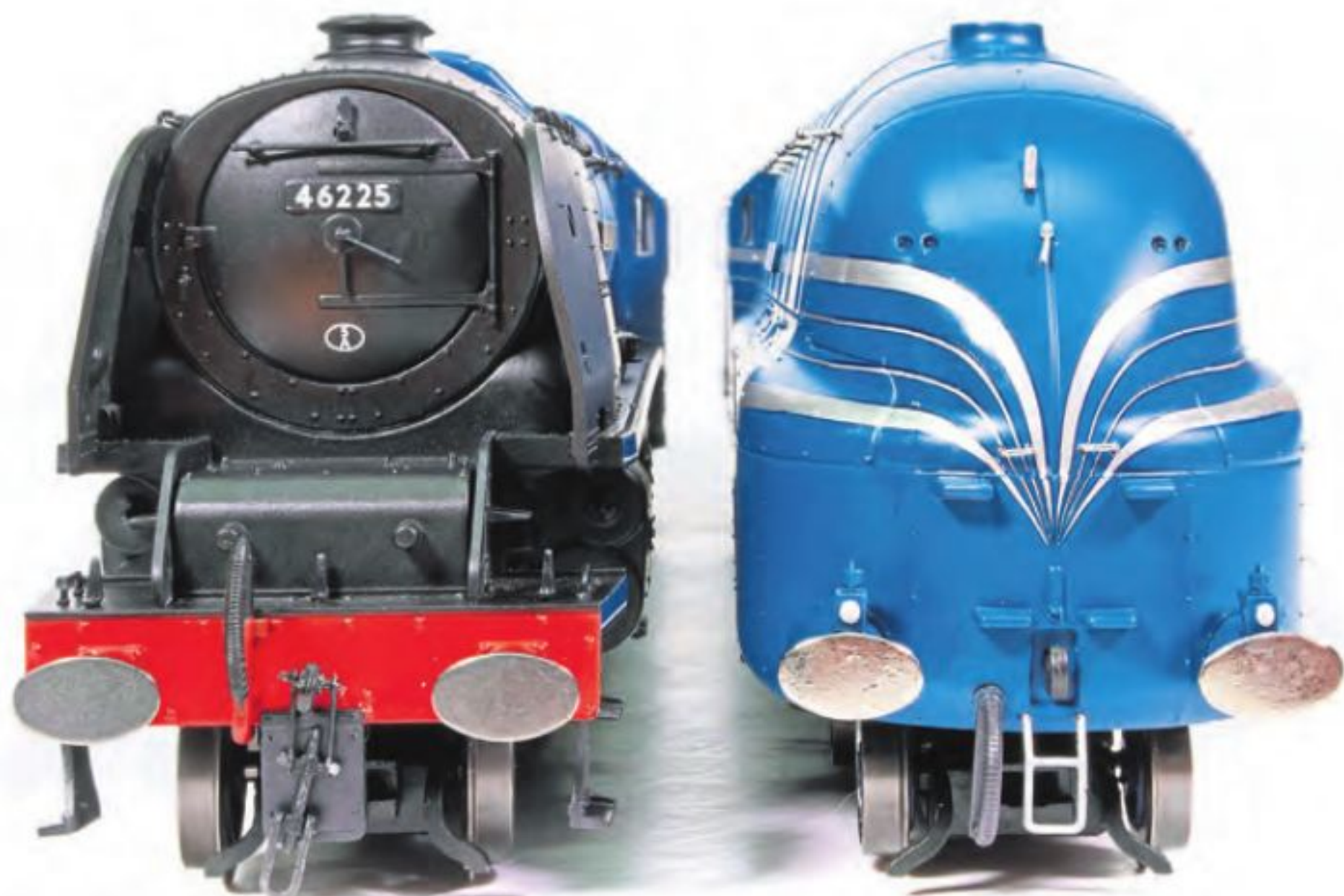
In this head-on detail shot of two versions of the class, note the taper to the top of the smokebox of the semi-streamlined version on the left - necessary to clear the casing when fitted with streamlining (right).
