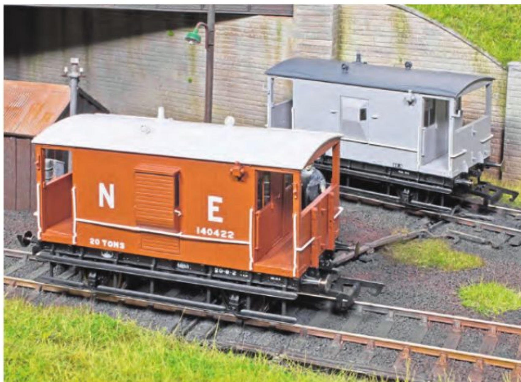
Detail differences between the two models include the buffer shanks, end bracing, side duckets, main body shell and side hand rails.
