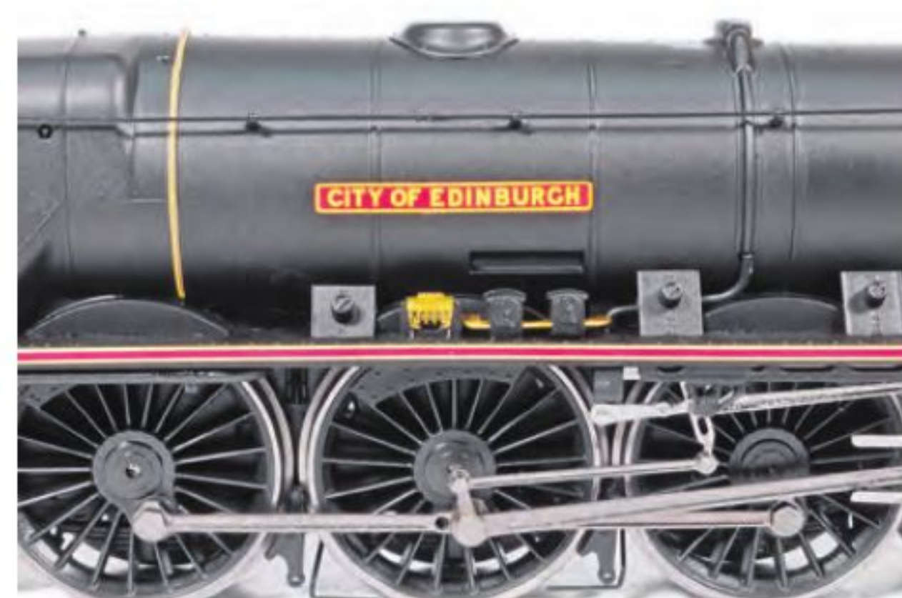
The chassis is detailed with sanding gear, brake blocks fitted in line with the wheels and driving wheels with fine spokes.
