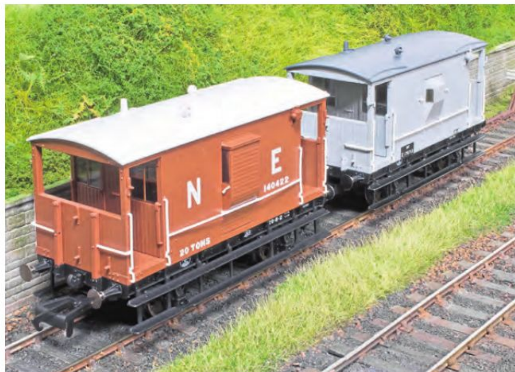
The same beautifully detailed underframe, with its fine spring and axle guard detail, is used on both models of the LNER 20t brake van.
