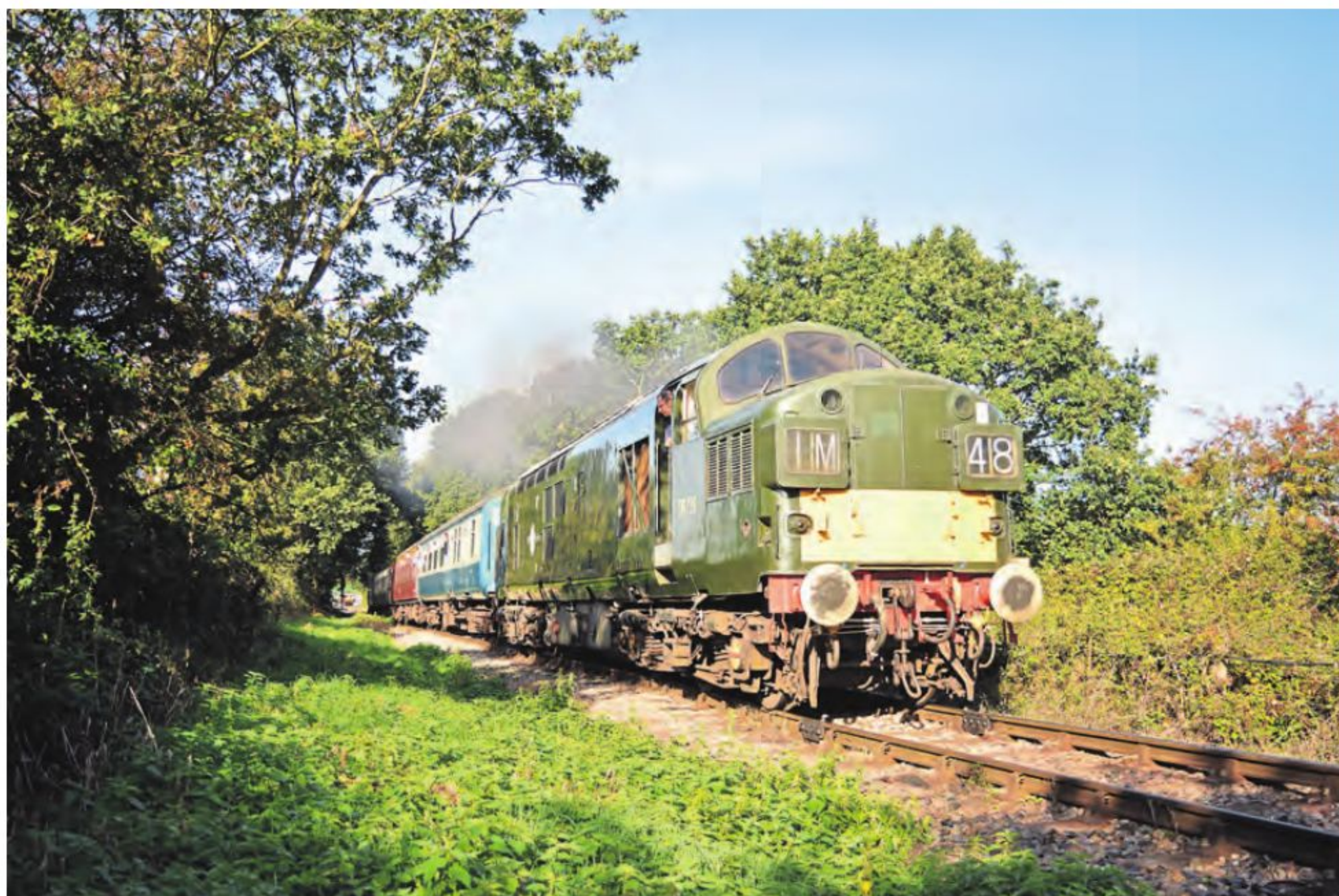
Locomotives like this beautifully-restored split-headcode English Electric Type 3 Co-Co diesel-electric No D6729 (class 37 No 37029) were once a familiar sight on former Great Eastern metals. It is seen powering through pleasant Essex countryside on the Epping Ongar Railway's Marconi gradient. PHOTO: OWEN HAYWARD.
