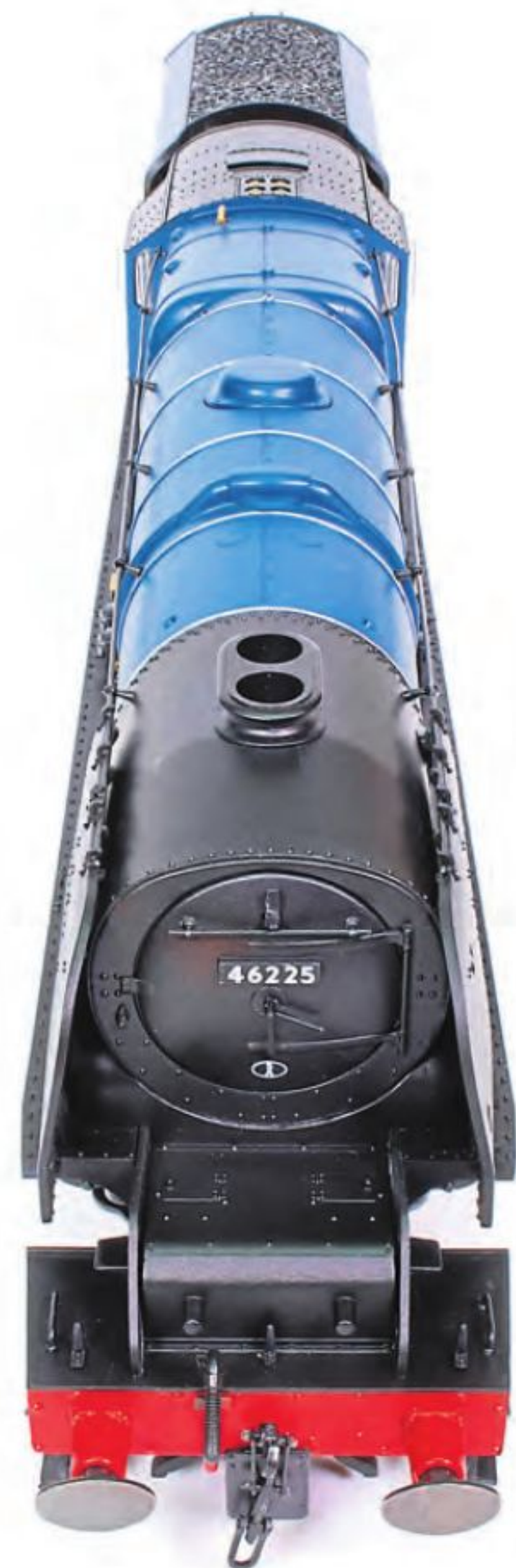
Smoke deflectors are fitted to both models and are of commendably thin section for plastic mouldings. Note the taper in the top of the smokebox.
