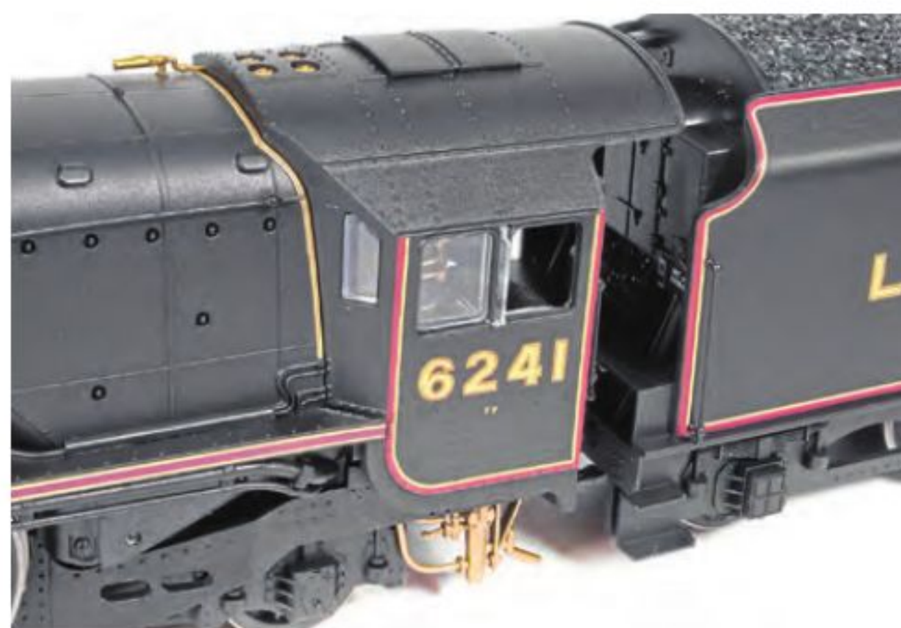
Flush glazing is fitted to the cab side and front windows.
