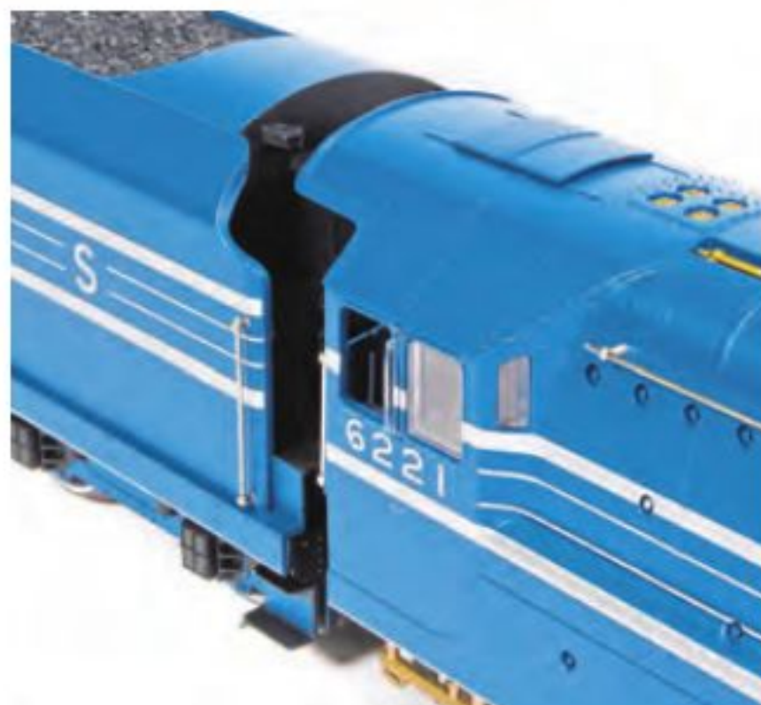
The cab roof includes whistle, cab roof ventilators and fine rivet detail.
