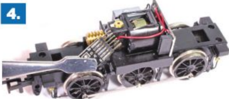
4. The analogue plug simply pulls out of the socket, and should then be popped in the model's box or other safe place.
