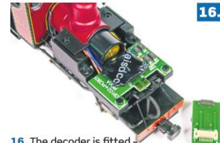
16. The decoder is fitted as simple as a conversion as one could hope for. Simply refit the body after testing the model on the service track to determine all is well with the installation.
