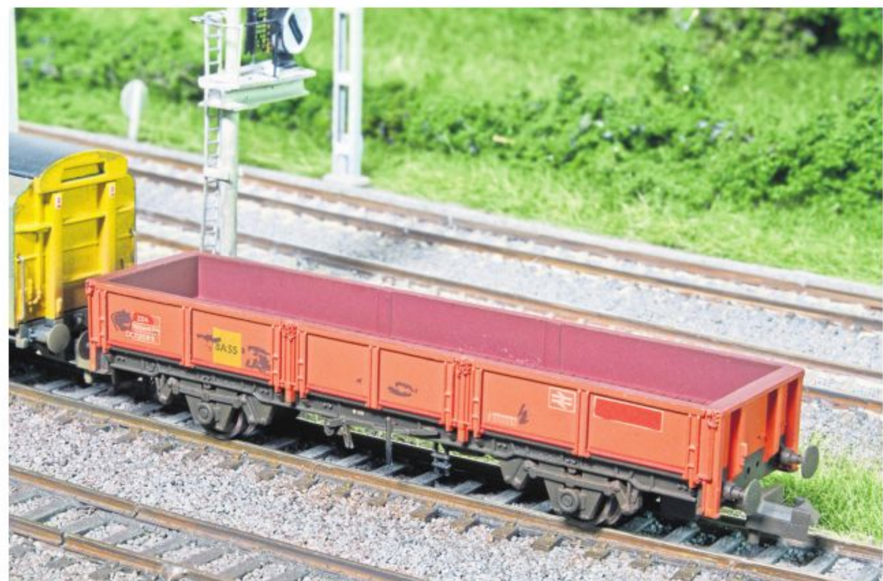
An air-braked OCA general merchandise wagon is included in recent releases both as an OCA in original BR Railfreight condition (not shown) and one in distressed condition with rust patching and faded colours as a ZDA 'Bass' engineers' wagon.
