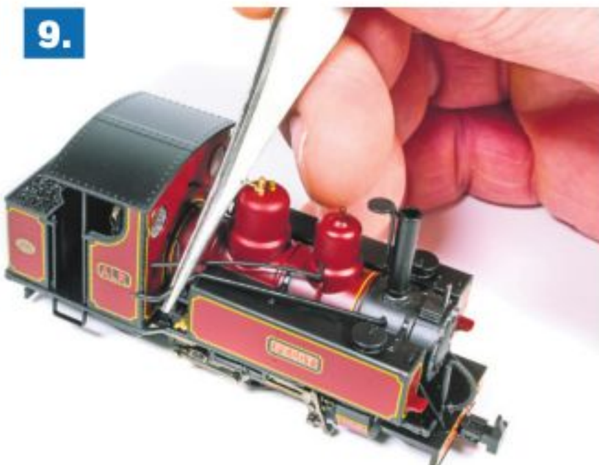
9. Several pipes linking the cab to the water tank moulding have to be released before dismantling the body.
