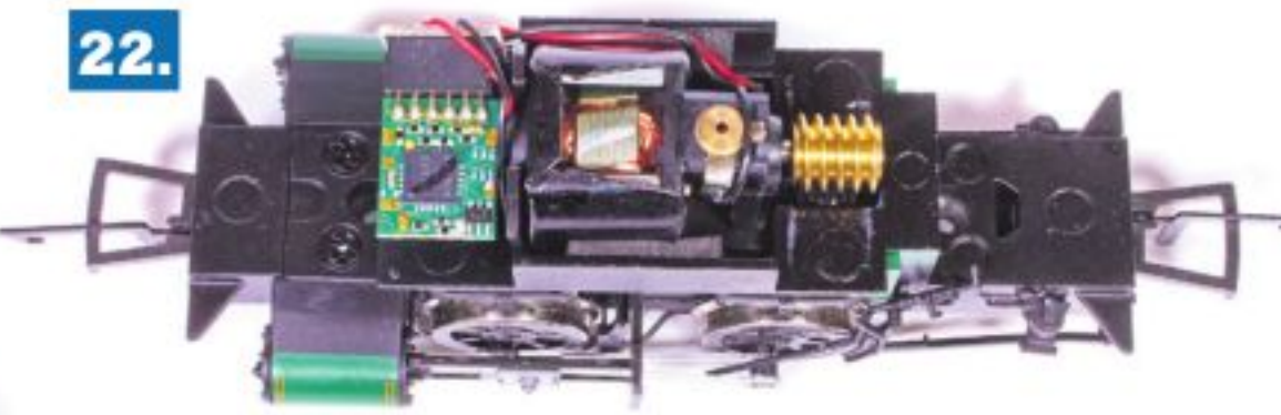
22. The completed conversion is shown with a Digitrax DZ126 decoder -- the perfect size for this model -- fitted. There are no metal parts for the decoder to touch, so no insulation tape was used to complete the installation.
