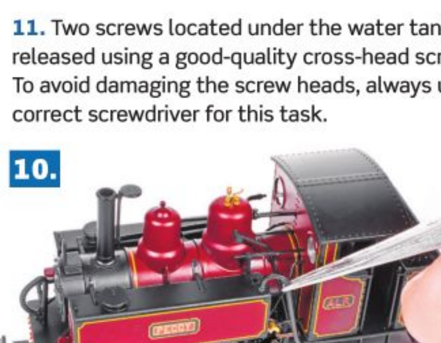
10. Pipework located on both sides of the model simply unclips with the assistance of a pair of tweezers.
