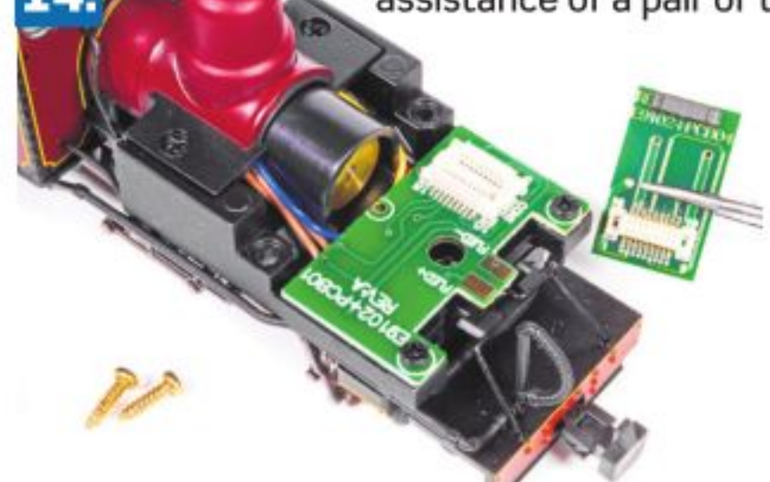
14. The analogue or dummy plug simply unclips from the socket.
