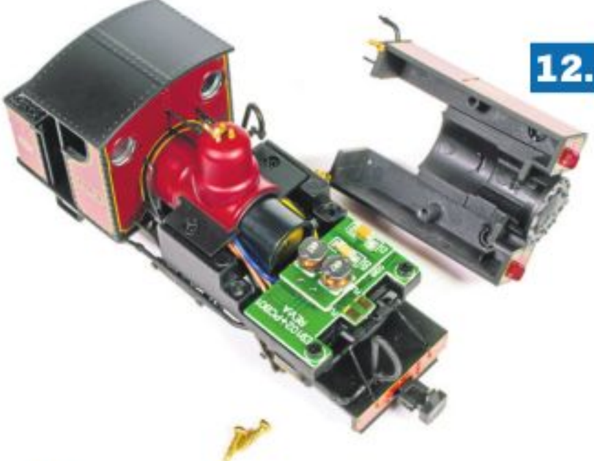
12. The side tank and smoke box moulding simply lifts off to reveal the circuit board.
