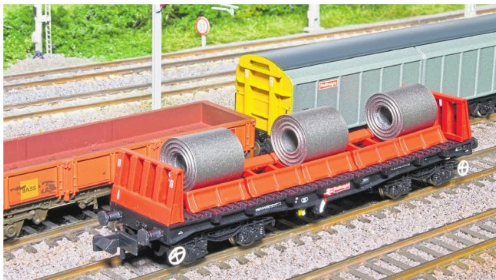
The BAA 100t steel carrier wagon was introduced in the 1970s and is offered as two models with cradles and loads in BR bauxite (not shown) and BR Railfreight red.
