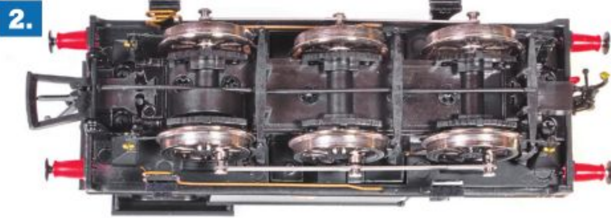
2. Four cross-head screws secure the body to the chassis. Drop them in a small tray or box to keep them safe.
