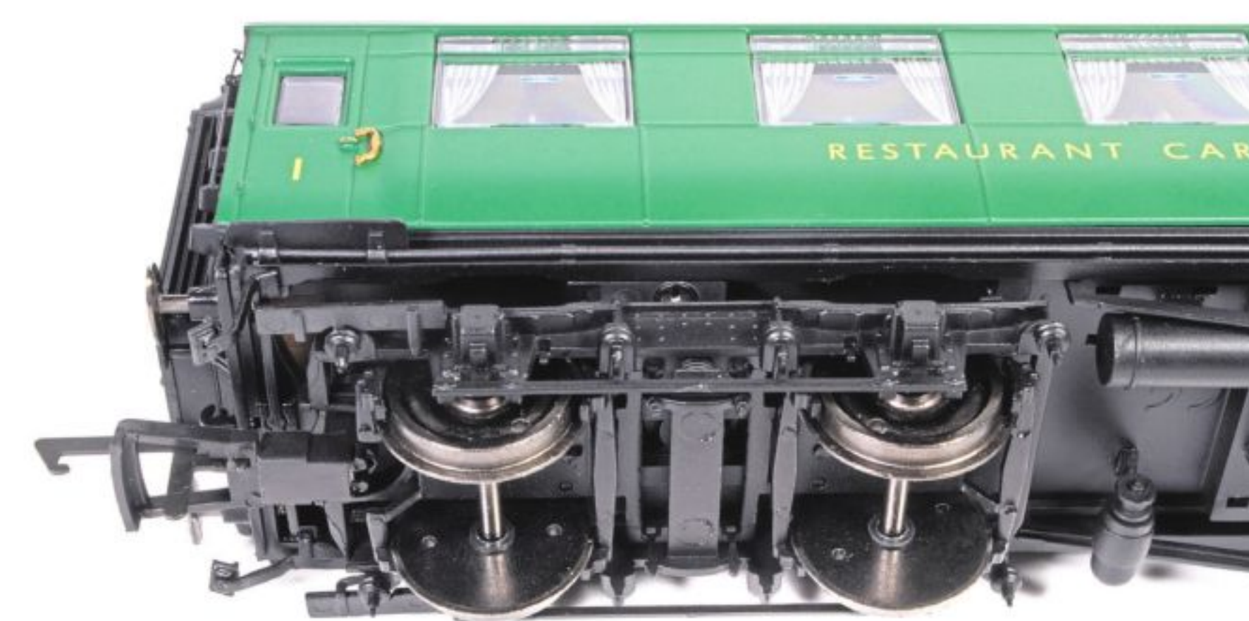
The coaches are equipped with excellent models of the SR 8ft bogies that are detailed with spring planks, brake shoes, brake linkages and footboards.
