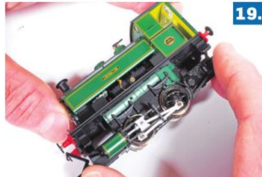
19. Ease the chassis out of the body after checking that pipework under the running plate doesn't snag.
