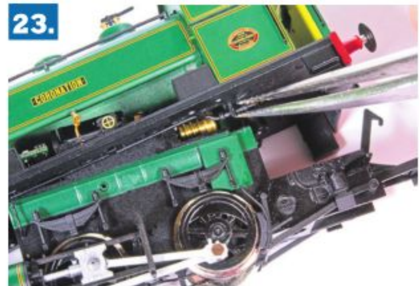
23. After testing the model, the body is put back using tweezers to ensure that the chassis pipework does not snag on the chassis, then the screws are refitted and the pipes plugged back into the side of the boiler.
