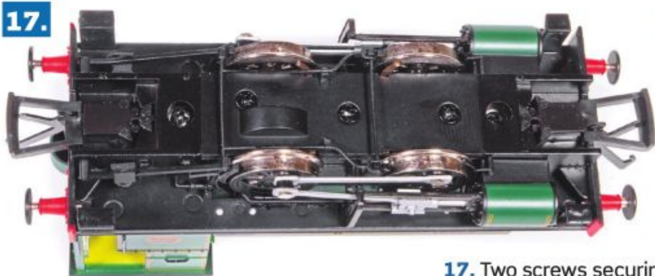
17. Two screws securing the body to the underframe are easily removed with a crosshead screwdriver, and one with a magnetic tip will be helpful for returning the screws when the conversion is complete.
