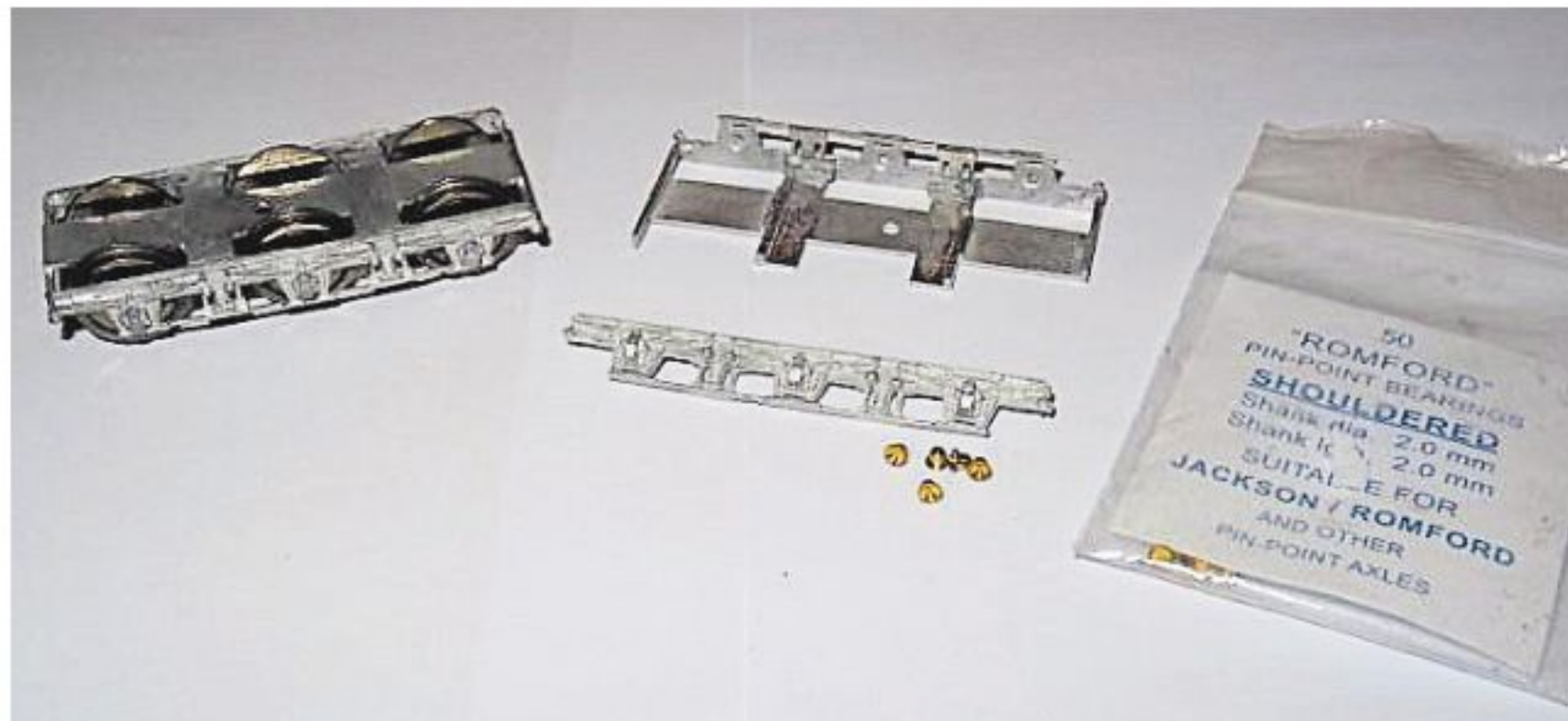
Left: An LNWR 11ft 6in six-wheel bogie (247 Developments #C612) are assembled with Romford bearings, and fitted with Bachmann 14mm wheels. Right: A bogie boss is installed with an M2 brass nut soldered on the underside.
