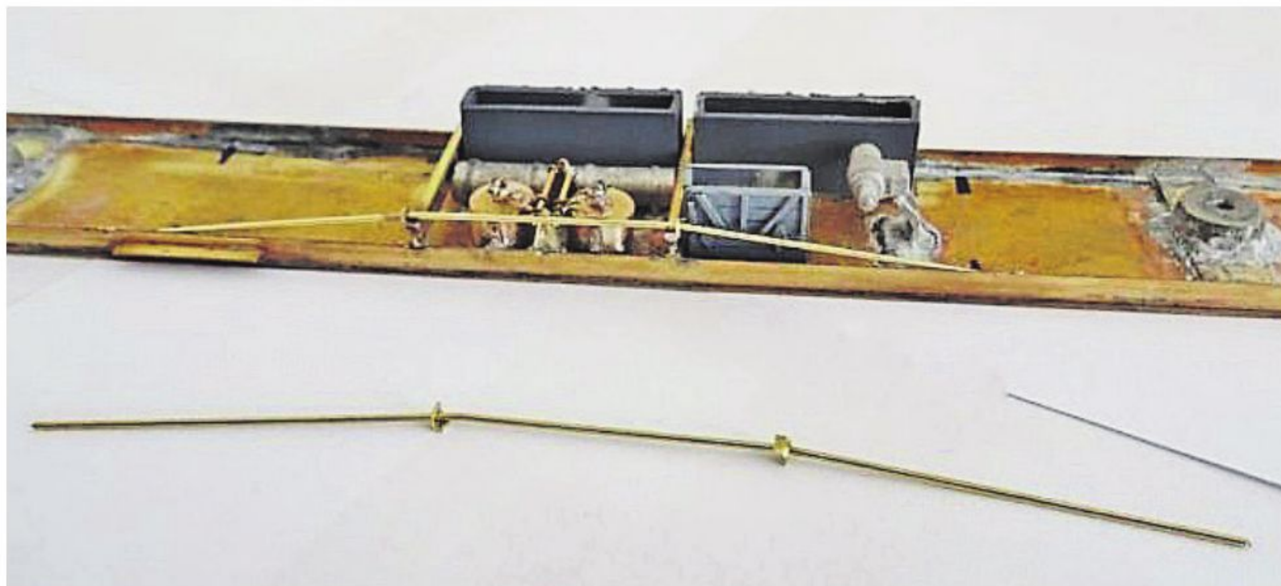
0.8mm brass rod was used to make the truss rods reinforcing the chassis.
