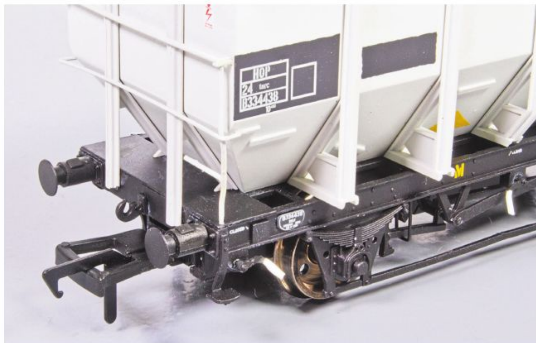
The ends of the hopper are detailed with accurately applied fine hand rails.
