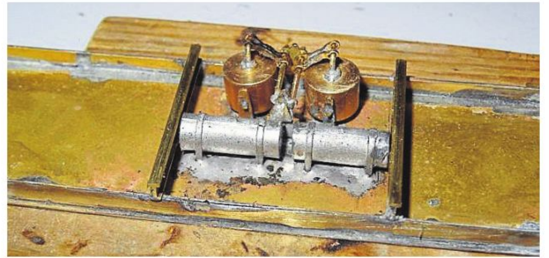
Left: K&S I-beams are soldered across the chassis. Right: Markits vacuum cylinders with a scratch-built assembly and seen with two white metal Dart/MJT castings.
