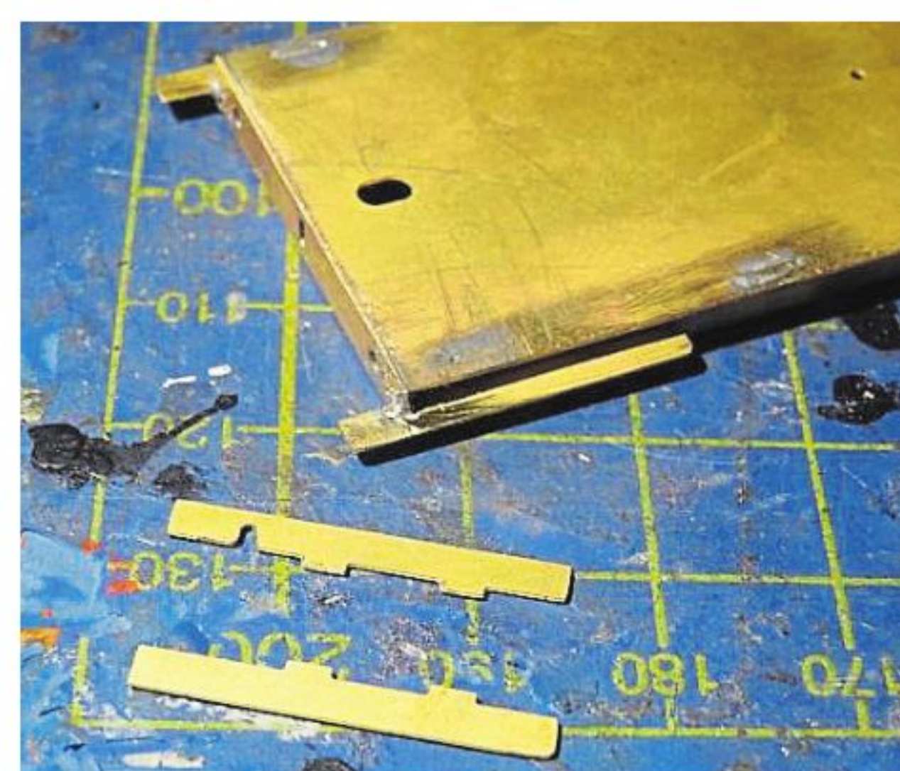
Cleaning a chosen area of brass with a glass-fibre pen before soldering will ensure a good join.
