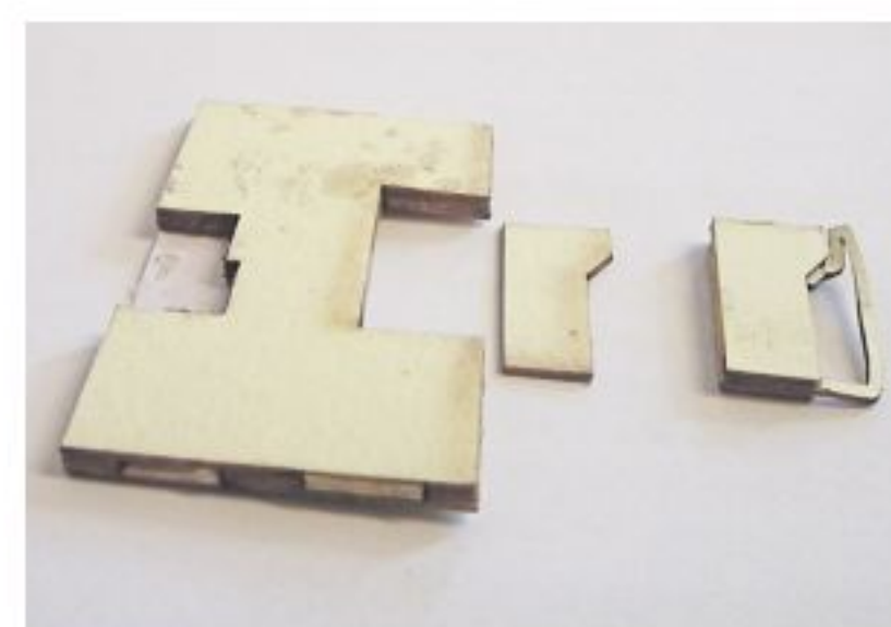
The laser-cut petrol pumps are so small they have to be assembled in a special jig that you also have to make up from laser-cut components. The different cut-outs on each side suit the type of pump chosen.
