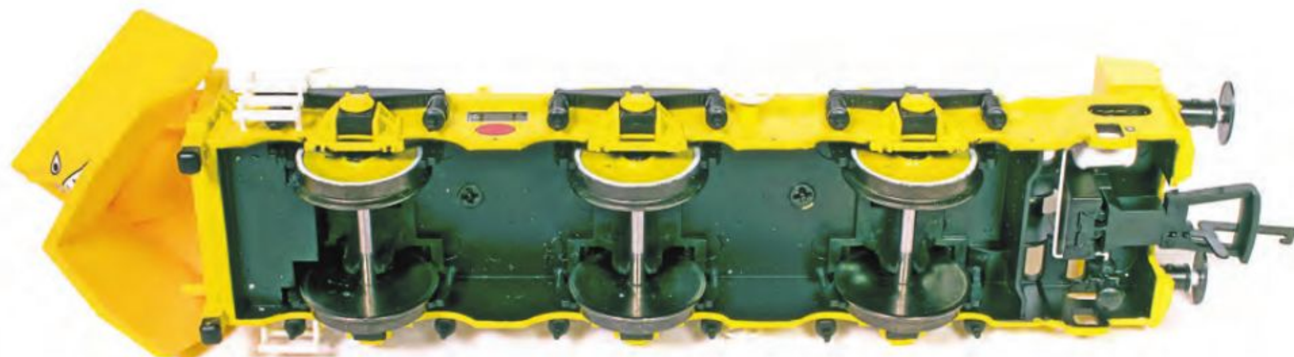
Metal wheels are fitted to the underframe running in inside bearings to allow the model to be propelled through sharp curves and complex junctions.
