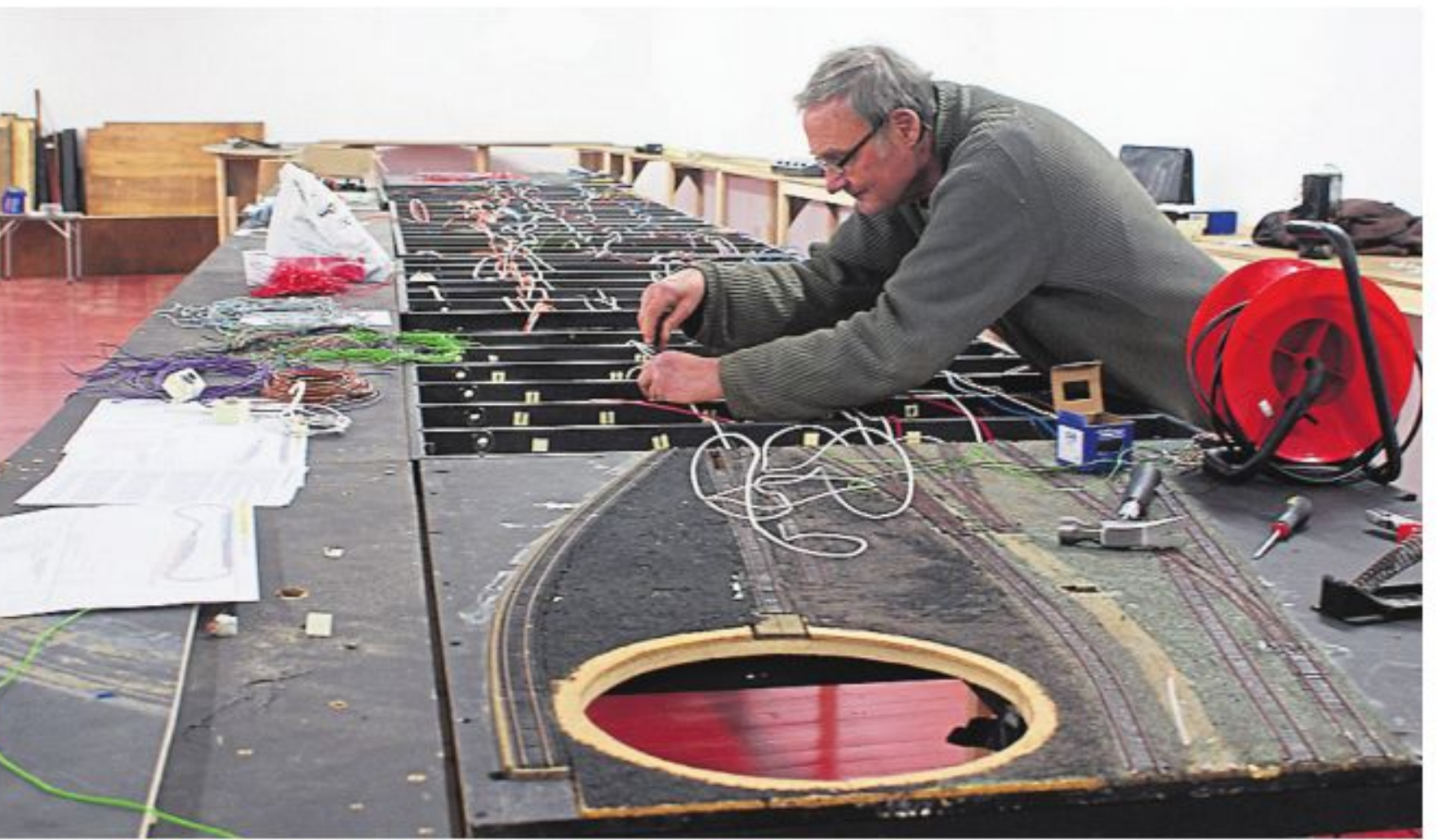
In the brightly lit, newly refurbished building in late 2013, trustee Peter Swift concentrates on rewiring the Chinley model railway to ensure traction continuity. The layout is worked on straight 12v DC supplied by Morley Vortrak controllers. Points are changed through probe-and-stud contacts on the control panel map. The members wanted it to be simple, so that there would be less to go wrong!
