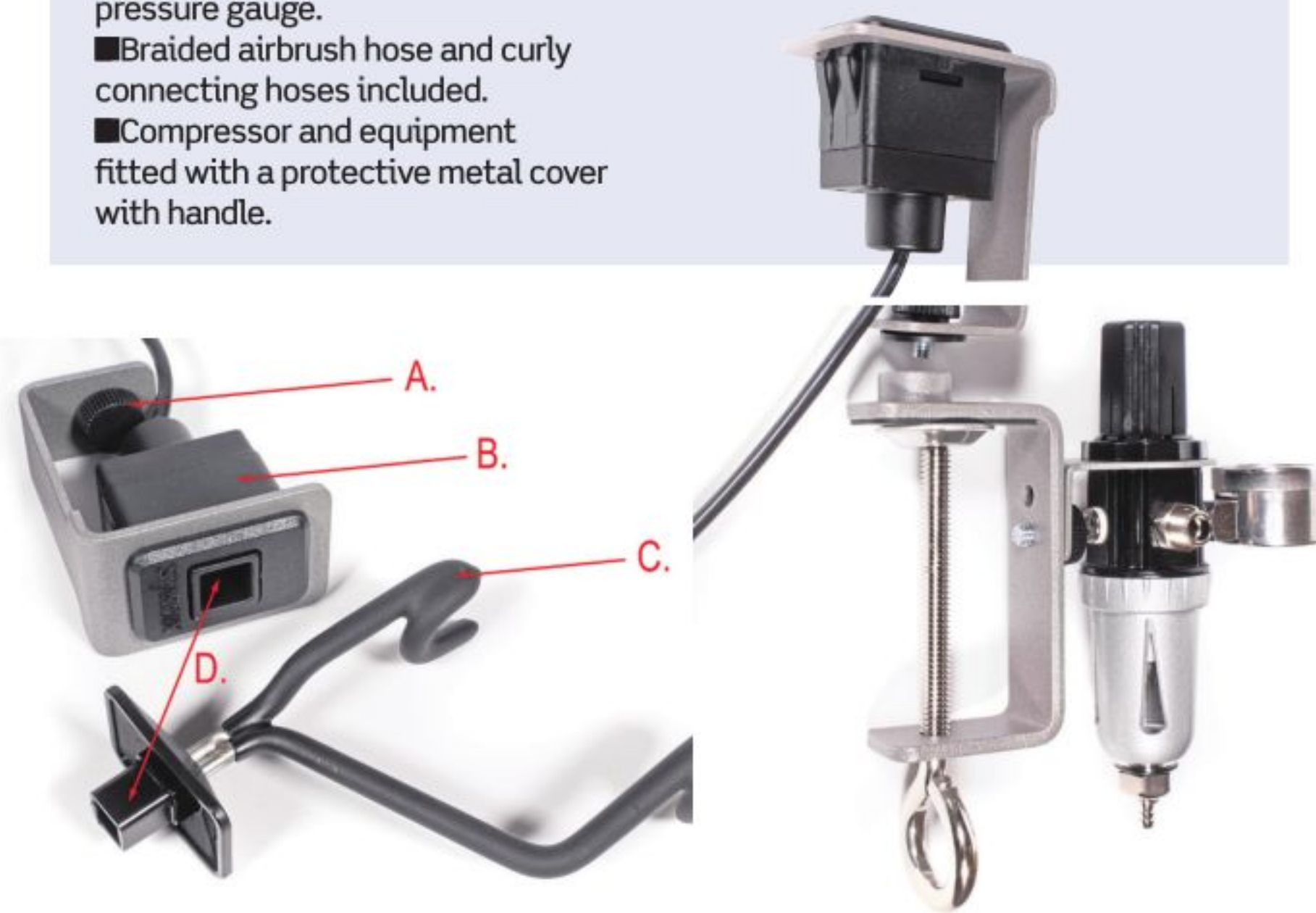
The 'Smart-Stop' assembly consisting of an airbrush hanger (C) and rocker switch box (B). It is attached to the air regulator clamp (A) and the airbrush stand plugs into the switch box (D).
