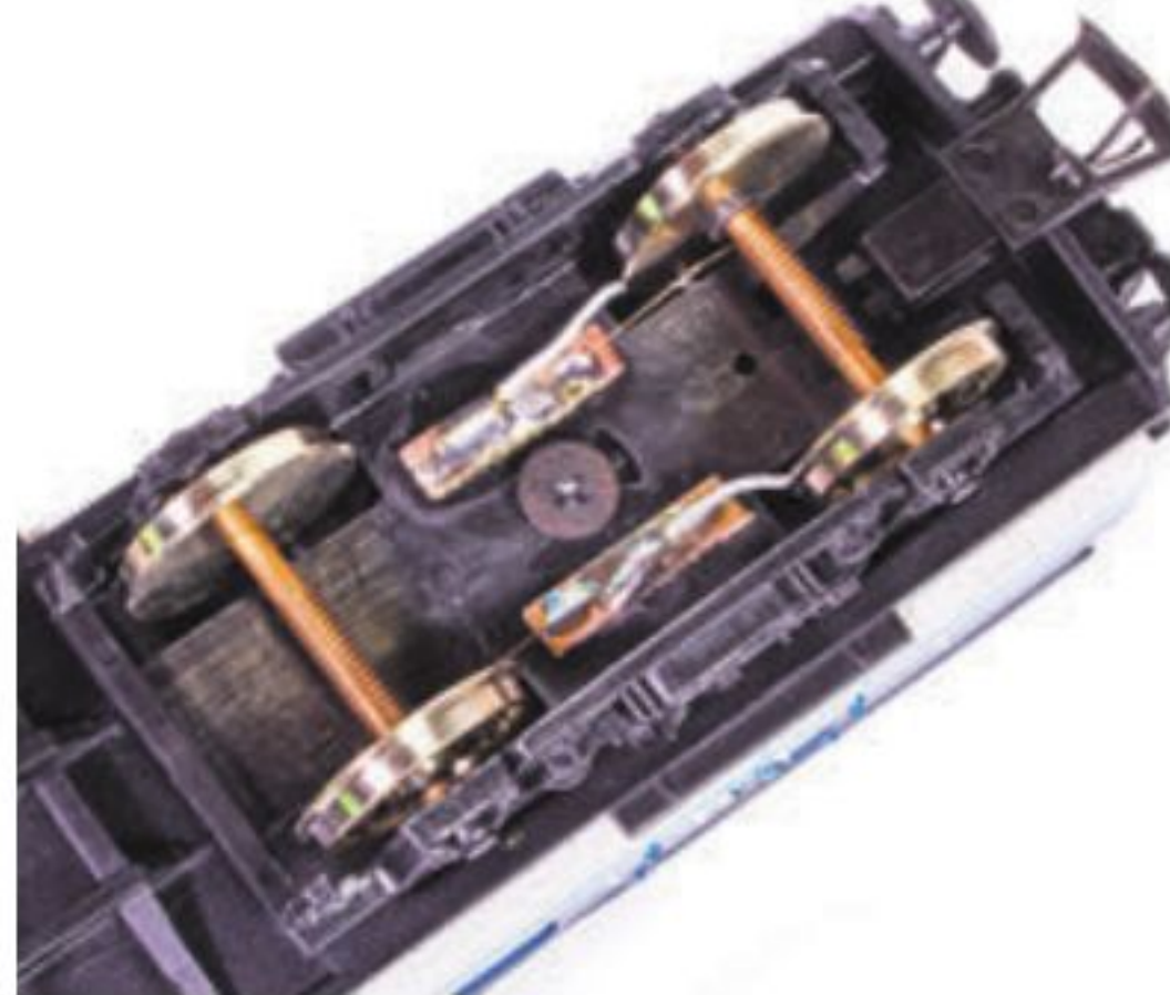
The DCC Concepts wheels and low friction pick-ups as fitted to the demonstration coach. Note that only one wheel axle collects current with this system, so it is good practice to use them on both bogies of the coach, with linking wires installed in the interior of the coach.
