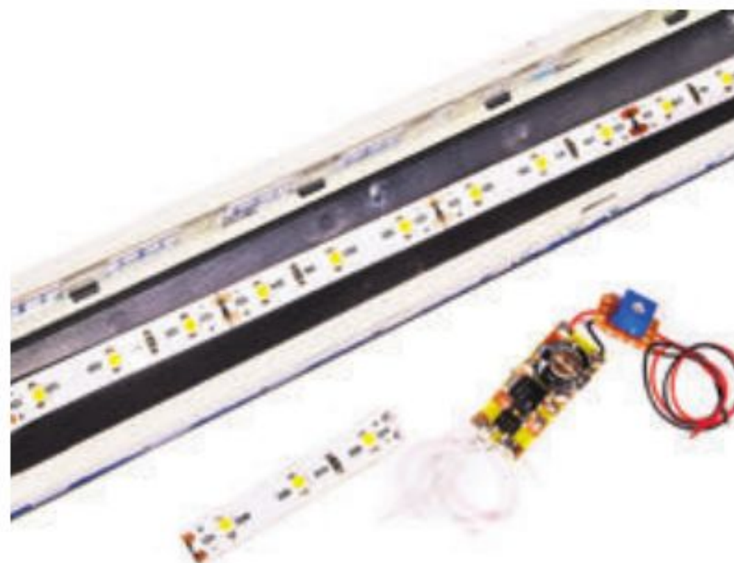
Test-fitting the trimmed lighting strip to the model, taking care to position LEDs in compartments of the BSK coach.
