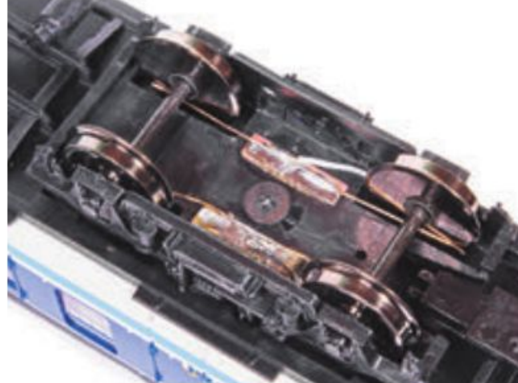
The circuit with track power is completed through wiper current collection pick-ups fitted to the bogie. When using the original Bachmann wheels, give them a thorough clean!
