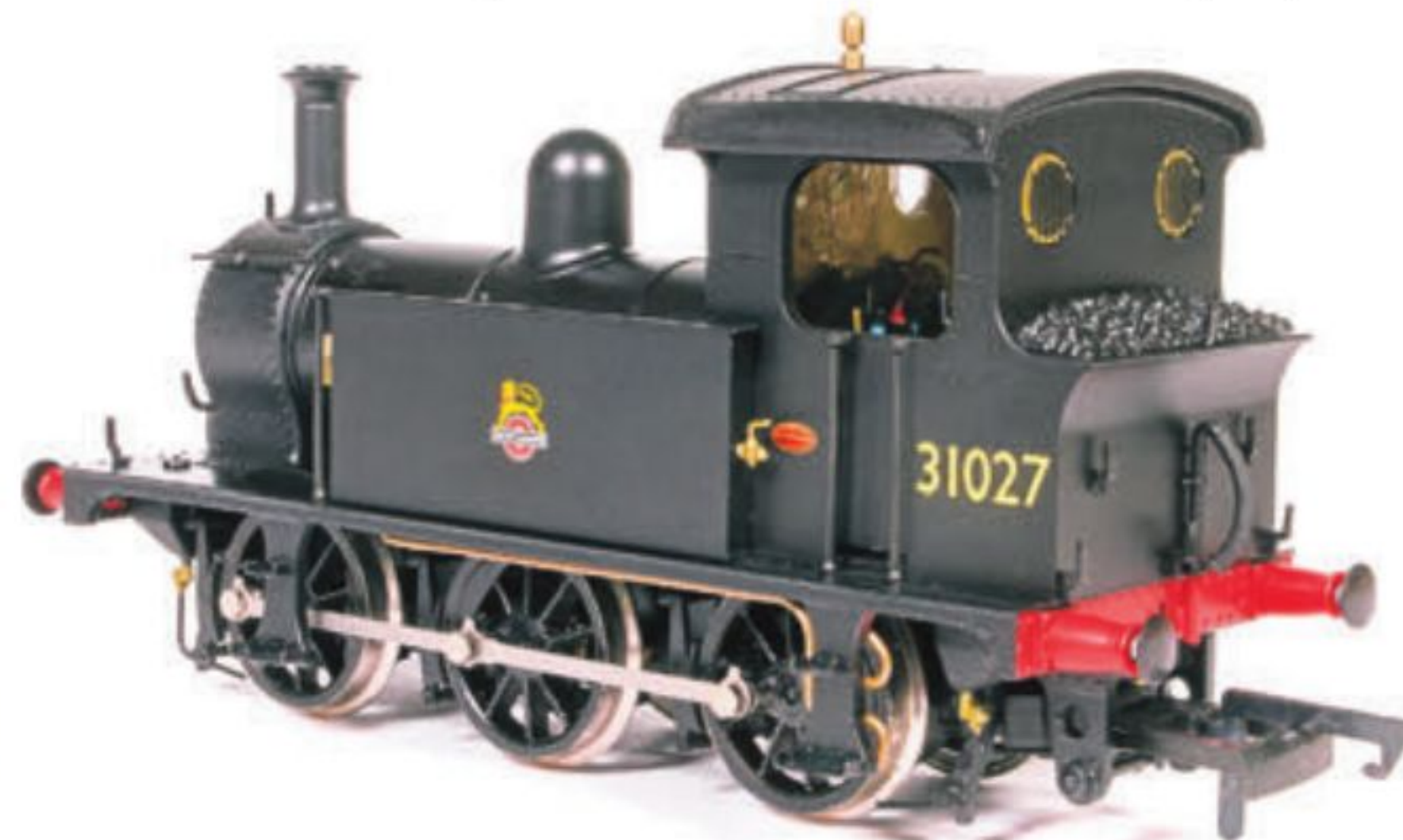
Toolings have been designed to allow locomotive specific details to be incorporated in individual models, including cabs and the guards on the rear cab windows.
