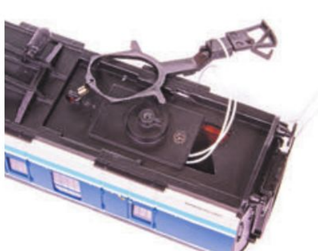
Having installed the kit, the coach is reassembled, with the power leads being fed through the close coupling cam opening to reach the bogies.
