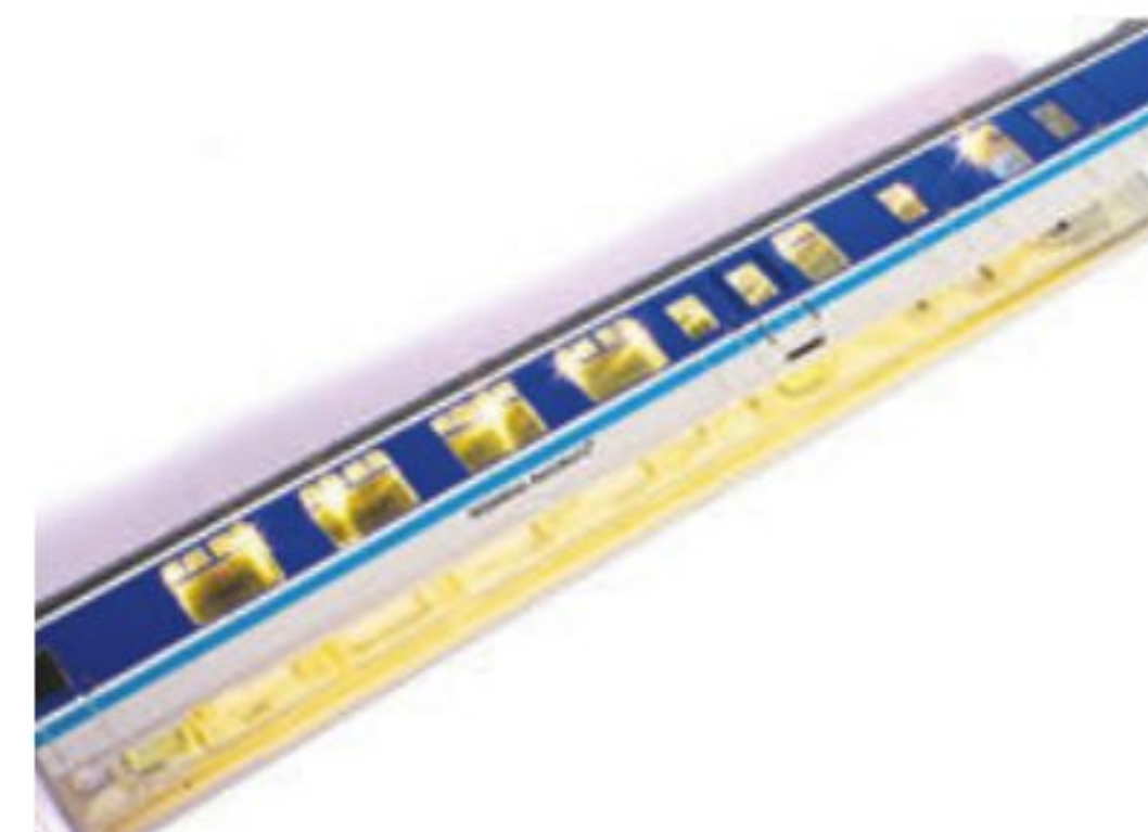
A kit with warm white LEDs was chosen for the Mark 1 coach. It's looking good at this stage, if a little bright. The light level is dimmed by adjusting the potentiometer with a small screwdriver.
