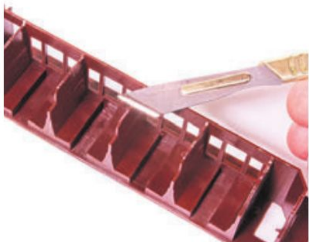
The compartment partitions are trimmed at the top to clear the lighting strip. About 1.5mm of plastic was removed.
