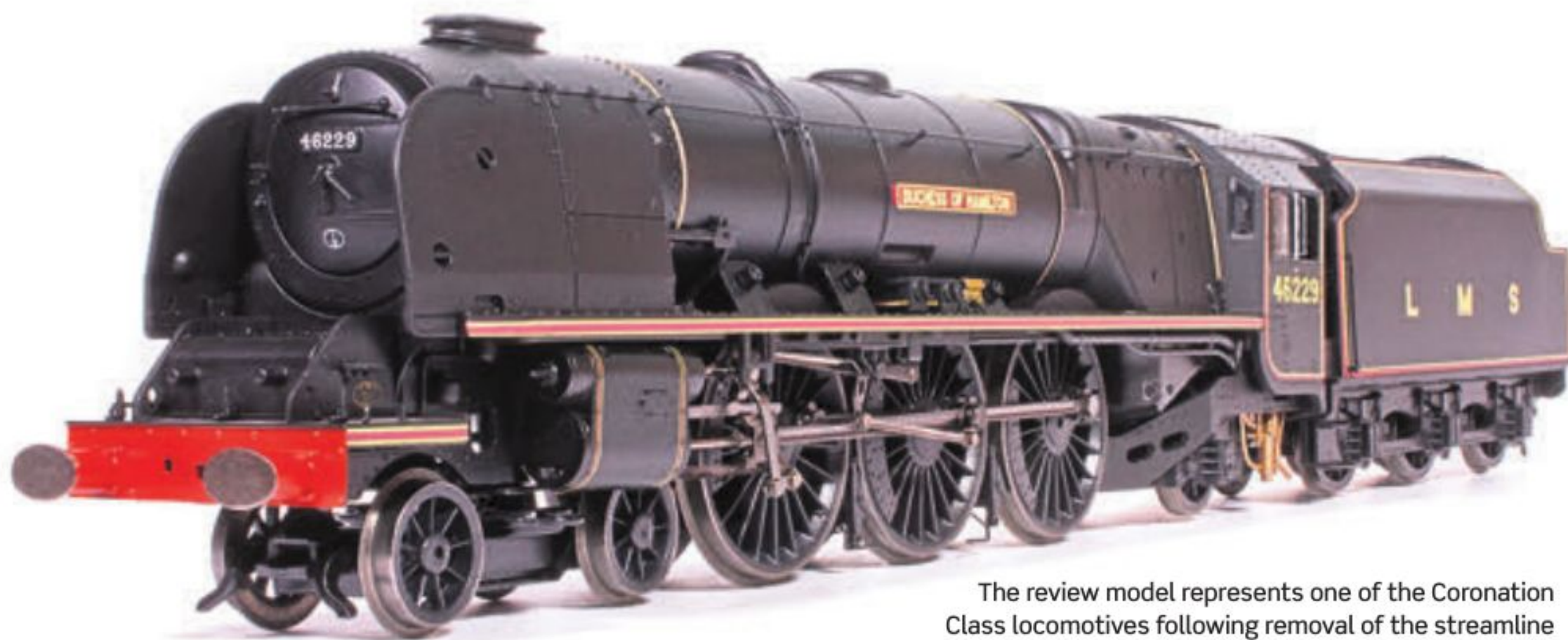
The front bogie is pivoted between the axles and lightly sprung.
