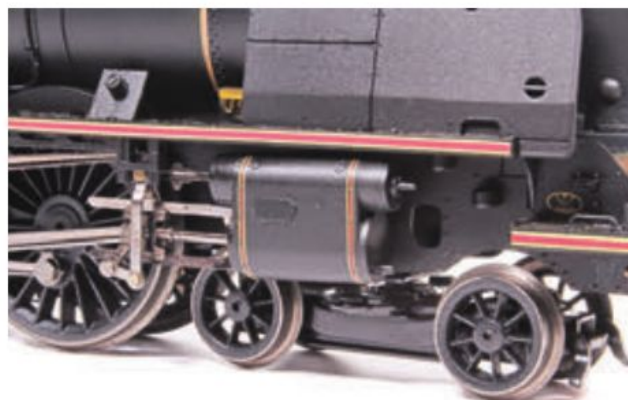
The front bogie is pivoted between the axles and lightly sprung.
