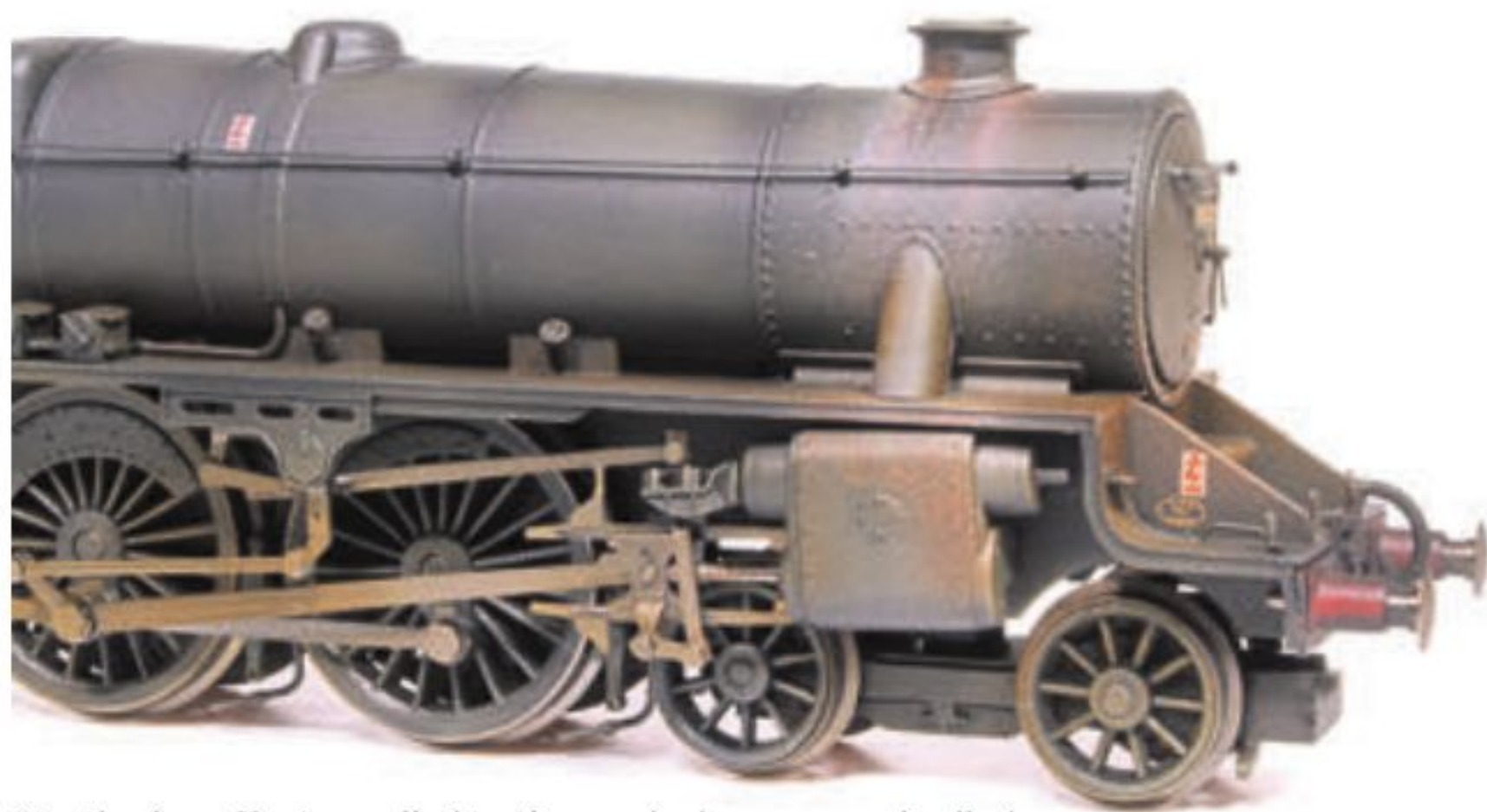
Weathering effects applied to the smoke box area and cylinders. Coupling rods and motion are also nicely rusted.
