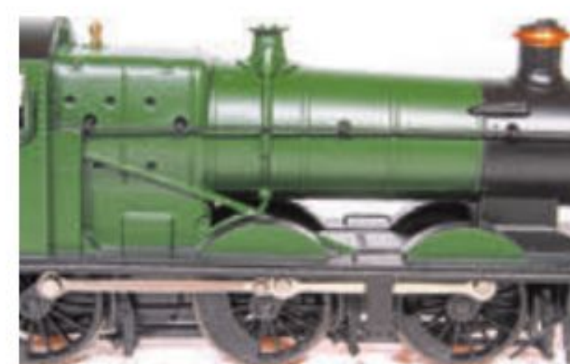
The gap between boiler and frames is clear of mechanism parts and the chassis is well detailed with brake gear and spring detail.
