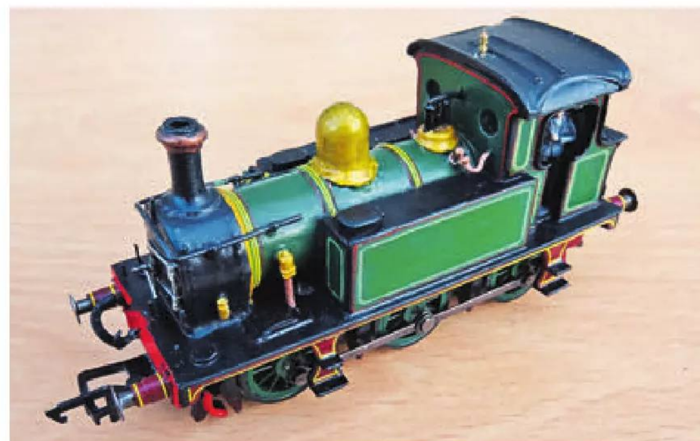
The black and red lining around the outer edges of the model, applied using paint and HMRS red lining from the LNER lining sheet
