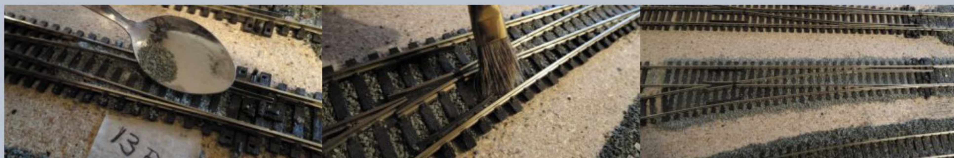
POINTS: Left – Adding small amounts of ballast with a spoon; middle – clearing and spreading the ballast; right – finished point ballast ready to glue.
