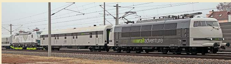
Railadventure bought ex-DB 280km/h test train locomotive No. 103222 last year and has put it into its livery. The loco is seen with the first delivery train to Rostock, with VR 'Vectron' loco No. 193971 on 'buggy' skates near the Siemens Munich Allach factory on March 15. SIEMENS
