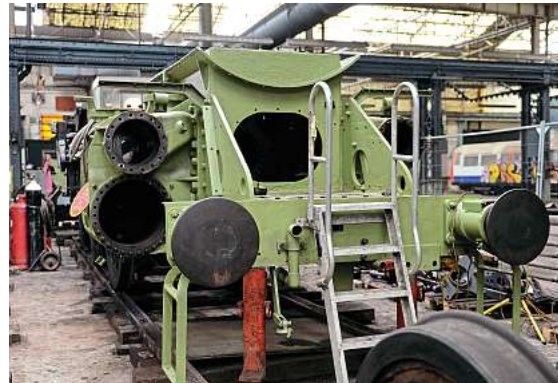
Dismantled No. 35005 Canadian Pacific stands inside the former Southern Railway erecting shop at Eastleigh on March 15. The rebuilt 'Merchant Navy' will be running again in two and a half years. RON COVER
