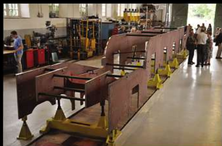
Frames erected and all major castings manufactured, including all 20 wheels.
