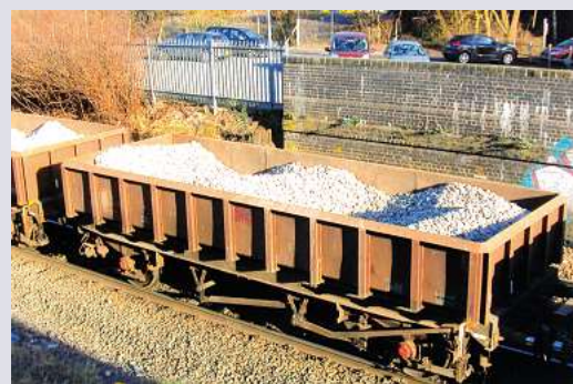
Older four-wheel MHA 'Coalfish' wagons, such as No. 394544, in this picture, are being replaced by newer MXA bogie wagons. S F LAPPAGE
