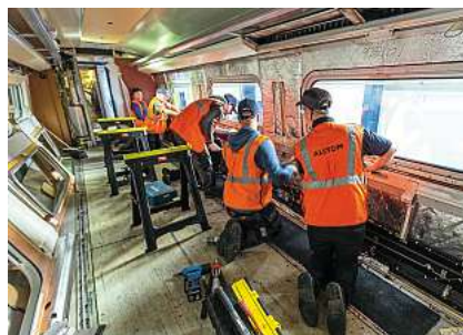
Left: Technicians at Alstom's Oxley depot strip the interior of 'Pendolino' coach G before rebuilding it as a standard class carriage. VIRGIN TRAINS
