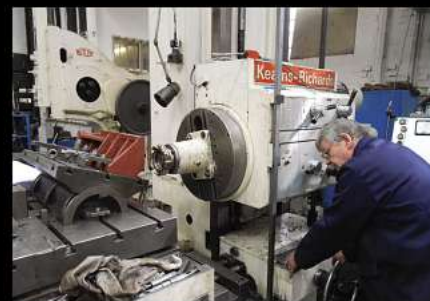
The Cartazzi horn block being machined.
