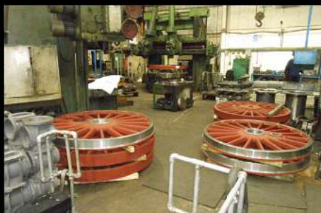
All 20 wheels now cast and being machined. Progress to date is astounding!
