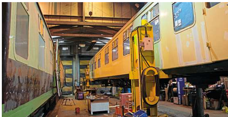
Left: The two-road lifting shop shed houses a useful 45-ton crane and will eventually be used for boiler lifts. At the moment, the building is used for carriage maintenance. The Mk 1 on the right is No. 1348, described in the main text.
