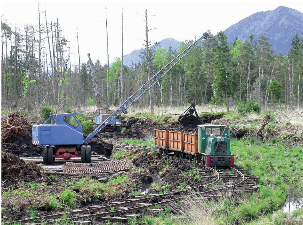
Deep in the forest, something stirred... 1950s-vintage cranes excavate the peat as Schöma diesel No. 4230 waits to take the loaded wagons to the unloading point. Both pictures taken on May 8, 2014, by J HARDING.
