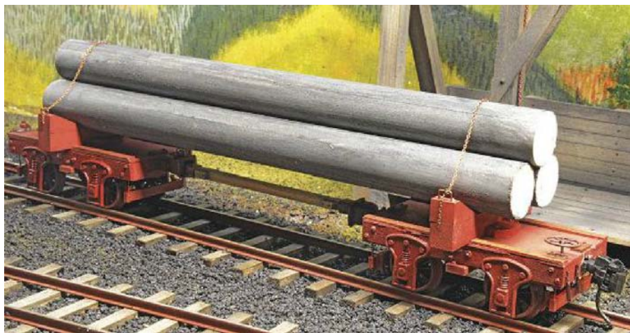
Above: A finished pair shows the rooster and logs in place.
