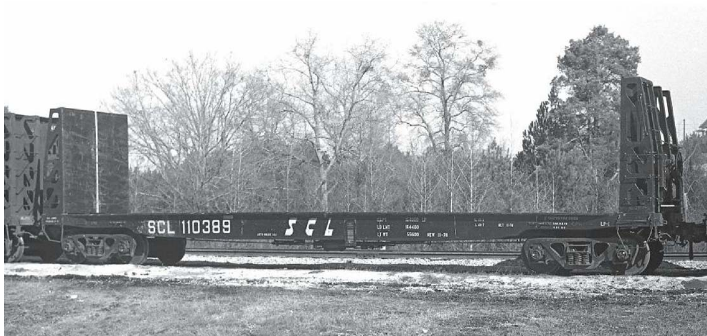
Above: In this image of SCL 110389, taken at Woodland, Georgia, on February 13, 1971, we can see the subtle changes in the side sill architecture mentioned in the text. The bulkhead design change is much more obvious. — Larry Goolsby photo
