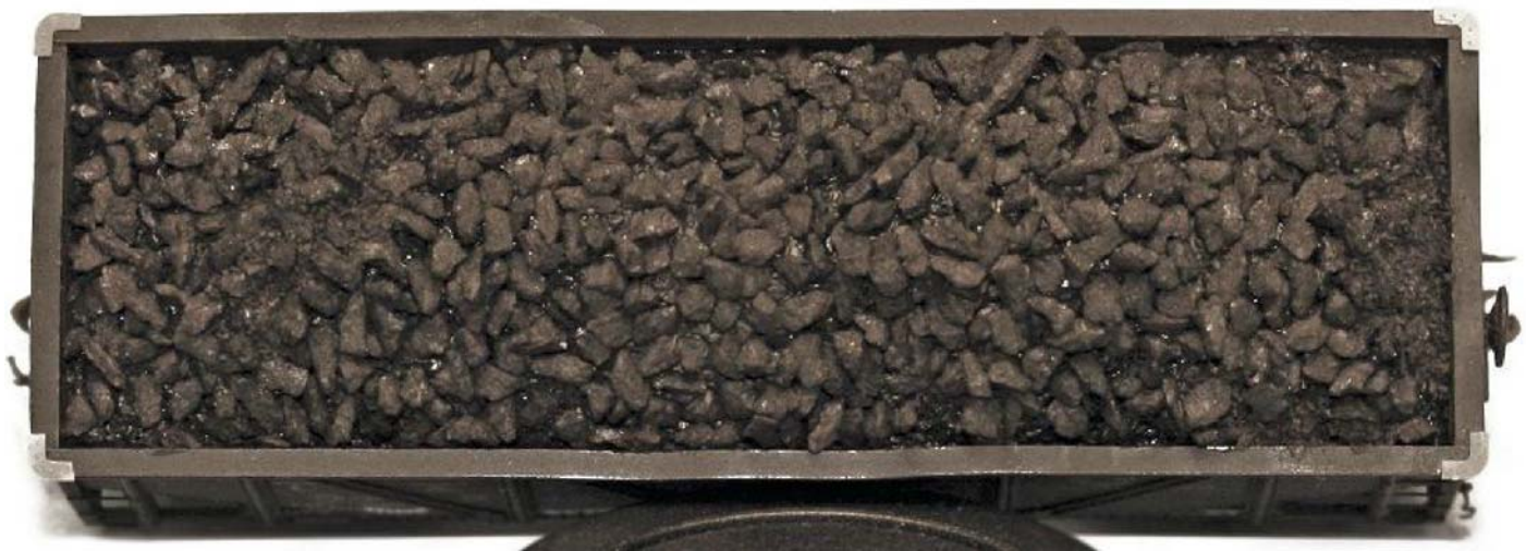
Tichy corner gussets were added to the top chord of the car. The large lump coal was added to represent a load of coke.
