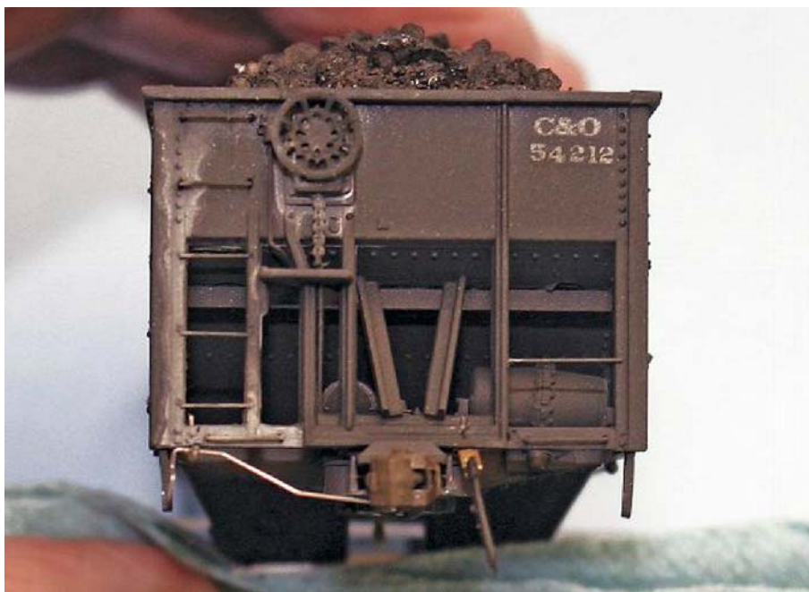
The B end shows off lots of detail, including the Precision Scale Ajax brake wheel and air hose bracket, Hi-Tech rubber air hoses, 0.012 phosphor-bronze wire grab irons, Tangent Models coupler cut levers, Evergreen 0.080 angle stock made into slope sheet supports, state-of-the-art schedule AB brake components, wire retainer line, and real chain and rod hand brake linkage.
