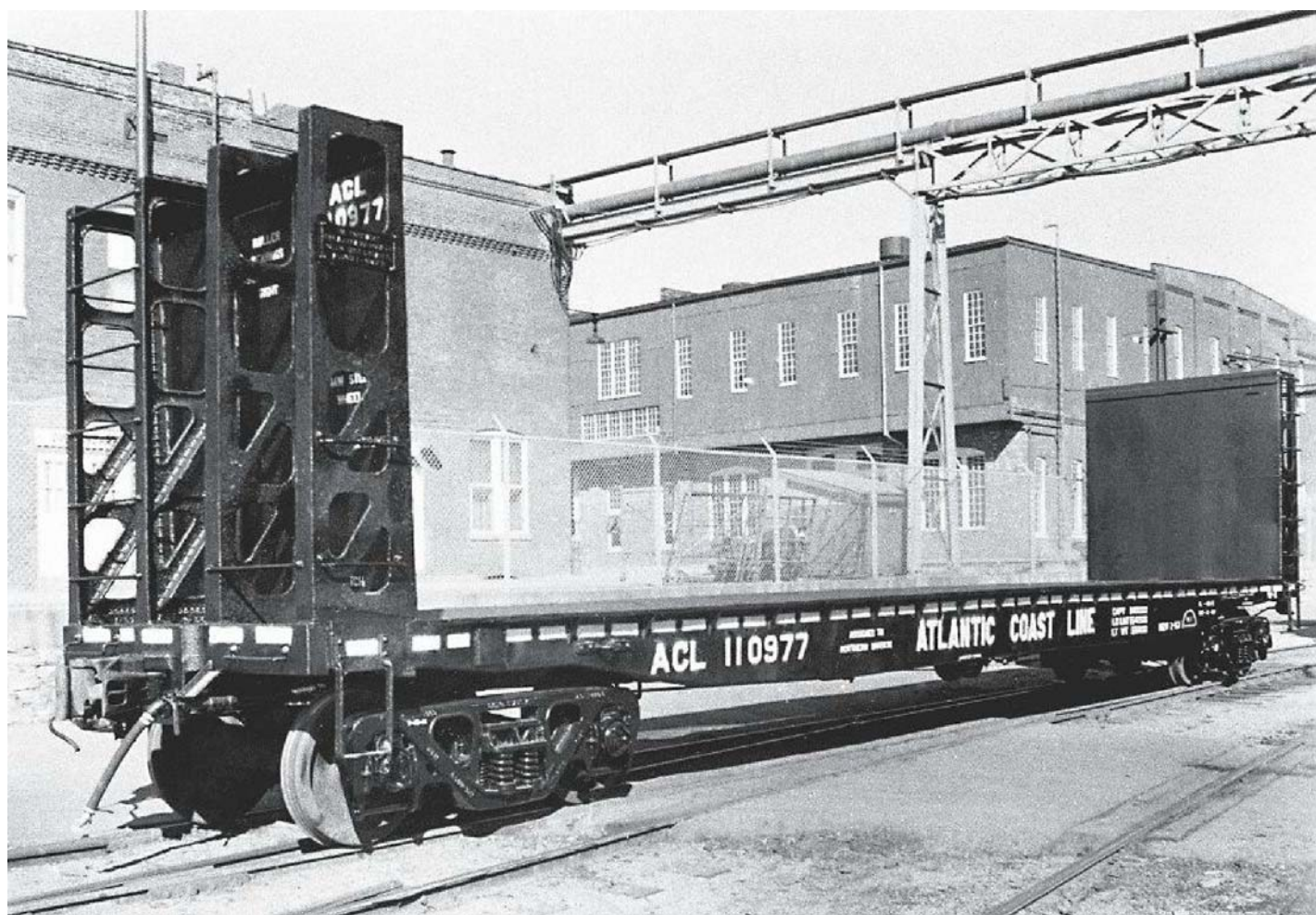
Below: In a rather unusual move, the ACL had American Car & Foundry assemble one lot of pulpwood cars at the St. Louis plant in 1953. This may have been due to the road's Waycross shops being too busy to build the cars. — ACF photo, Ed Hawkins collection
