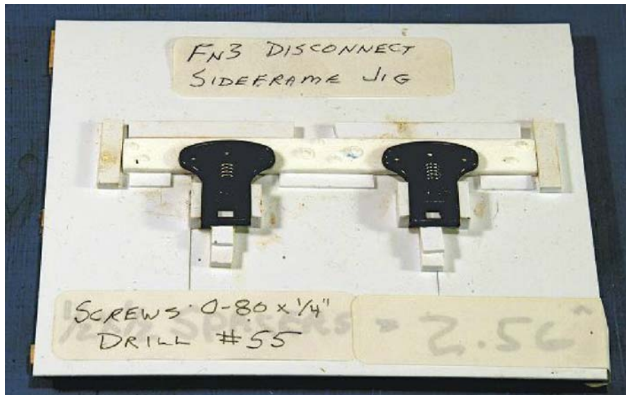
Above: A jig was used to make sure all the pedestals were in the exact same place and the wheels were at a true 90 degrees to the sideframe and exactly across from one another.
