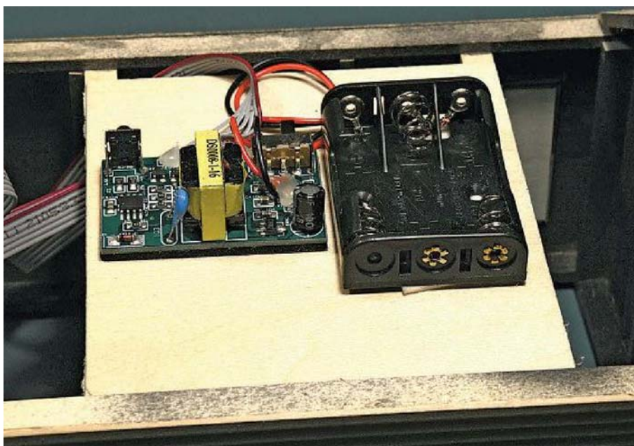
The electronics were mounted to two sticks of styrene to rest just under, and clear of, the roof.
