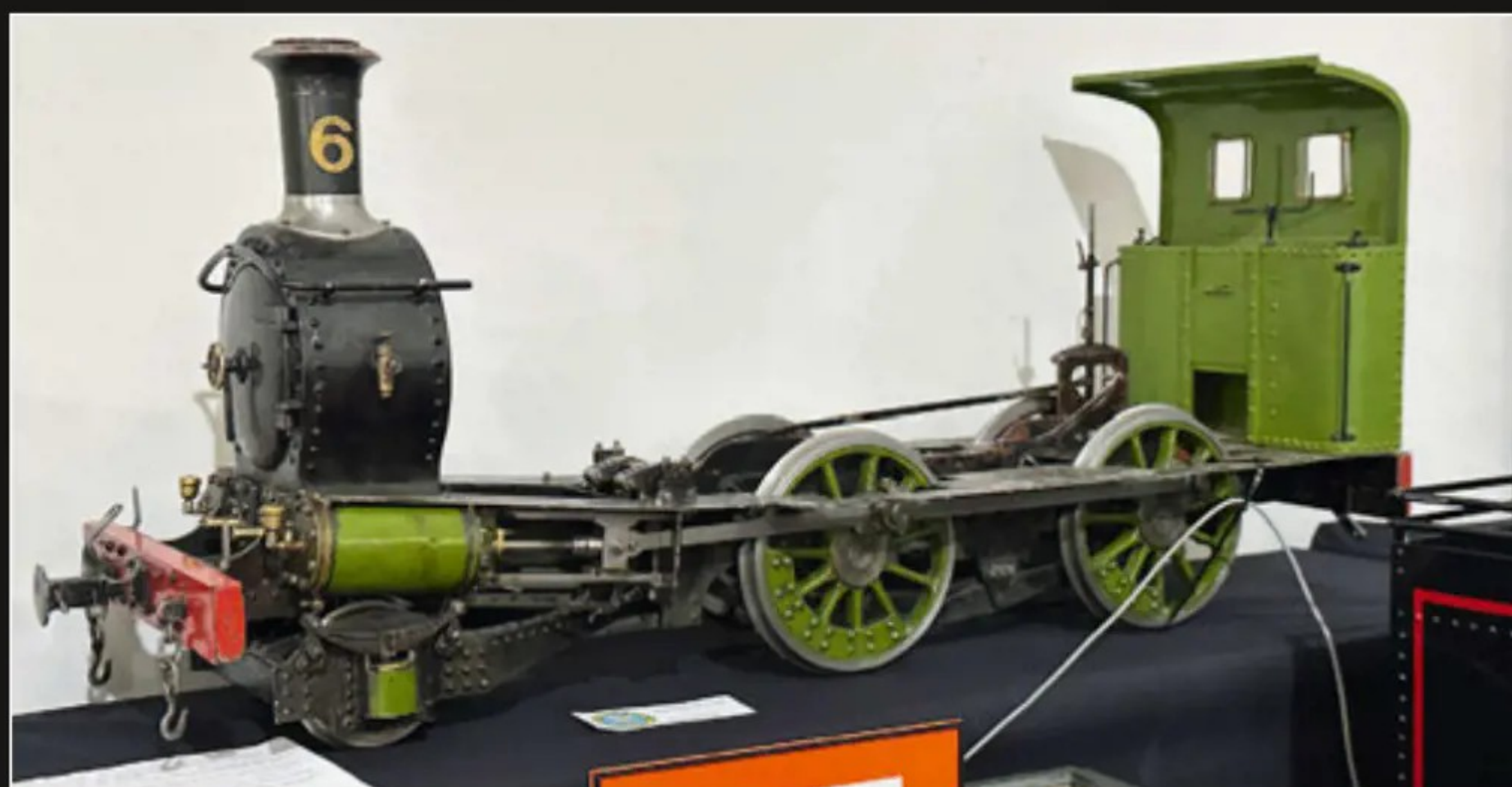
Below: 3ft gauge prototypes, such as this under construction Isle of Man Railway 'Peverill', make for more compact models.
