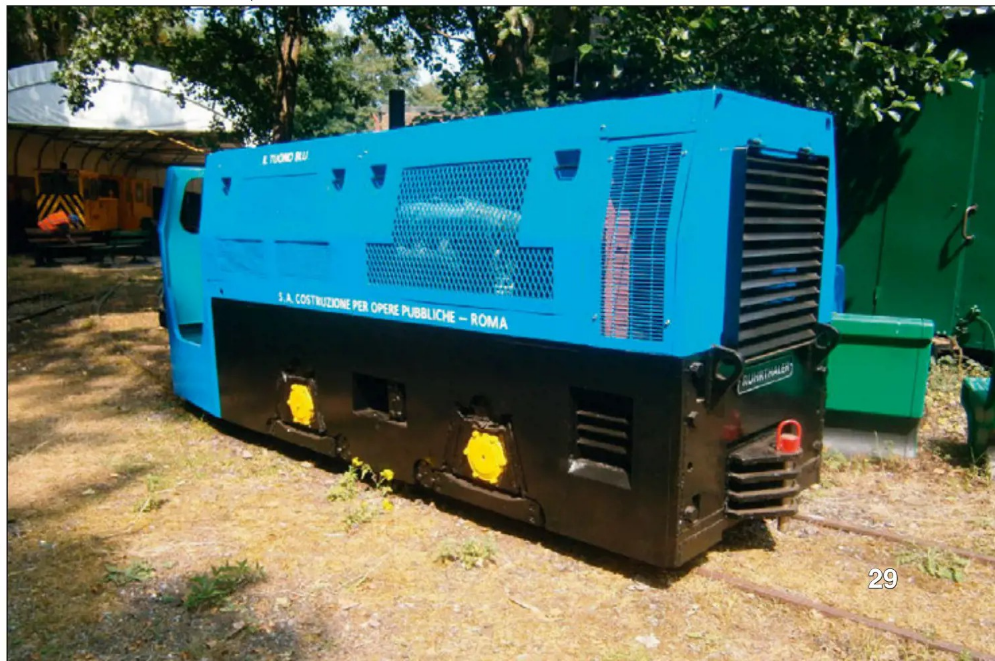
Below: 140HP Ruhrthaler 0-4-ODH 'Il Tuono Blu' (3920/1969), ex-Rome Public Works Company, restored to working order in June 2024 after 15 years in open storage.
